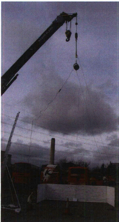
Photograph 19 – Test 11 10.2 m drop test over top rim
