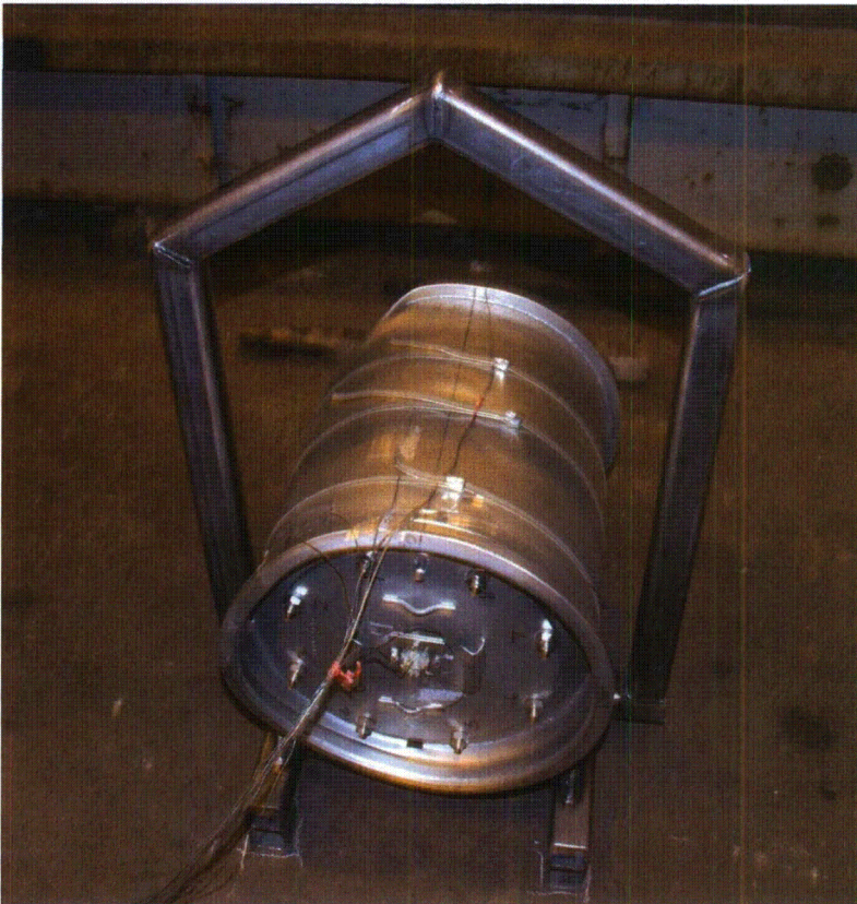
Photograph 23 – Test package on support cradle in preparation for thermal test
