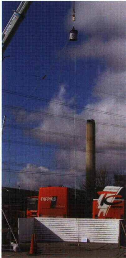
Photograph 20 – Test 12 10.2 m drop test over top end.
