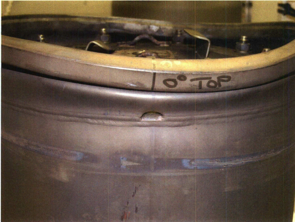
Photograph 54 – Damage caused to top rim
