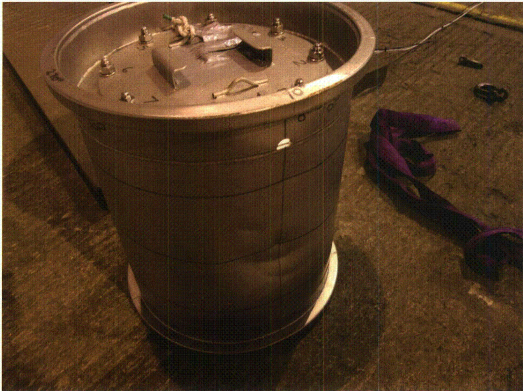
Photograph 36 – Test 9 damage caused to package
