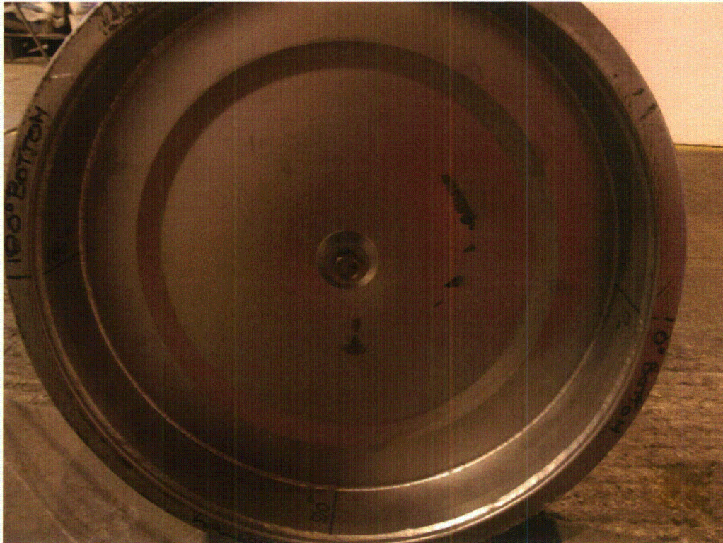
Photograph 34 – Test 8 damage caused to keg
