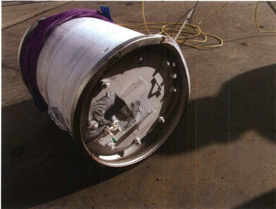
Photograph 46 – Test 12 damage caused to keg
