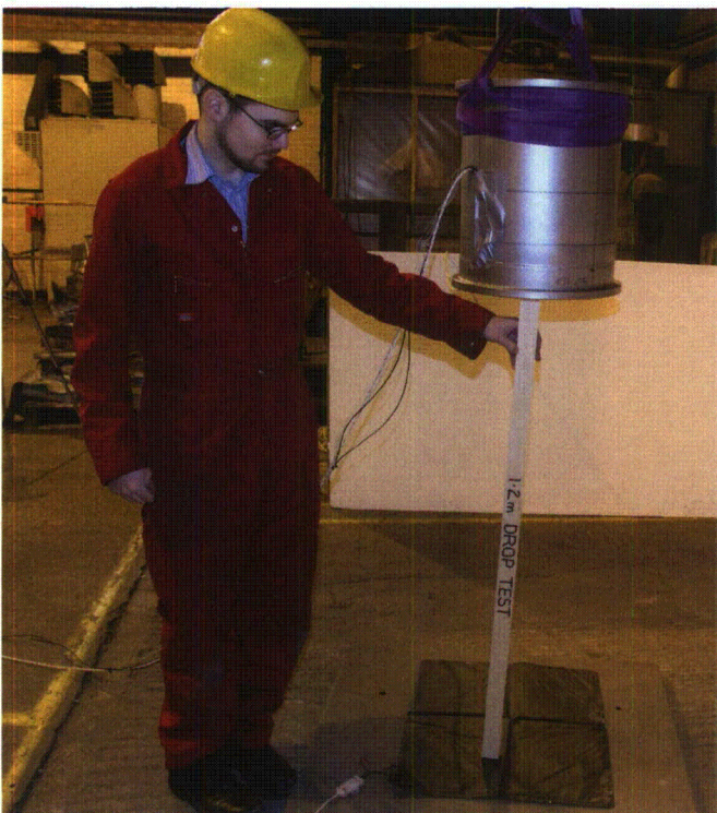
Photograph 13 – Test 5 1.2 m drop test onto top end
