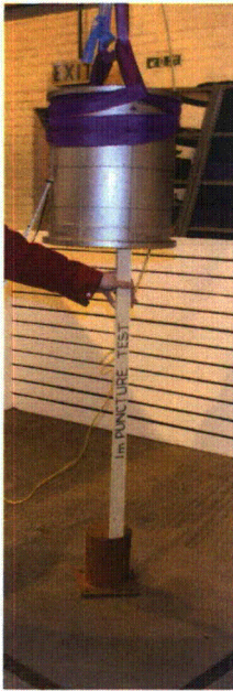
Photograph 16 – Test 8 1m puncture test over bottom
