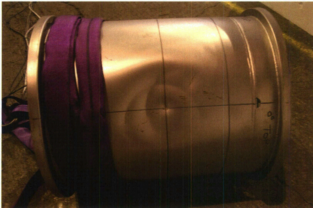
Photograph 32 – Test 7 damage caused to keg
