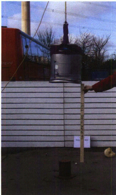
Photograph 21 – Test 12a 1m puncture test on top end
