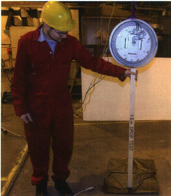
Photograph 12 – Test 4 1.2 m drop test onto side
