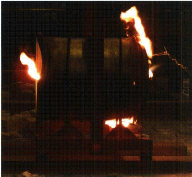
Photograph 50 – Test 13 Removal of Package from Furnace
