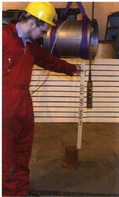
Photograph 15 – Test 7 1m puncture test over side
