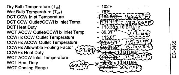
\*As discussed in section 5.4, these values are calculated using an ACCW inlet temperature to the CCWHx of 89.3°F in order to maintain the Tech. Spec. maximum ACCW temperature of 89°F.
