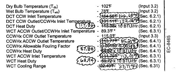
\*As discussed in section 5.4, these values are calculated using an ACCW inlet temperature to the CCWHx of 89.3°F in order to maintain the Tech. Spec. maximum ACCW temperature of 89.0°F.
