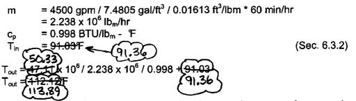
Using STER Version 5.04, the following heat exchanger performance is calculated for a CCW<sub>out</sub> temperature of 115F. The printouts are provided in Attachment 7.2
