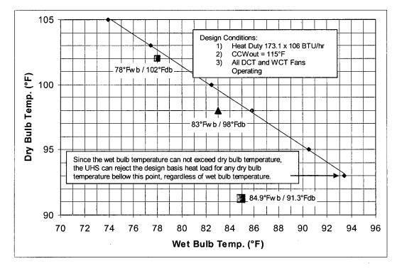
Note: The  $102^{\circ}F_{db}$  /  $78^{\circ}F_{wb}$  point does not fall on the curve as may be expected. This is due to the methodology discussed in section 5.4 and implemented in 6.4.1. The WCT basin temperature would be maintained cooler than the temperature specified in Technical Specification 3/4.7.4, assuming the design basis meteorological condition of  $102^{\circ}F_{db}$  /  $78^{\circ}F_{wb}$ .
