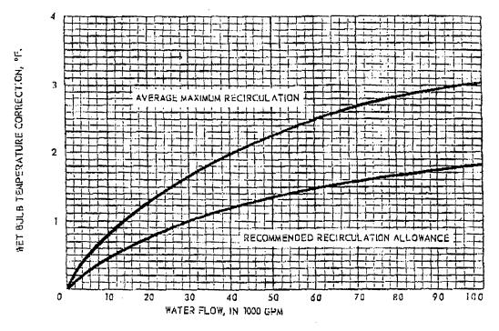
NOTE: Recipitation allowances shown in Curve shows are based on a 20 F approach to any war bulb tomperature. Recipitation allowandes for other performance conditions can be obtained by means of the Correction Factors shown at right. For further instructions are reverse of this sheet.
