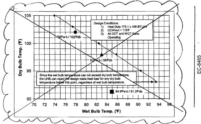
Note: The  $102 \text{F}_{db}$  /  $78 \text{F}_{wb}$  point does not fall on the curve as may be expected. This is due to the methodology discussed in section 5.4 and implemented in 6.4.1. The WCT basin temperature would be maintained cooler than the temperature specified in Technical Specification 3/4.7.4, assuming the design basis meteorological condition of  $102 \text{F}_{db}$  /  $78 \text{F}_{wb}$ .
