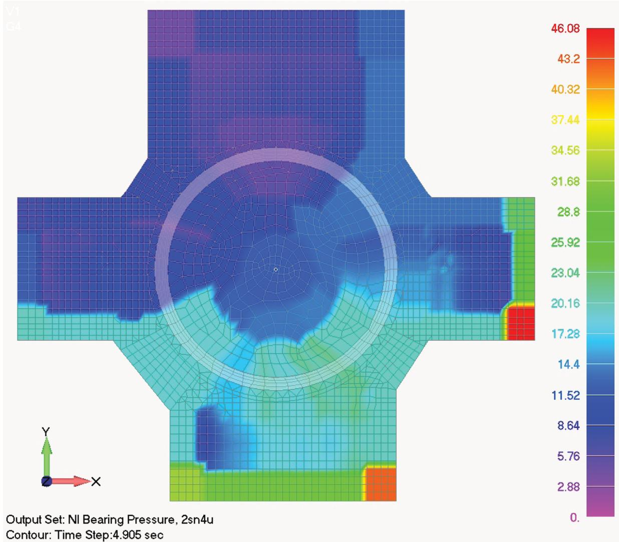
**Figure 3.8.5-28-C: Bearing Pressure, Analysis Case 4ue-cr, Seismic and Dead Load, Time = 5.160 sec, Plan View, (ksf)**
