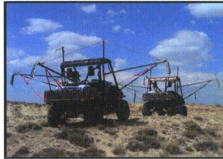
Figure 2.9-4: 3-detector GPS-based scanning systems mounted on Rhino OHVs
