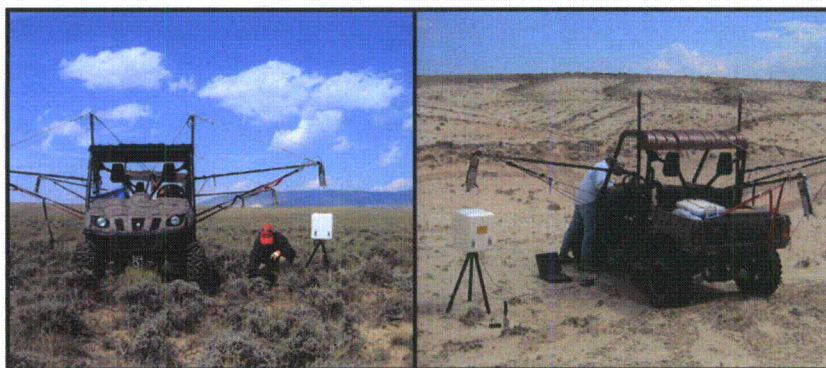
Figure 2.9-5: Photos of NaI/HPIC cross-calibration measurements being performed at other ISR sites in Wyoming
