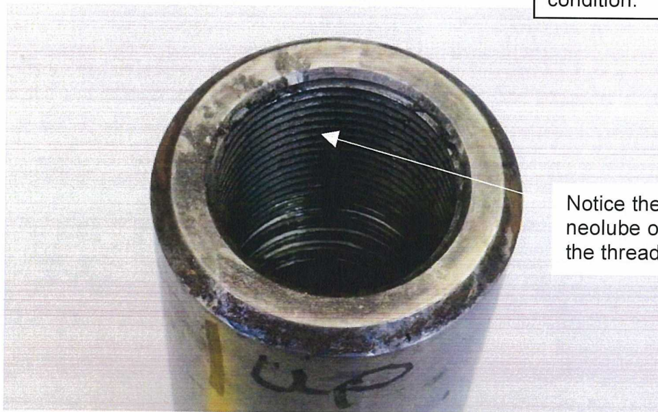
Figure 2-1: As-Received Coupling No. 11-P7A-7
