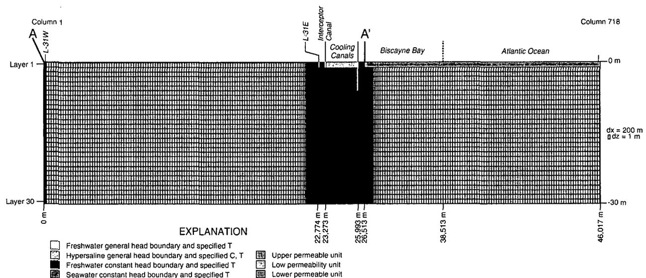
**Fig. 2** Model grid, boundary conditions, and hydraulic conductivity zones evaluated. The location *A* to *A'* in the two-dimensional cross-section model is shown in Table 1. Model parameters used in the two-dimensional cross-section model and the hydraulic conductivity values associated with each hydraulic unit is summarized in Table 2
