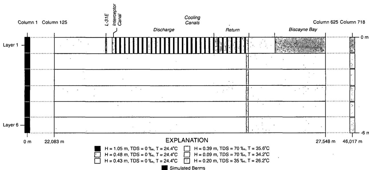
**Fig. 3** Configuration of boundary condition heads, TDS concentrations, and temperatures in the vicinity of the cooling canal system in the two-dimensional cross-sectional model
