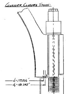
P. DESIGN PRESSURE: 2.5 KS/ DESIGN TEMP: 650 F ds - STUD SIZE: 6.797" SHANK DIA. dy = HOLE THEN CENTER OF STUD: 1.125" N= NUMBER OF STUDS: 54 STUD MATERIAL: SA-320 GR. L43 CLASS 3 WITH Sm = 34.8KSI AT 650 F.
