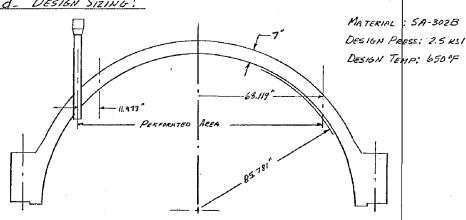
CONSIDER THE REQUIRED THICKNESS IN THE UN-PERFORATED AREA! REFERENCE PARAGRAPH N-431, SECTION III NUCLEAR CODE:
