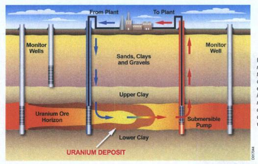
In-situ leach (ISL) mining involves recovering minerals such as uranium through boreholes drilled into the deposit. CNWRA developed a generic environmental impact statement to identify and evaluate potential environmental consequences of constructing, operating and restoring aquifers, and decommissioning ISL facilities in the western United States.
