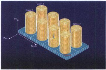
Geometrical stability of storage dry casks under earthquake conditions was evaluated using a finite element model of freestanding cylindrical casks on a concrete pad embedded in deep soil deposits and time domain soil-structure interaction analyses.
