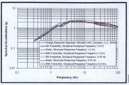
CNWRA engineers evaluate the seismic design bases of structures identified as important to safety by comparing structural response curves.
