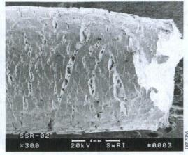
CNWRA researchers evaluated the stress corrosion cracking susceptibility of waste package materials in potential repository environments. Test results show the possibility of Alloy 22 stress corrosion cracking within a narrow range of environmental conditions and electrochemical potentials.
