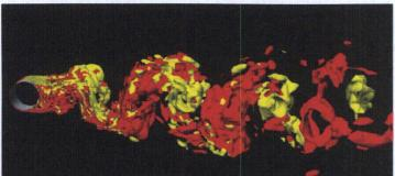
CNWRA performed three-dimensional simulations of high-speed cooling-water flow around fuel assemblies in nuclear power plants.
