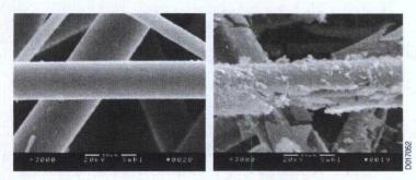
CNWRA scientists evaluated how the chemical degradation of submerged insulation materials may affect emergency cooling pumps in nuclear reactors after a loss-of-coolant accident.
