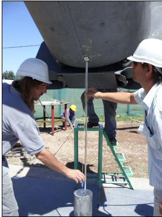
Figure 6: 1.030m above target (with height gauge)
