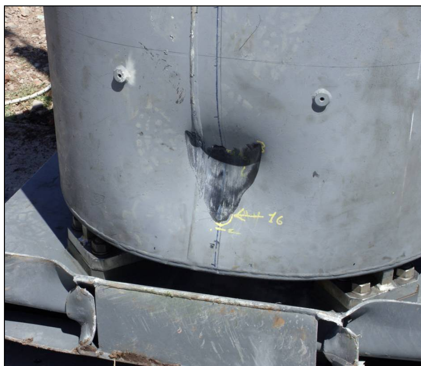
Figure 9: Impact point and jacket indentation
