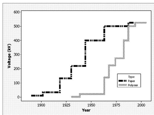
Figure 1 Evolution of the Highest AC Cable Voltage
