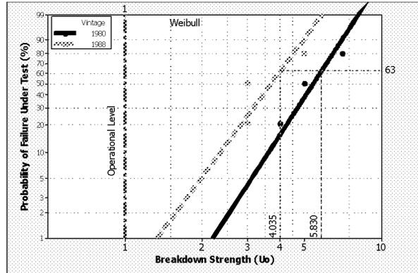
**Figure 5** AC Step ( $U_0/5min$ ) Breakdown Tests On XLPE Unjacketed Cables Identified As Poor Performers. Vertical Dashed Lines Show The Weibull Scale Parameter.
