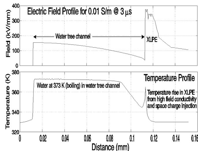
Figure 3. Electric field and temperature profiles on axis for water conductivity of 0.01 S/m at 3 μs into the lightning impulse waveform. The profiles run from just inside the conducting water tree region (left), through the axis of the water tree channel, and into the XLPE beyond the tip of the water tree channel. The temperature rise (from an initial 330 K) is greatest at the base of the water tree channel for reasons discussed in the text. The water is assumed to boil.
