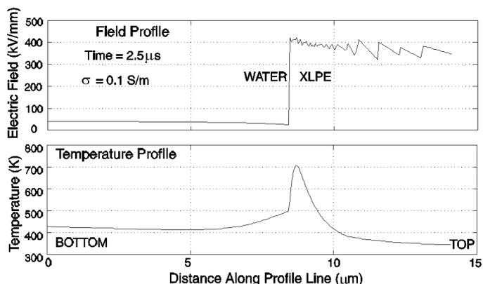
Figure 11. Electric field and temperature profiles for water conductivity of 0.1 S/m at 2.5  $\mu$ s into the lightning impulse waveform for a computational model which assumes that the water is confined at constant volume so that it cannot boil and which also includes high field conductivity in the XLPE. As seen from Figure 12, the maximum temperature in the channel of about 480 K would result in a pressure throughout the channel of about 1.6 MPa or 16 bars.
