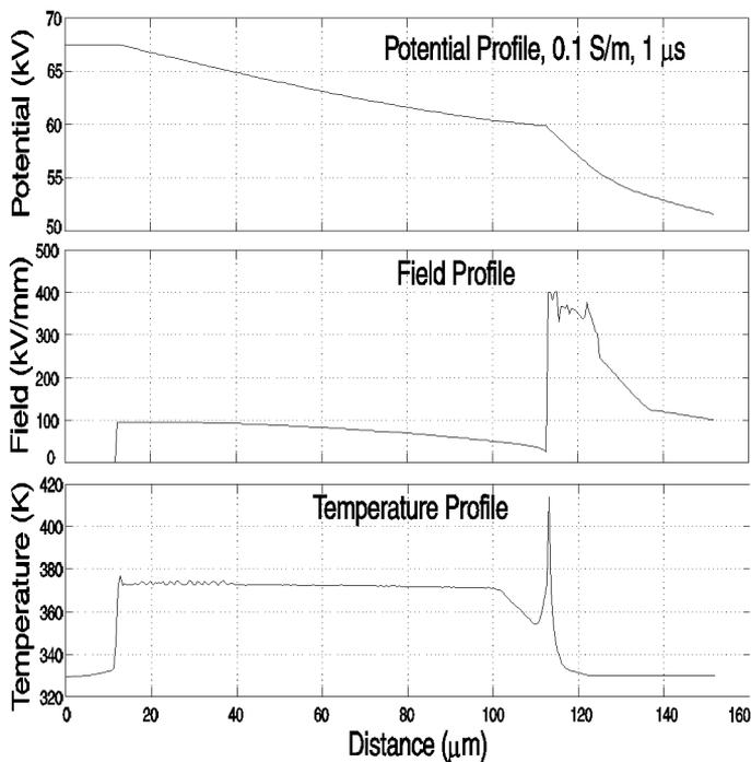
Figure 7. Electric potential, electric field, and temperature profiles for water conductivity of 0.1 S/m at 1  $\mu$ s into the lightning impulse waveform for a computational model which includes high field conductivity in the XLPE. Even before the peak voltage of the impulse, the water is boiling over most of the tree channel length, and the high field conductivity-induced temperature rise in the XLPE at the tip of the water tree channel is over 140 °C.
