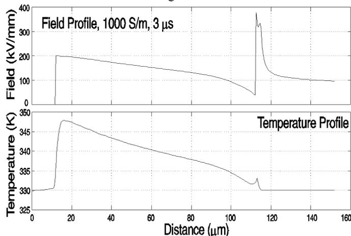
Figure 10. Electric field and temperature profiles on axis of a 1  $\mu$ m diameter water tree channel for a water conductivity of 1000 S/m at 3  $\mu$ s into a standard lightning impulse of 80 kV magnitude. The conductivity is sufficiently high that the water does not boil during the lightning impulse.
