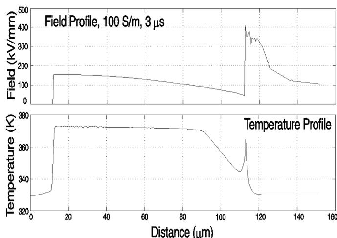
Figure 9. Electric field and temperature profiles on axis of a 1  $\mu$ m diameter water tree channel for a water conductivity of 100 S/m at 3  $\mu$ s into a standard lightning impulse of 80 kV magnitude. The water boils over most of the length of the water tree channel.
