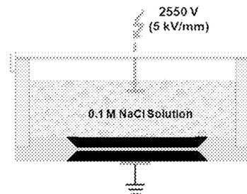
Fig. 1. Experimental setup for electrical aging test. The sandwiched semicon-PE-semicon sample is employed for simulation of stress exposure in cable. Standard conductor semicon and 0.1 M NaCl are used in aging as sources of ions.
