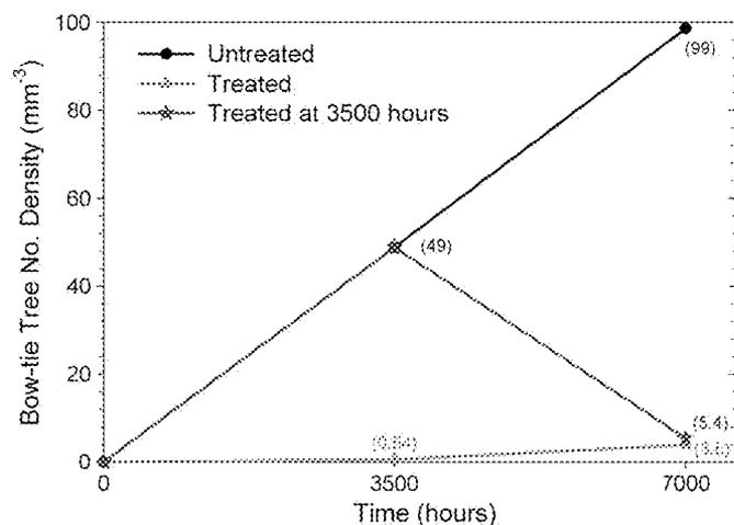
Fig. 5. Plot of bow-tie water tree number density as a function of aging time for the various sample classes. The numbers in parentheses provide the numerical value of the datum. Bow-tie water tree number density is presented as volume number density (mm<sup>-3</sup>).
