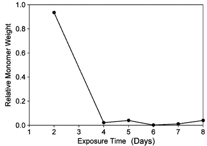
Fig. 2. Phenyl Methyl Dimethoxy Silane (PMDMS) content in the semicon-PE-semicon plaque as a function of exposure time in 100% relative humidity at 50 °C. Four days exposure of the fluid-saturated samples is sufficient for nearly complete curing.
