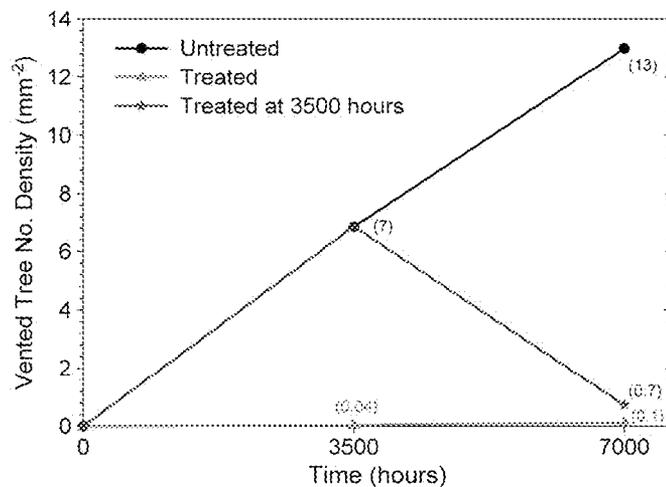
Fig. 6. Plot of vented water tree number density as a function of aging time for the various sample classes. The numbers in parentheses provide the numerical value of the datum. Vented water tree number density is presented as number of vented water tree per unit semicon-insulation interface area (mm<sup>-2</sup>).
