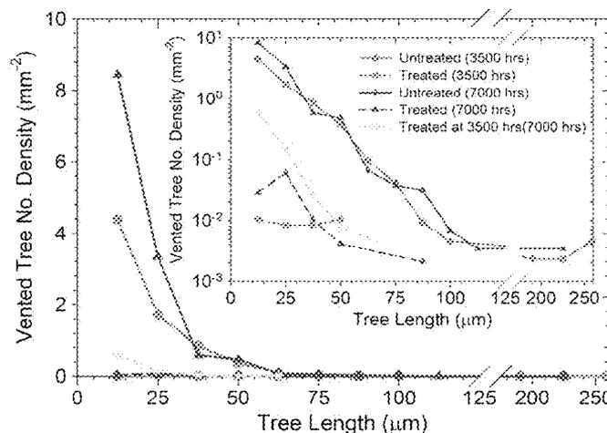
Fig. 7. Vented water tree length distribution for all five sets of sample plaques after 3500 and 7000 h aging at 5 kV/mm and exposure to 0.1 M NaCl solution. The main plot has a linear ordinate while the subplot presents the same data on a logarithmic ordinate. Treated samples, whether treated prior to aging or at the midpoint of aging, contain very few vented water trees.
