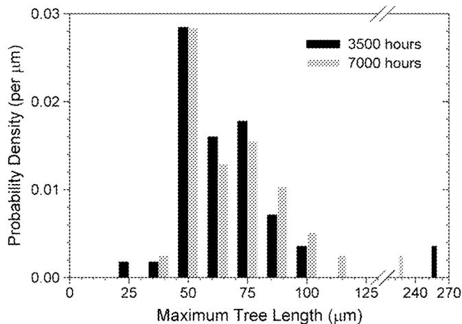
Fig. 4. Probability density for maximum vented water tree length in untreated sample plaques. The typical maximum vented water tree length per slice under examination is 50 to 75 μm at both 3500 h and 7000 h aging time.
