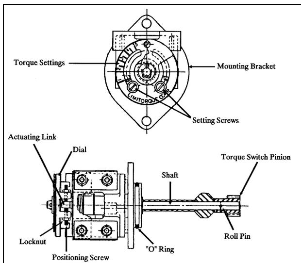
**Figure 5-10 Knee Type Torque Switch (New Style)**
