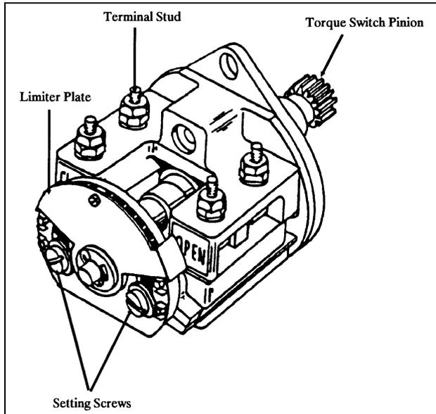
**Figure 5-9 Knee Type Torque Switch (Old Style)**
