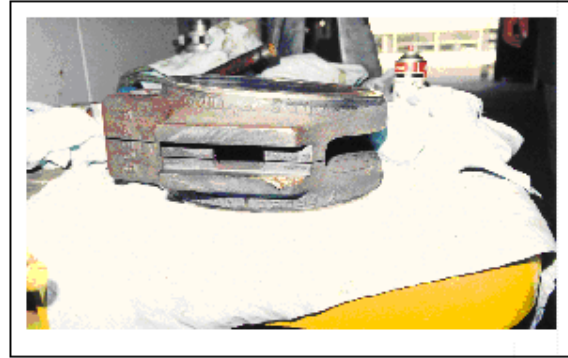
Figure 3-10 Valve Damage to Disc Guides
