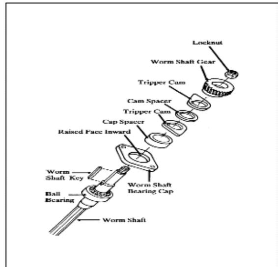
**Figure 2-23 SMB-000/00 Worm Shaft Gear Assembly**
