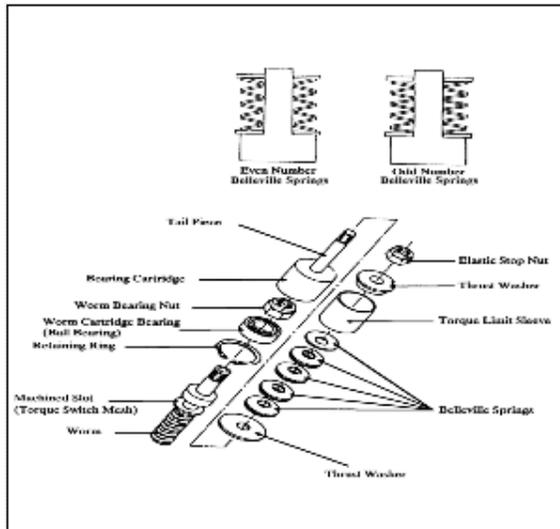
**Figure 2-24 SMB-000/00 Worm/Belleville Spring Pack Assembly**
