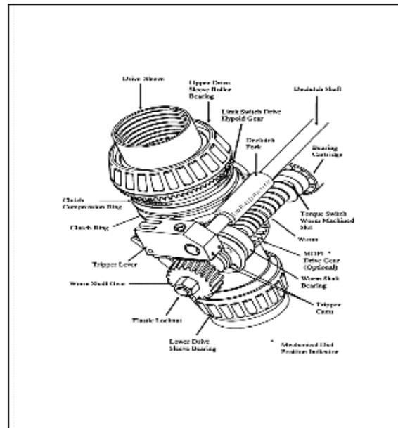
Figure 2-19 SMB-00 Actuator Drive Sleeve
