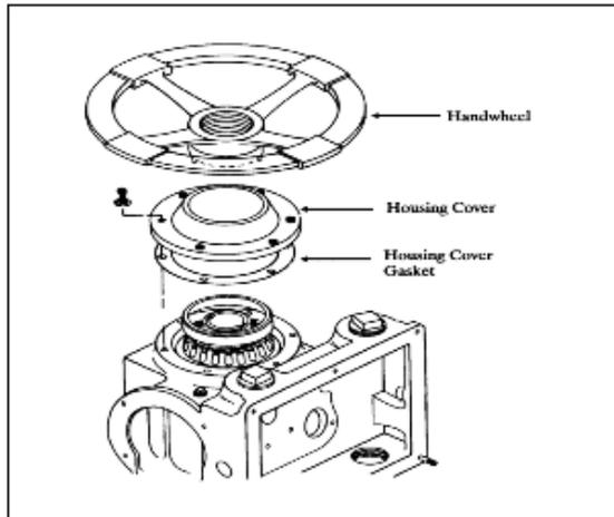
**Figure 2-14 SMB-00 Top-Mounted Manual Power Train**
