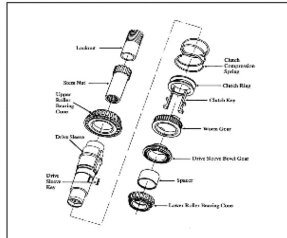
**Figure 2-27 SMB-000/00 Drive Sleeve Exploded View**
