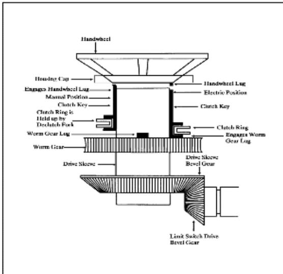
**Figure 2-15 SMB-000/00 Handwheel Worm Gear Assembly**
