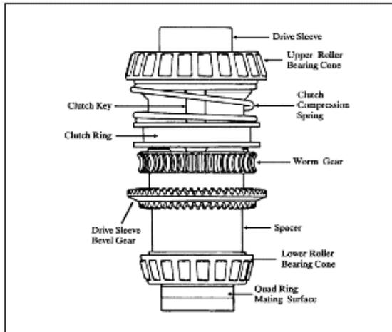
**Figure 2-26 SMB-000/00 Drive Sleeve**
