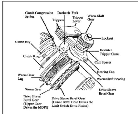
Figure 2-17 SMB-000 Actuator Drive Sleeve Assembly
