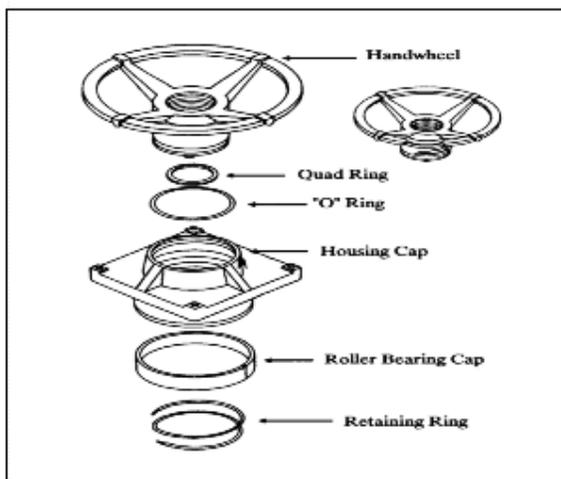
**Figure 2-28 SMB-000/00 Handwheel and Housing Cap Assembly**
