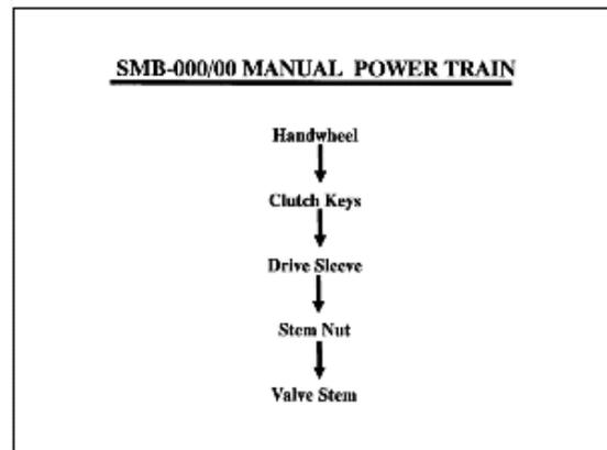
From this point the power train in manual matches the power train in electric and the effect on the valve is the same. The only thing that protects the valve in this case, however, is a well-trained operator.
