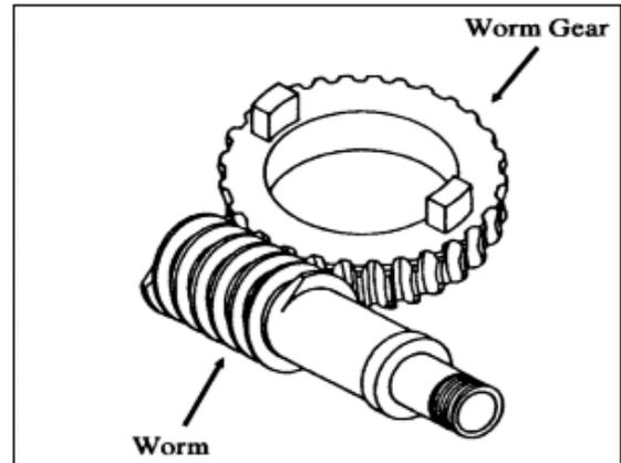
Figure 2-25 SMB-000/00 Worm and Worm Gear
