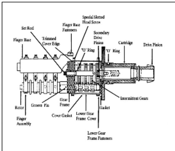
Figure 2-18 SMB-000/00 Limit Switch Assembly
