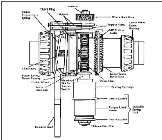
Figure 2-12 Electric Power Train Side View
