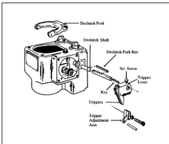
Figure 2-29 SMB-000/00 Declutch Mechanism
