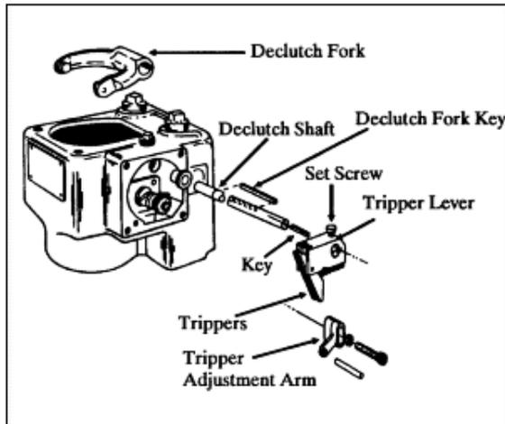
Figure 2-16 SMB-000/00 Declutch Mechanism
