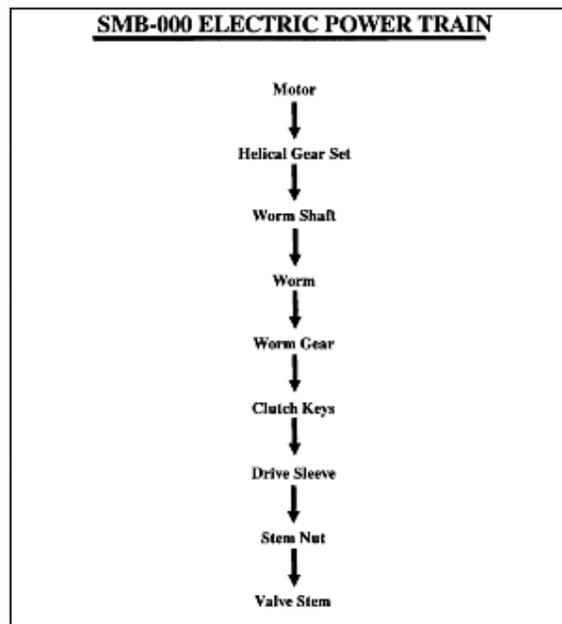
As the clutch keys are driven, they drive the DRIVE SLEEVE which has internal splines. Those internal splines rotate the STEM NUT which can be threaded, splined, or keyed. The stem nut rotates around the valve stem or input shaft and the valve will be repositioned by the motion of the valve stem. In normal operation, this will
