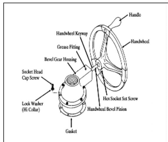
Figure 2-13 SMB-00 Side-Mounted Manual Power Train
