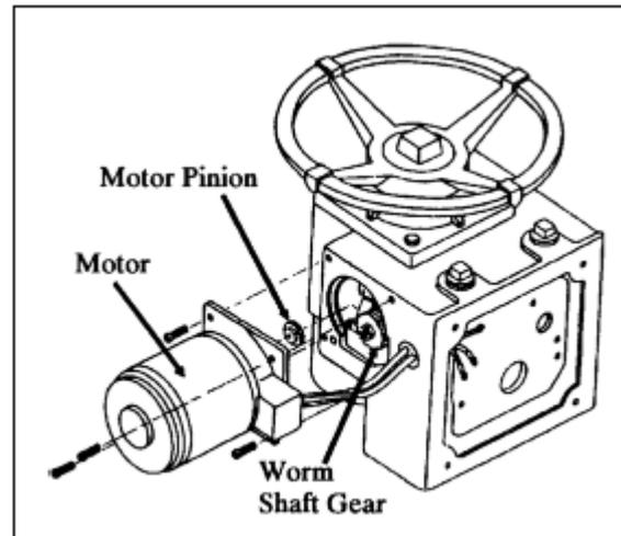
**Figure 2-22 SMB-000 Motor**
