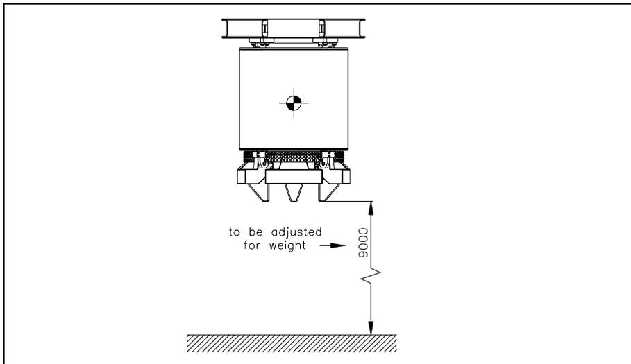
5.13.6 Drop 10 (1.0m punch: Onto top shield opposite vent plug)
