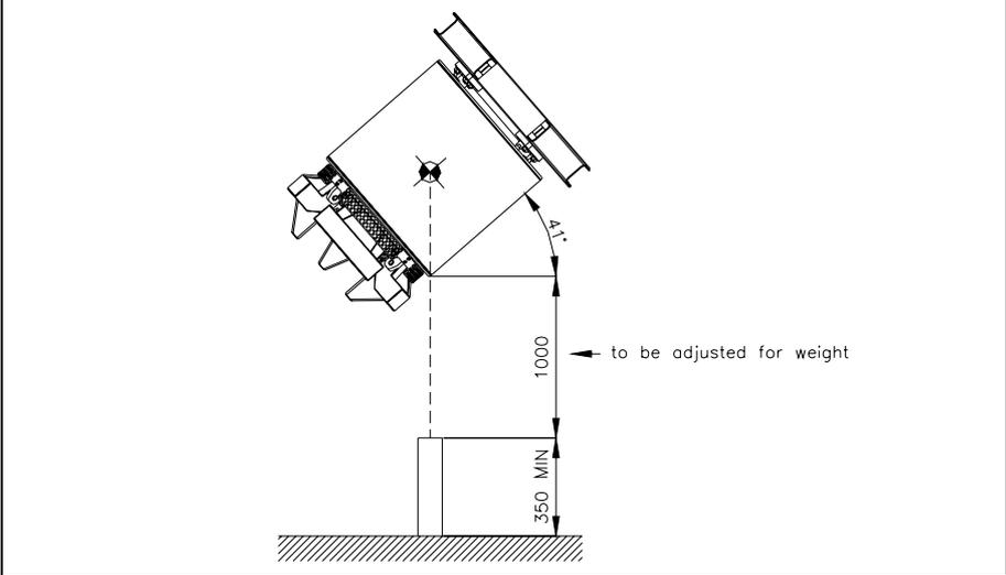
5.13.10 Drop 14 (1.0m punch: Onto jacket opposite drain plug)
