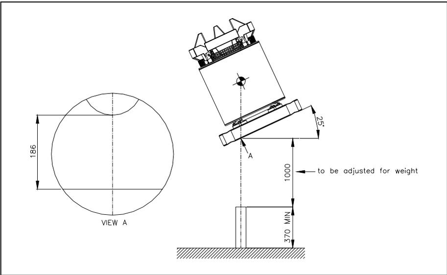
5.13.4 Drop 8 (1.0m punch: Onto top shield over vent plug)
