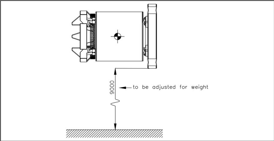
5.13.12 Drop 16 (1.0m punch: Onto jacket over drain plug)
