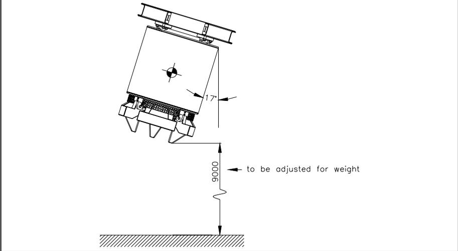
5.13.9 Drop 13 (1.0m punch: Angled inverted onto jacket corner)
