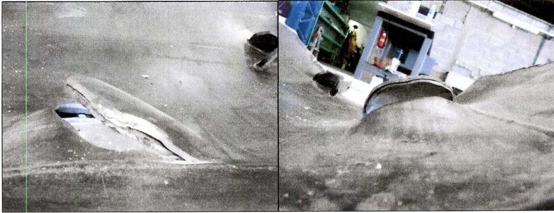
Figure 25: Shearing of jacket outer and inner skins from angled side punch
