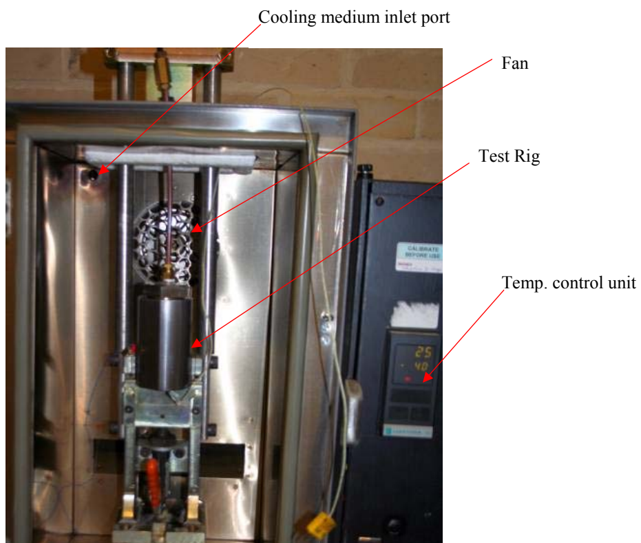
Figure 3 Close up of environmental test chamber
