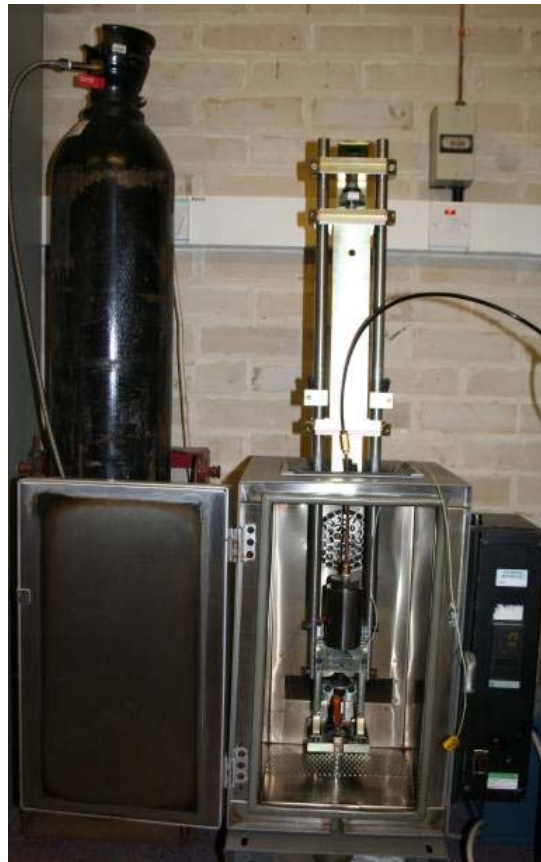
Figure 4 Test Chamber with CO 2 cylinder attached
