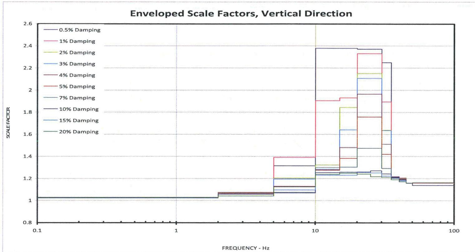
Figure 03.07.01-29 S1.278: Enveloped Scale Factors for Vertical Response Spectra, Reactor Service Water (RSW) Piping Tunnel
