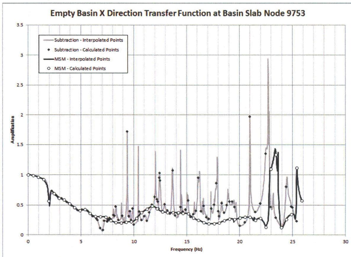
**Figure 03.07.01-29 S1.37: X Direction Transfer Function, Basin Slab Node 9753
