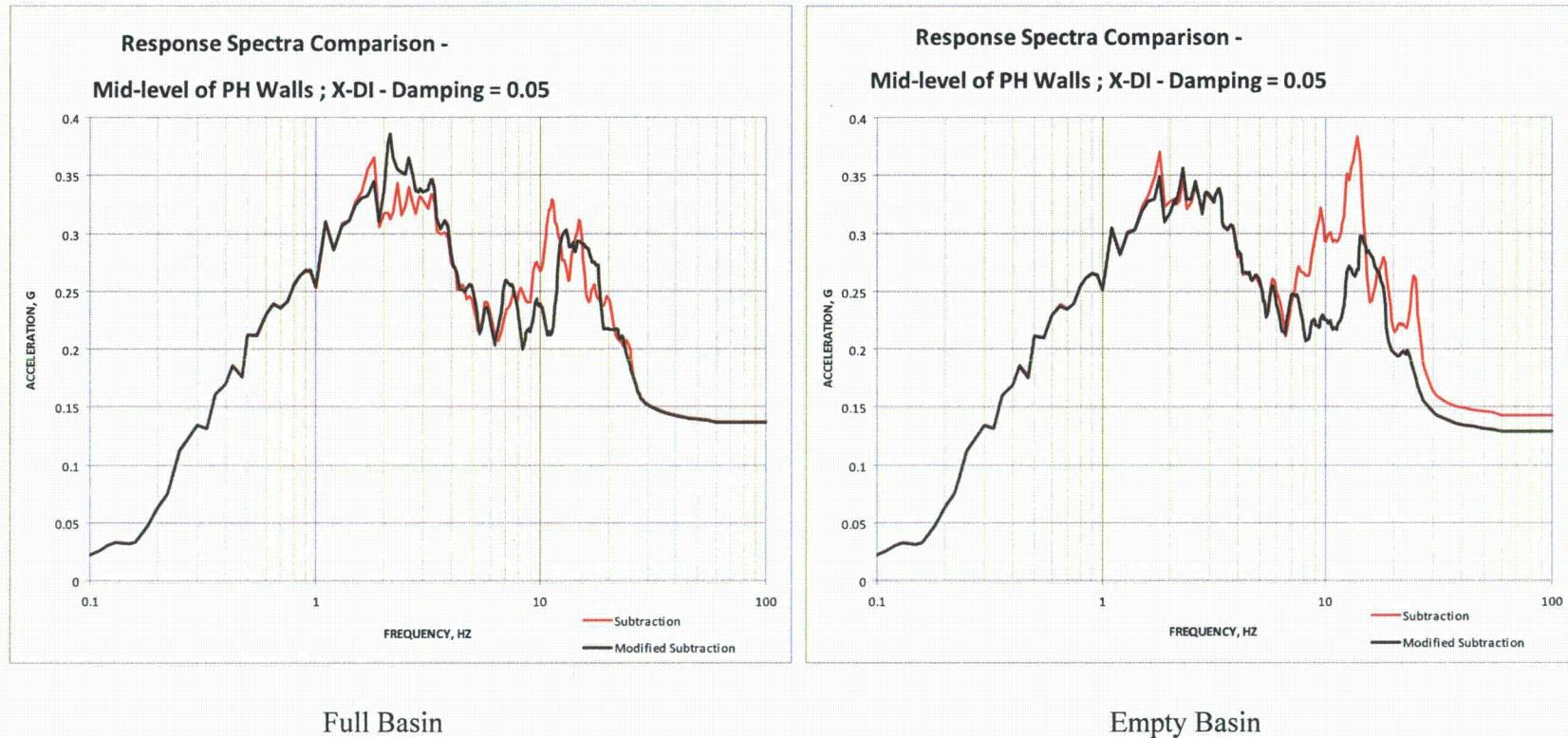
Figure 03.07.01-29 S1.49: Mid-Level Pump House Walls (Group 2) - X-Direction
