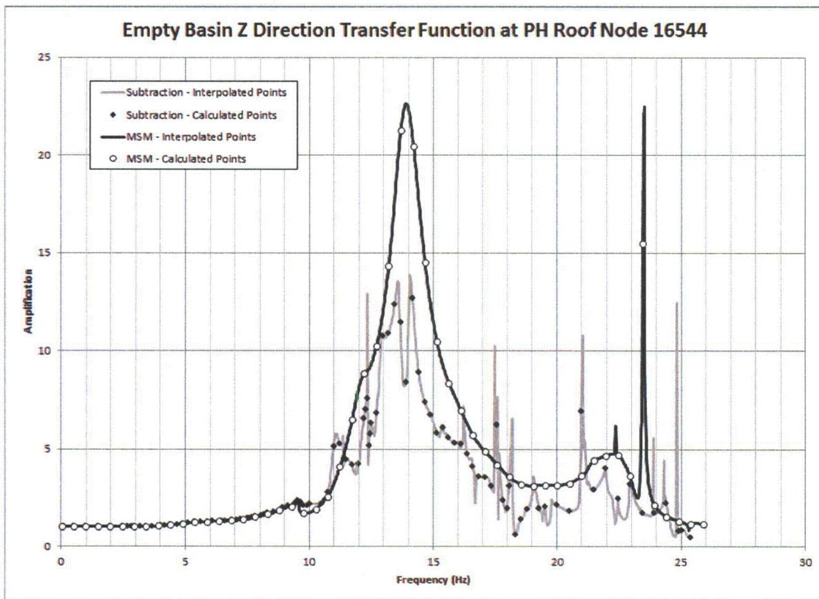
**Figure 03.07.01-29 S1.36: Z Direction Transfer Function, PH Roof Node 16544
