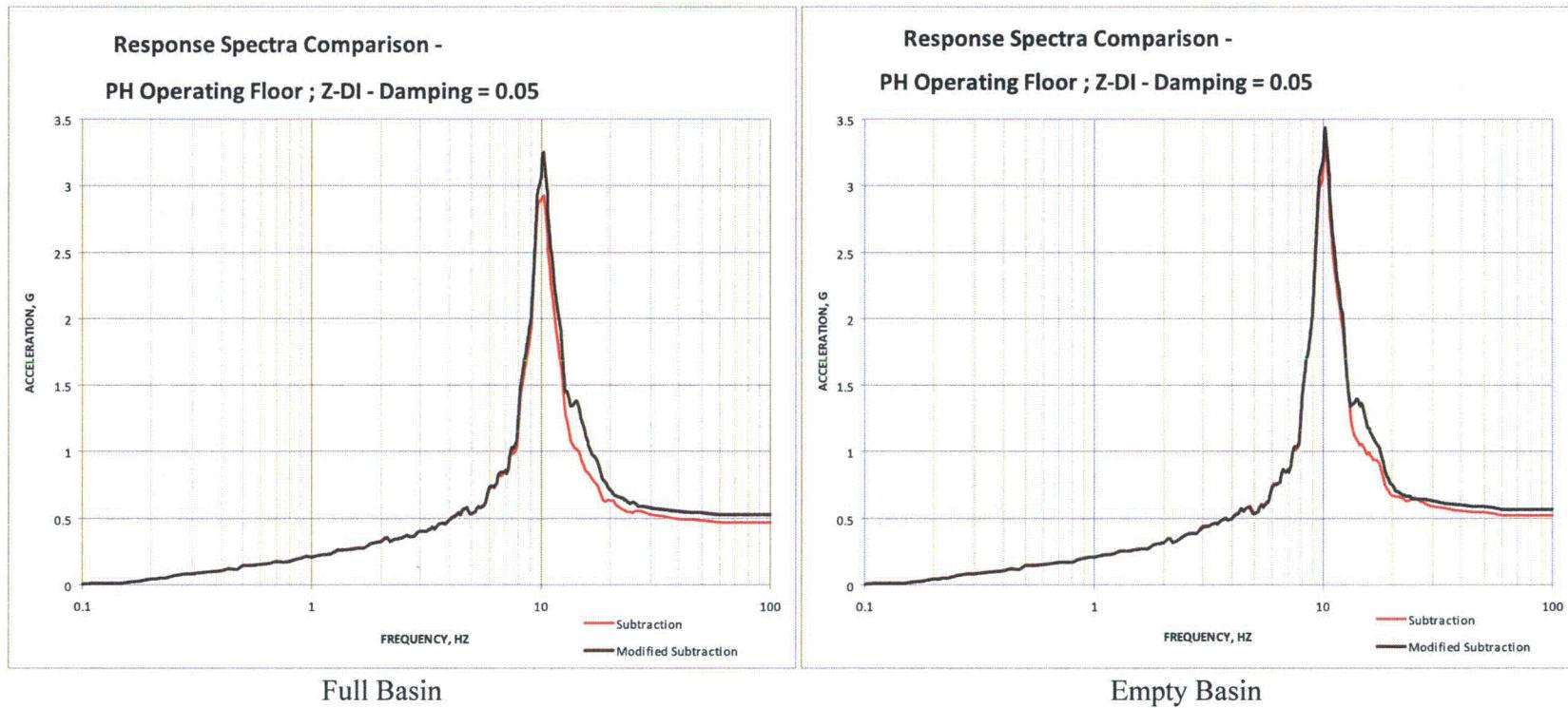
**Figure 03.07.01-29 S1.57: Pump House Operating Floor (Group 4) - Z-Direction**
