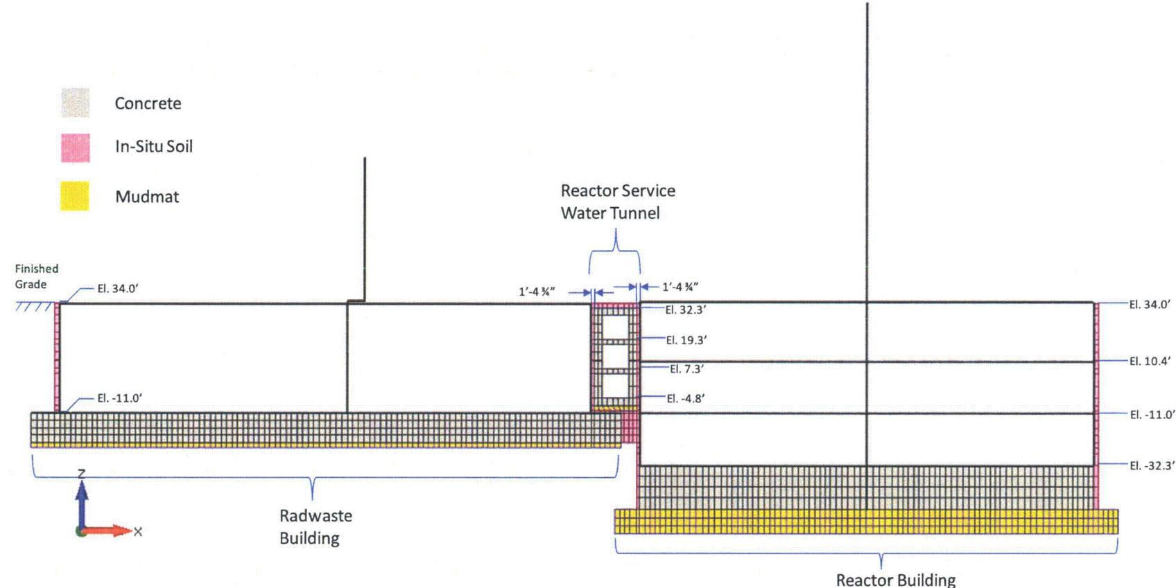
**Figure 03.07.01-29 S1.80: SSSI 2D Model of RB + RSW Piping Tunnel + RWB
