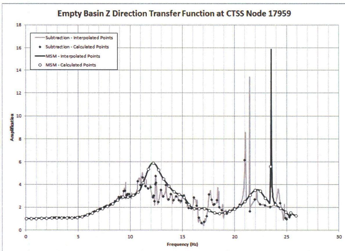
**Figure 03.07.01-29 S1.42: Z Direction Transfer Function, CTSS Node 17959
