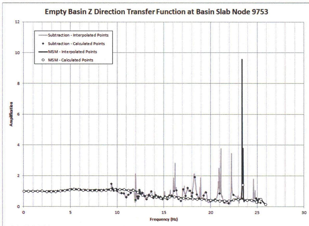
**Figure 03.07.01-29 S1.39: Z Direction Transfer Function, Basin Slab Node 9753
