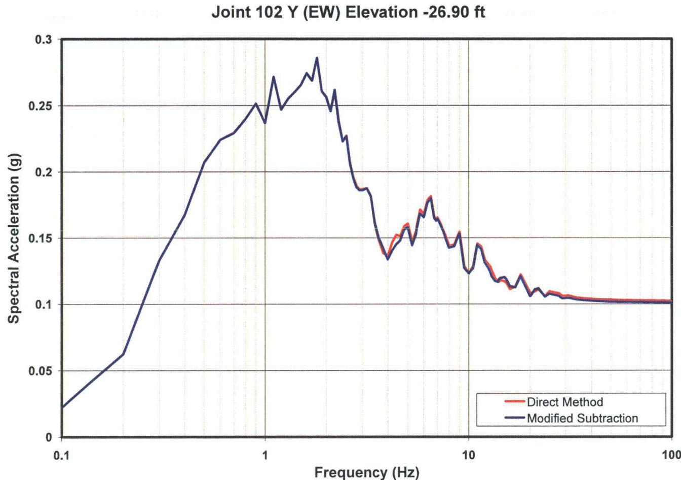
**Figure 03.07.01-29 S1.6: 5% Damped Acceleration Response Spectra Comparison
