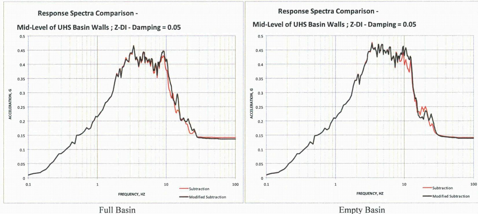
**Figure 03.07.01-29 S1.63: Mid-Level of UHS Basin Walls (Group 6) - Z-Direction**
