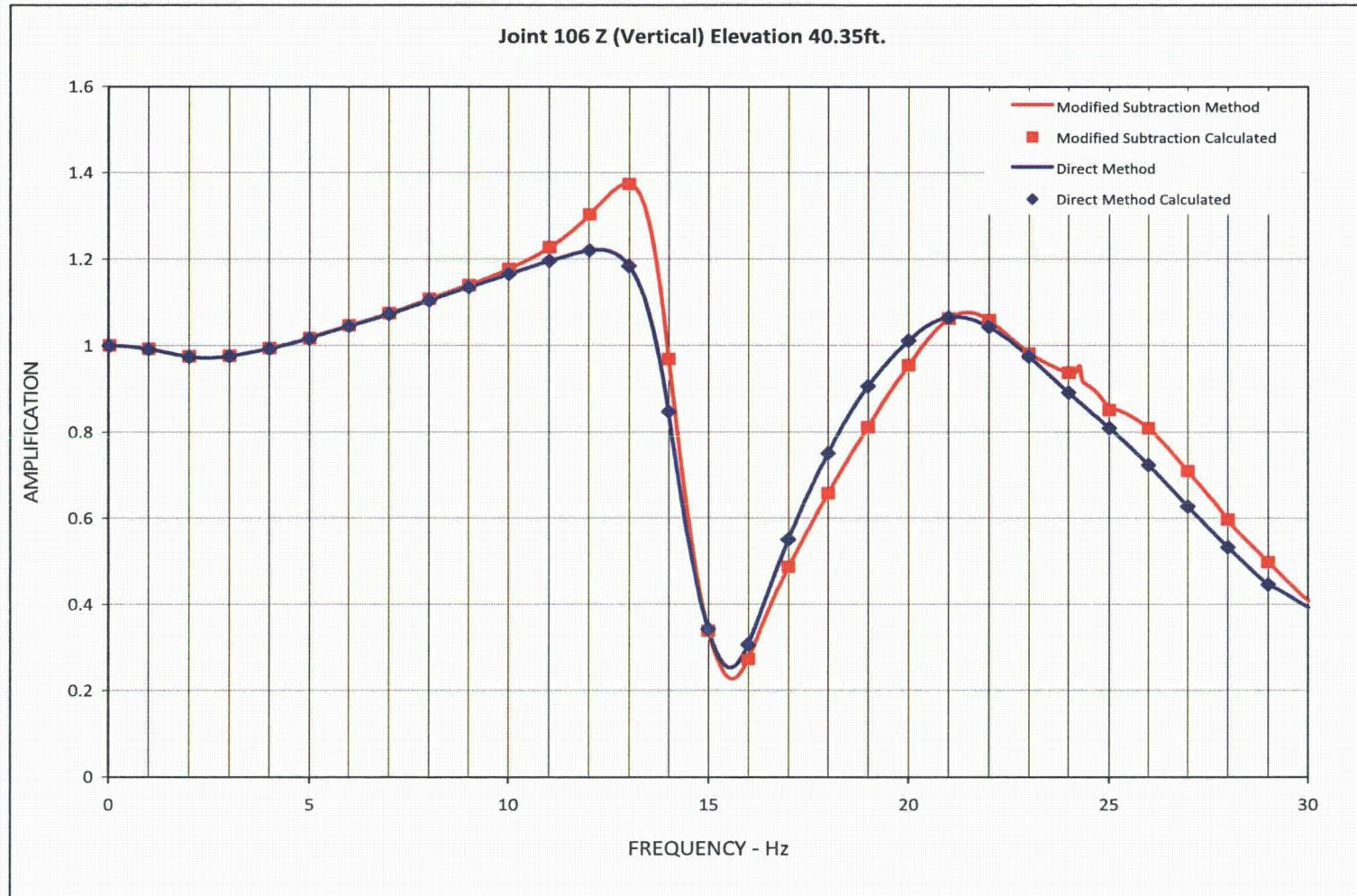
**Figure 03.07.01-29 S1.17: Interpolated and Calculated Transfer Function Comparison
