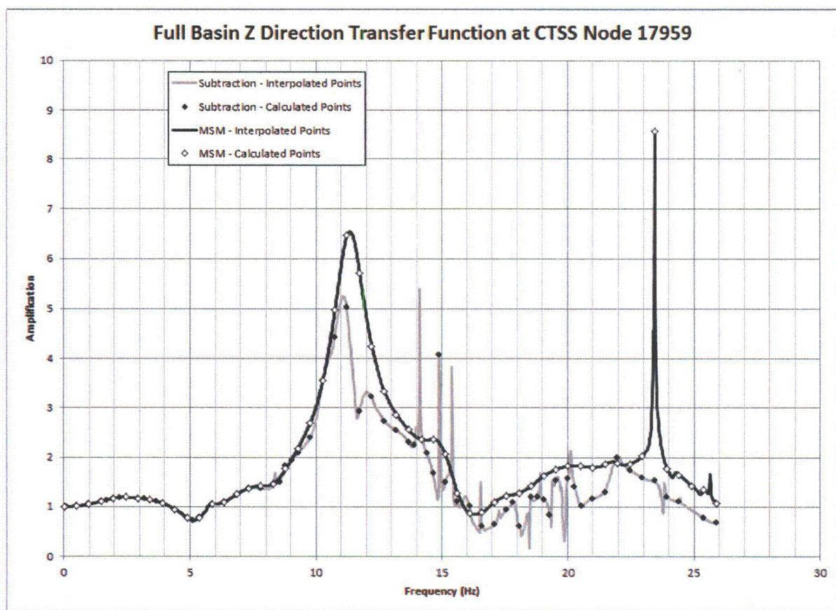
**Figure 03.07.01-29 S1.30: Z Direction Transfer Function, CTSS Node 17959
