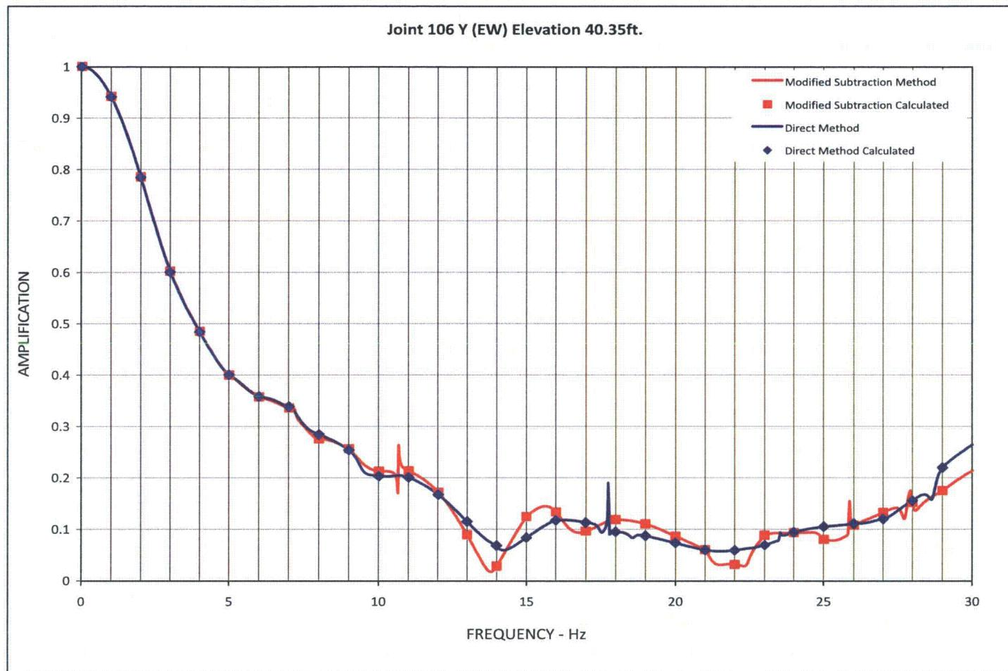
**Figure 03.07.01-29 S1.16: Interpolated and Calculated Transfer Function Comparison
