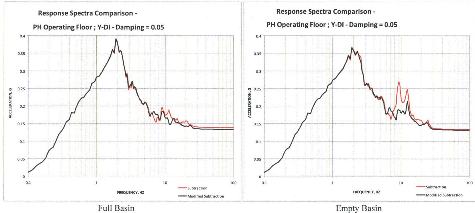
Figure 03.07.01-29 S1.56: Pump House Operating Floor (Group 4) - Y-Direction
