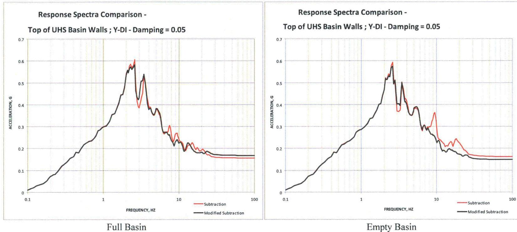
Figure 03.07.01-29 S1.65: Top of UHS Basin Walls (Group 7) - Y-Direction
