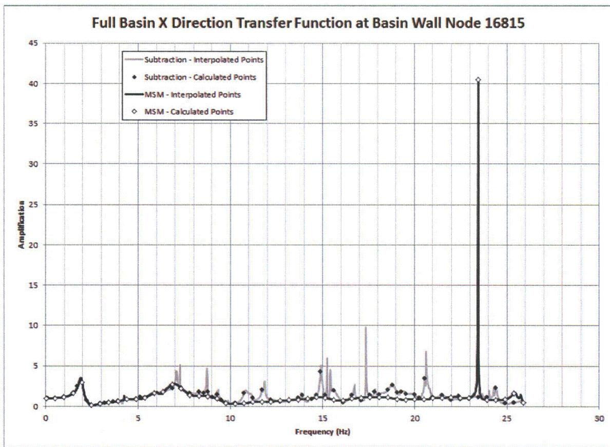
**Figure 03.07.01-29 S1.31: X Direction Transfer Function, Basin Wall Node 16815
