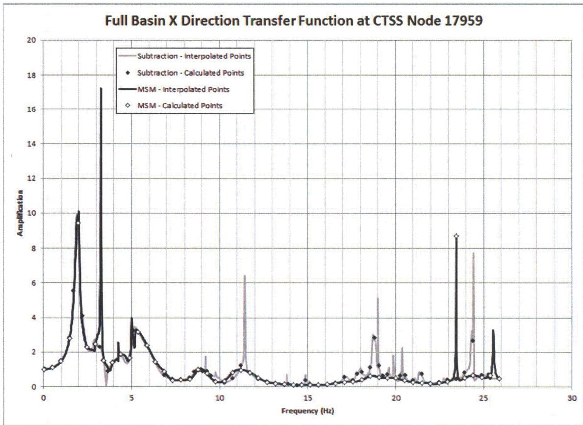
**Figure 03.07.01-29 S1.28: X Direction Transfer Function, CTSS Node 17959
