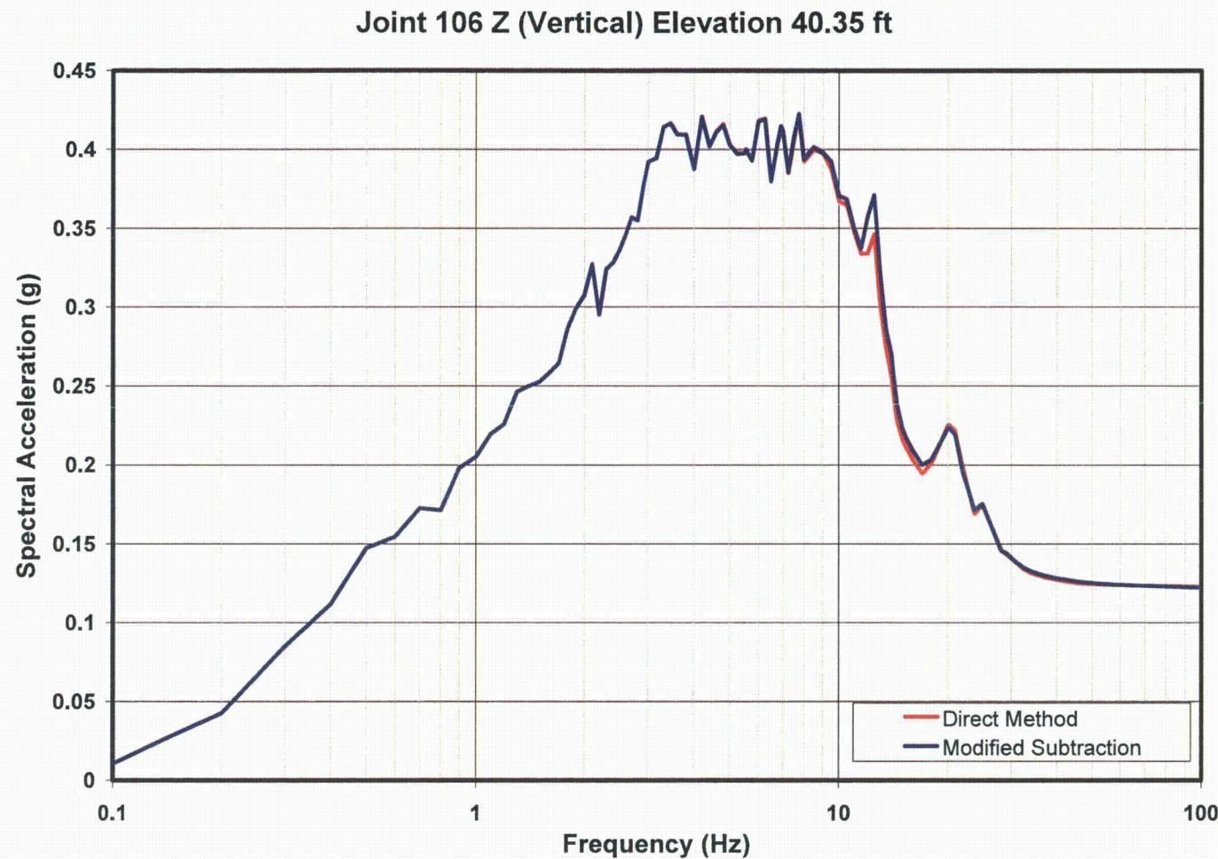
**Figure 03.07.01-29 S1.10: 5% Damped Acceleration Response Spectra Comparison
