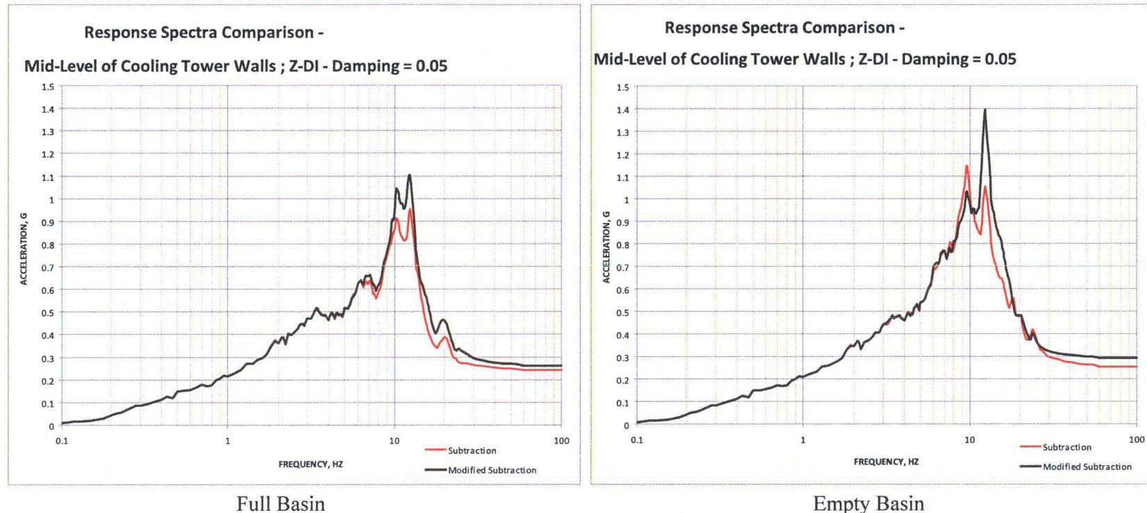
**Figure 03.07.01-29 S1.72: Mid-Level of Cooling Tower Walls (Group 9) - Z-Direction**
