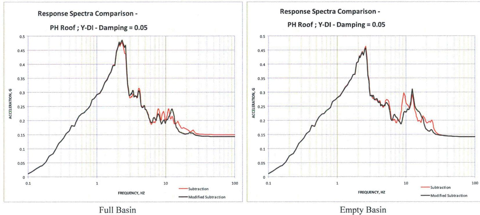
**Figure 03.07.01-29 S1.53: Pump House Roof (Group 3) - Y-Direction**
