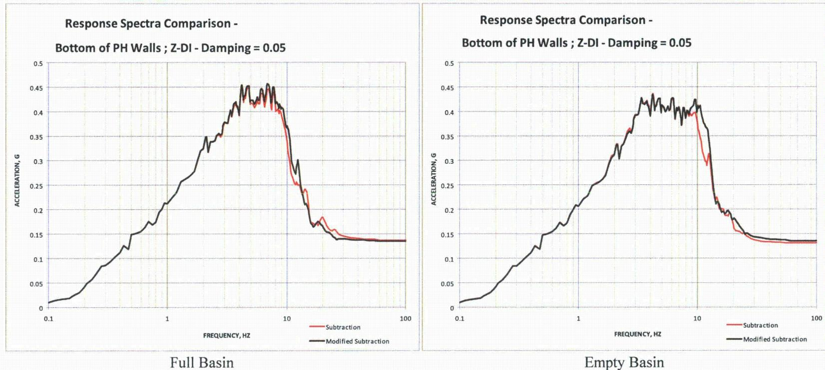
Figure 03.07.01-29 S1.48: Bottom of Pump House Walls (Group 1) - Z-Direction
