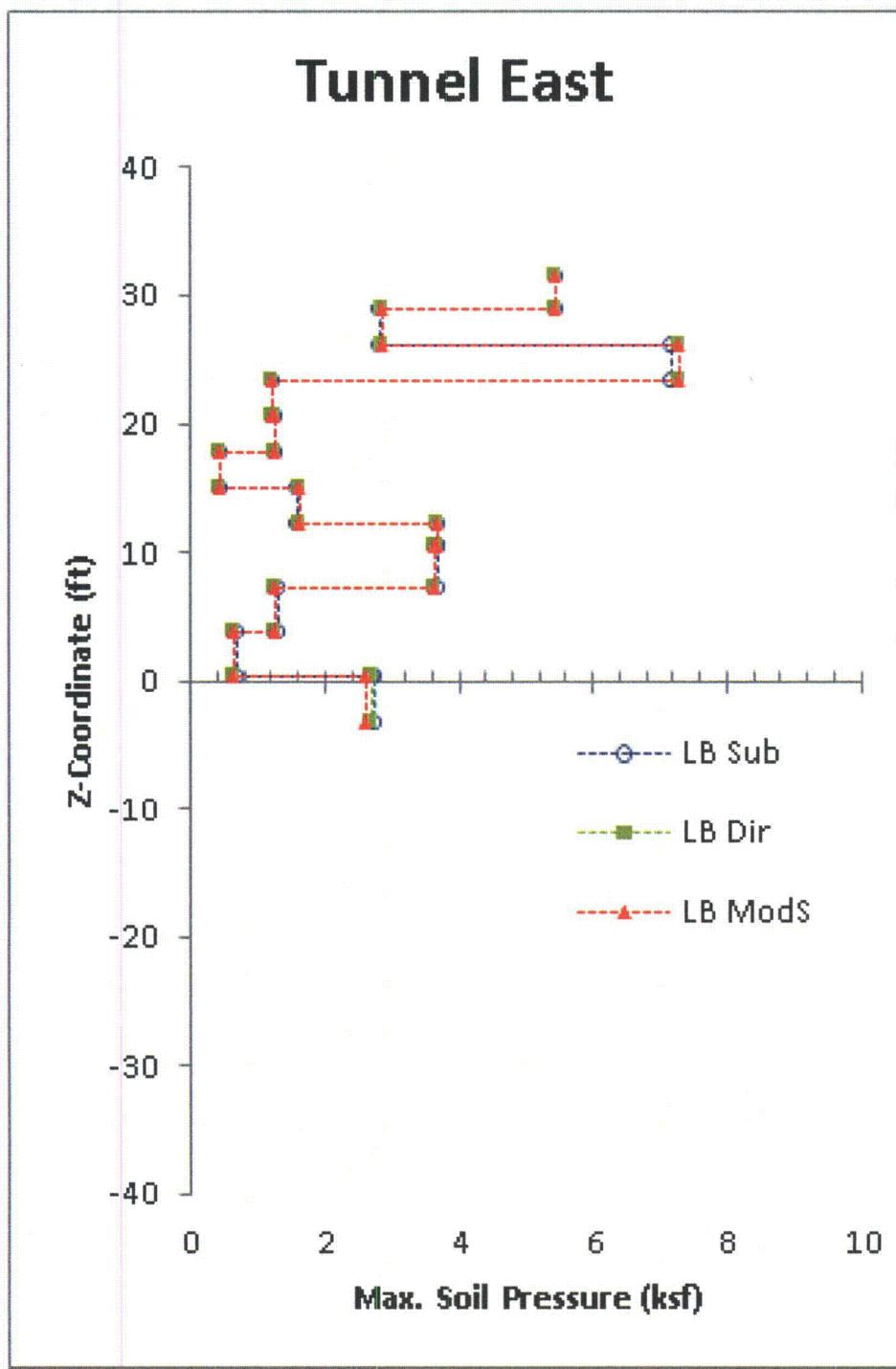
Figure 03.07.01-29 S1.89: Maximum Absolute Soil Pressure (Subtraction vs. Direct vs. Modified Subtraction), RSW Tunnel East Wall, Lower Bound In-Situ
