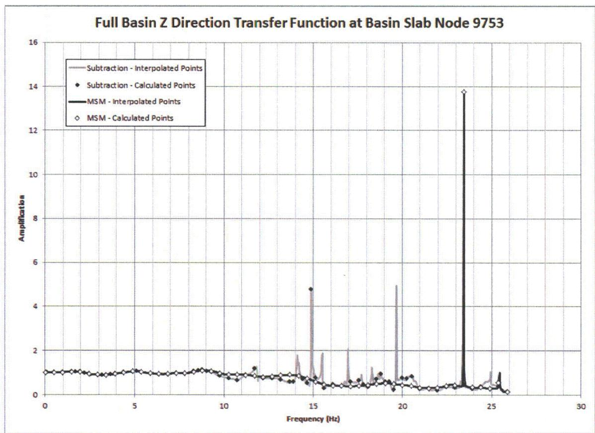
**Figure 03.07.01-29 S1.27: Z Direction Transfer Function, Basin Slab Node 9753
