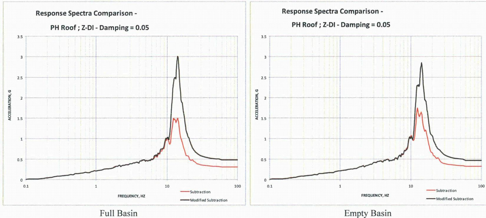
**Figure 03.07.01-29 S1.54: Pump House Roof (Group 3) - Z-Direction**
