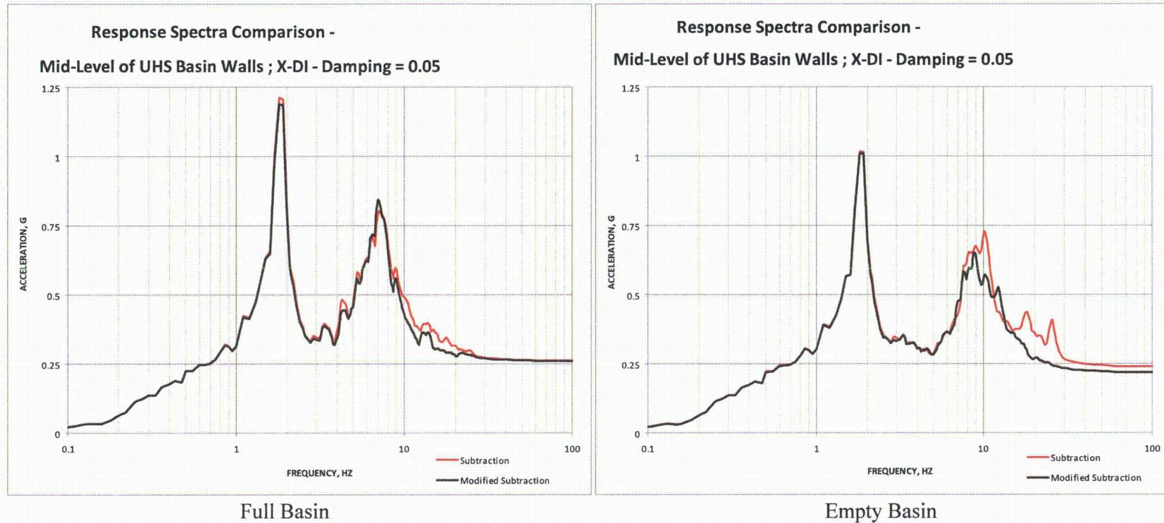
Figure 03.07.01-29 S1.61: Mid-Level of UHS Basin Walls (Group 6) - X-Direction
