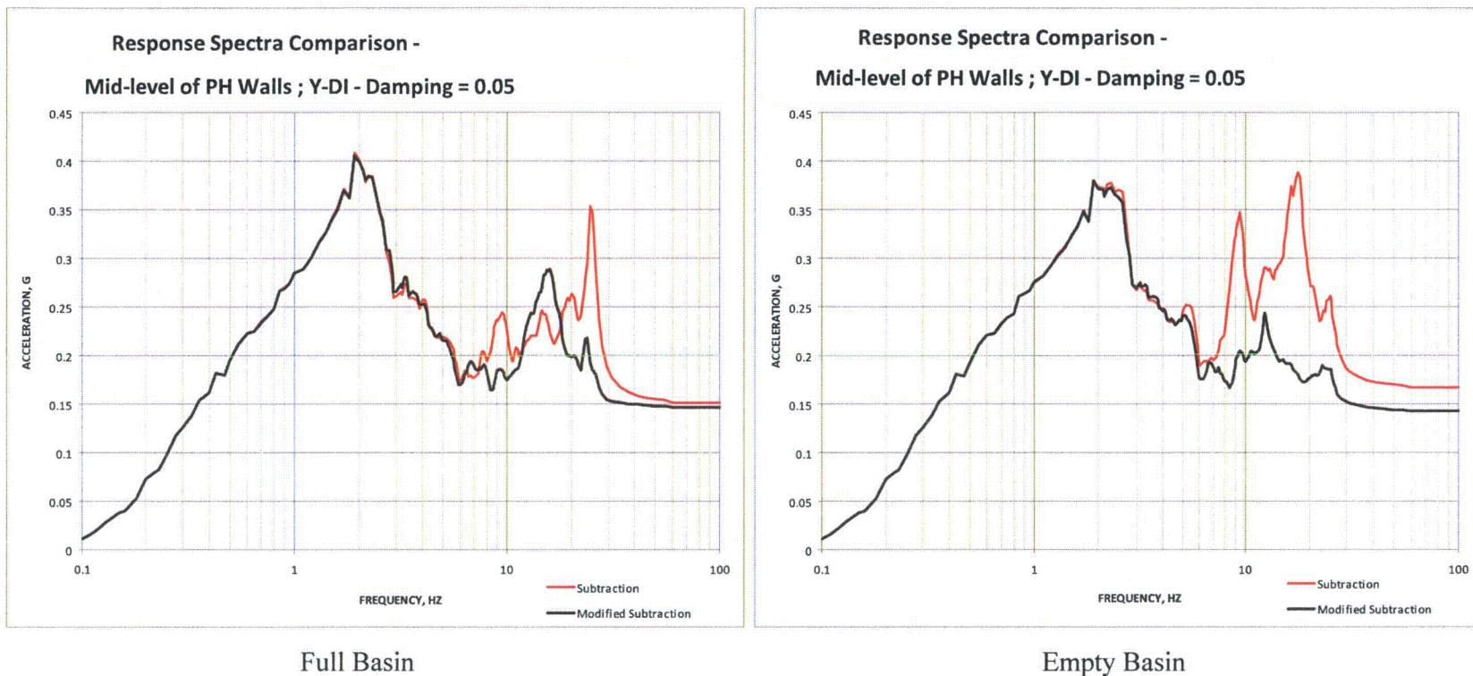
**Figure 03.07.01-29 S1.50: Mid-Level Pump House Walls (Group 2) - Y-Direction**
