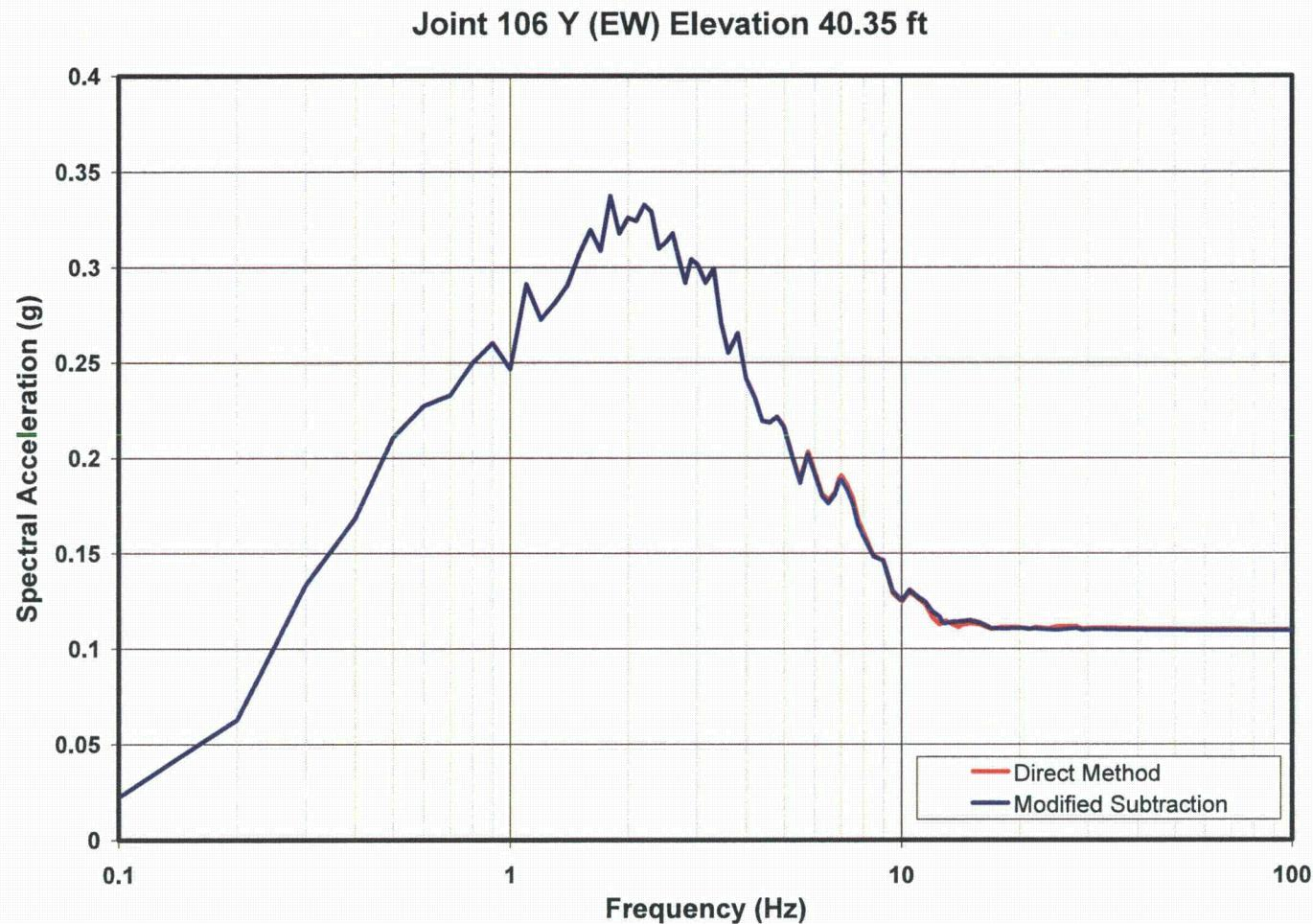
**Figure 03.07.01-29 S1.9: 5% Damped Acceleration Response Spectra Comparison
