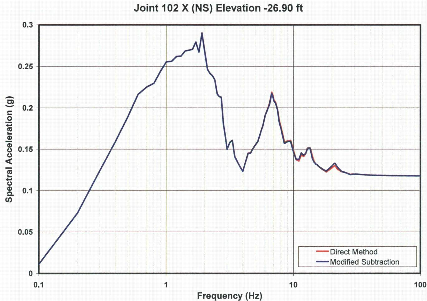
**Figure 03.07.01-29 S1.5: 5% Damped Acceleration Response Spectra Comparison**
