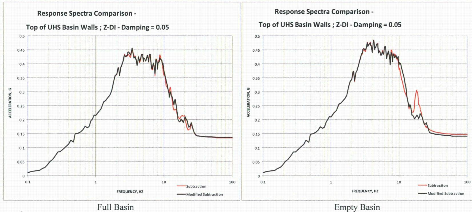
Figure 03.07.01-29 S1.66: Top of UHS Basin Walls (Group 7) - Z-Direction
