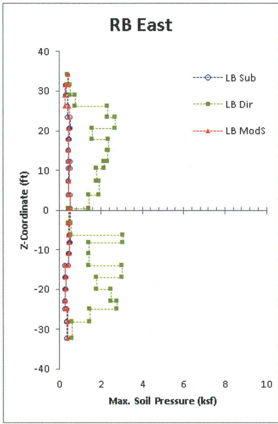
Figure 03.07.01-29 S1.87: Maximum Absolute Soil Pressure (Subtraction vs. Direct vs. Modified Subtraction), RB East Wall, Lower Bound In-Situ
