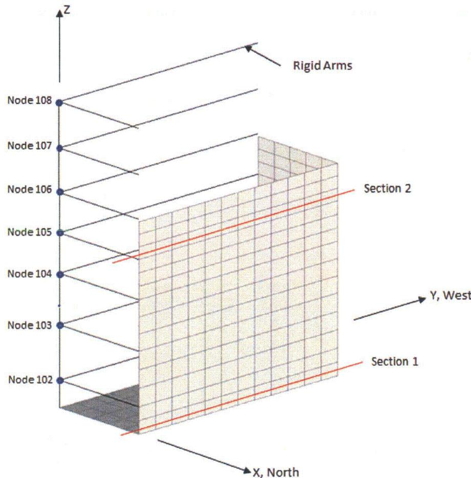
Figure 03.07.01-29 S1.2: Control Building Section Force Calculation Location
