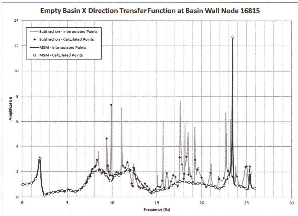
**Figure 03.07.01-29 S1.43: X Direction Transfer Function, Basin Wall Node 16815
