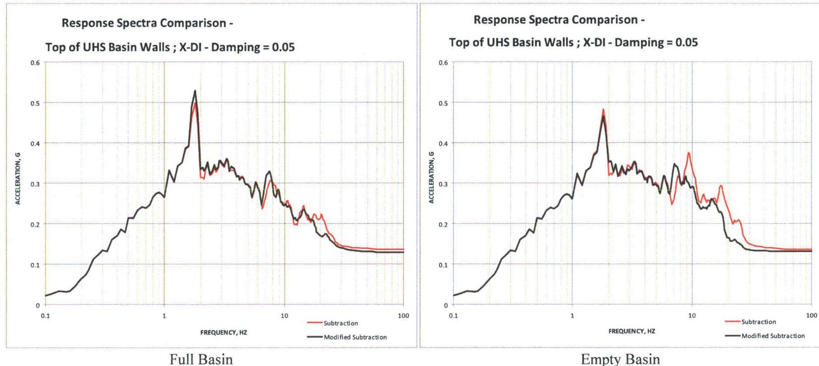
**Figure 03.07.01-29 S1.64: Top of UHS Basin Walls (Group 7) - X-Direction**
