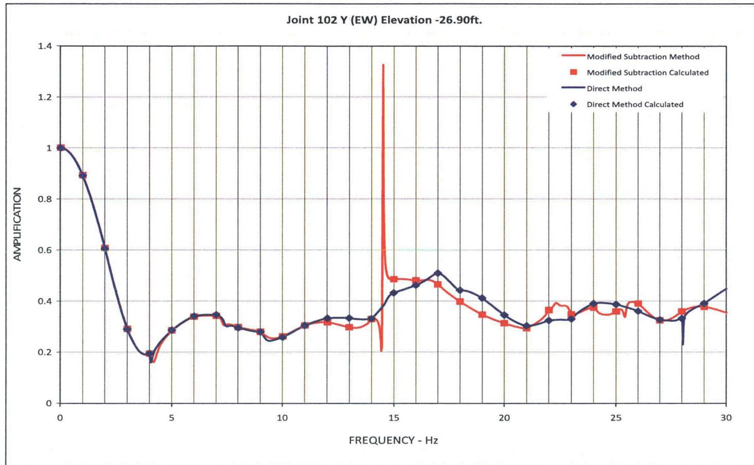
**Figure 03.07.01-29 S1.13: Interpolated and Calculated Transfer Function Comparison
