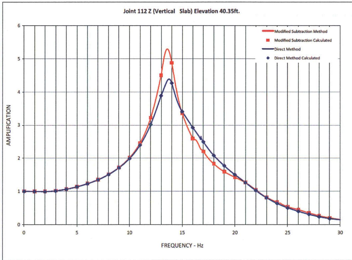
**Figure 03.07.01-29 S1.18: Interpolated and Calculated Transfer Function Comparison
