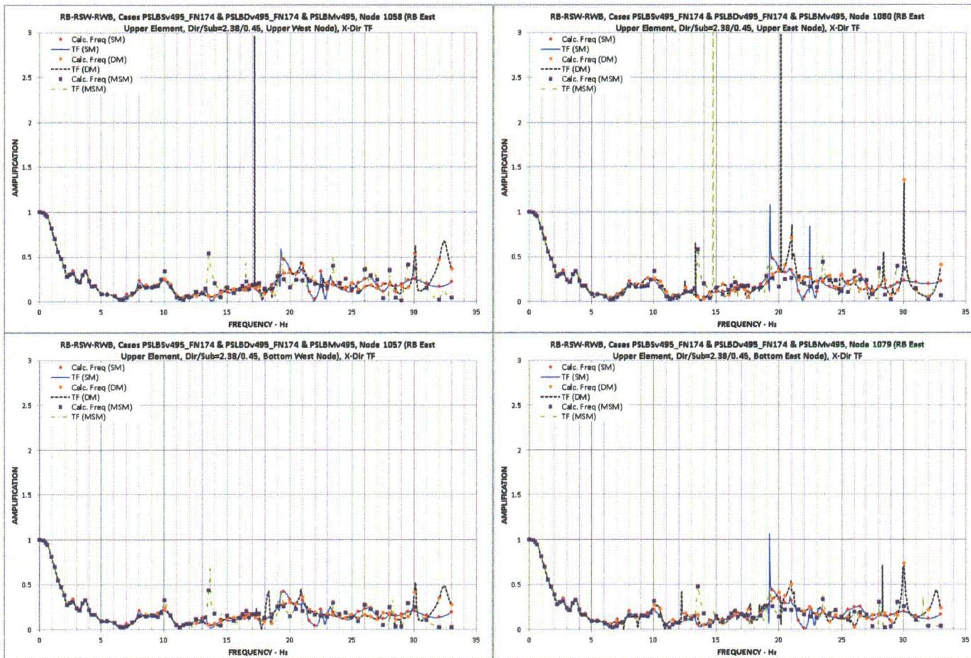
Figure 03.07.01-29 S1.100 - Transfer Functions (Subtraction vs. Direct vs. Mod. Sub.) of Four Corner Nodes for the Element near RB East Upper, Dir/Sub Max Stress Ratio = 2.38/0.45, X-Dir
