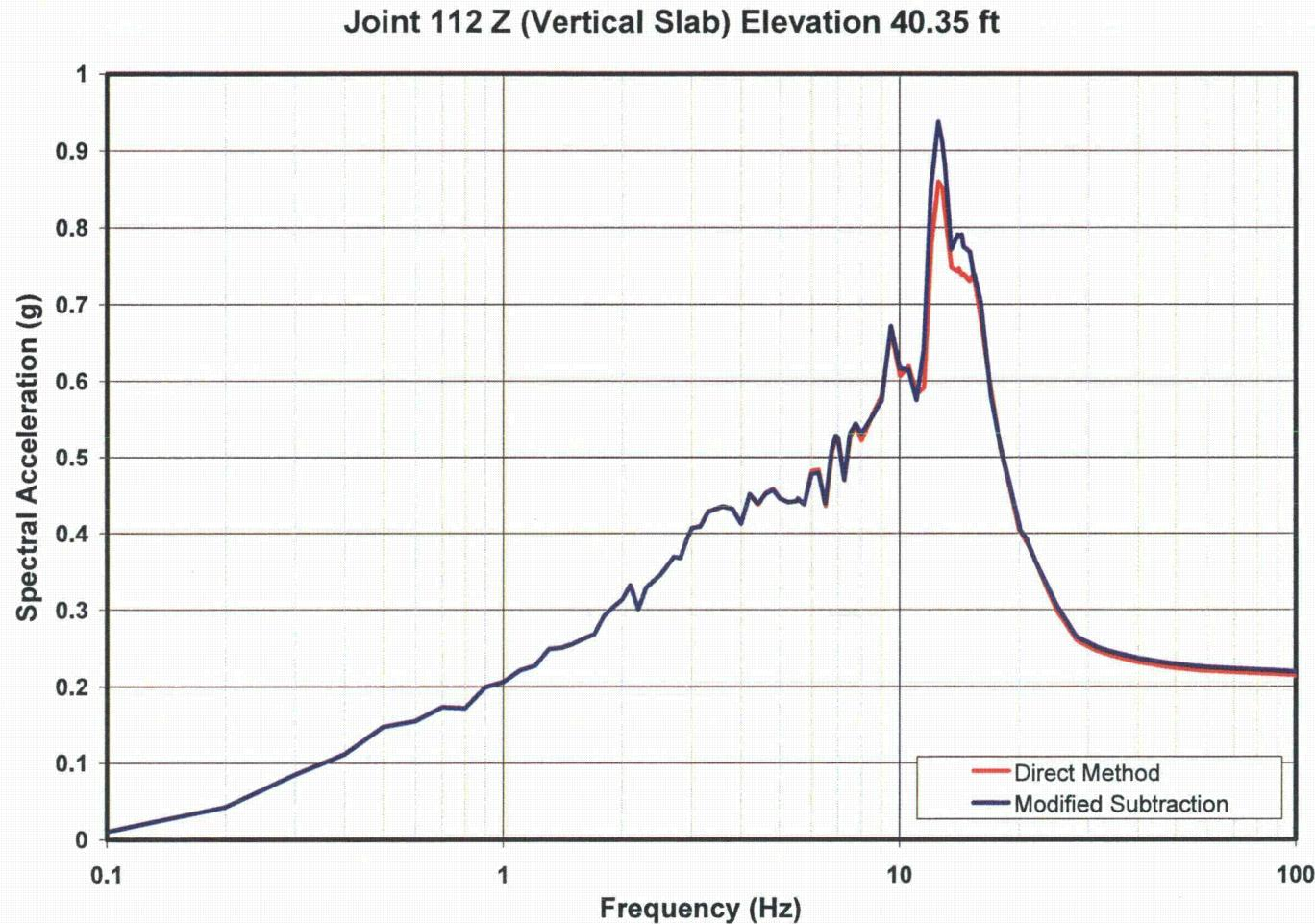
**Figure 03.07.01-29 S1.11: 5% Damped Acceleration Response Spectra Comparison
