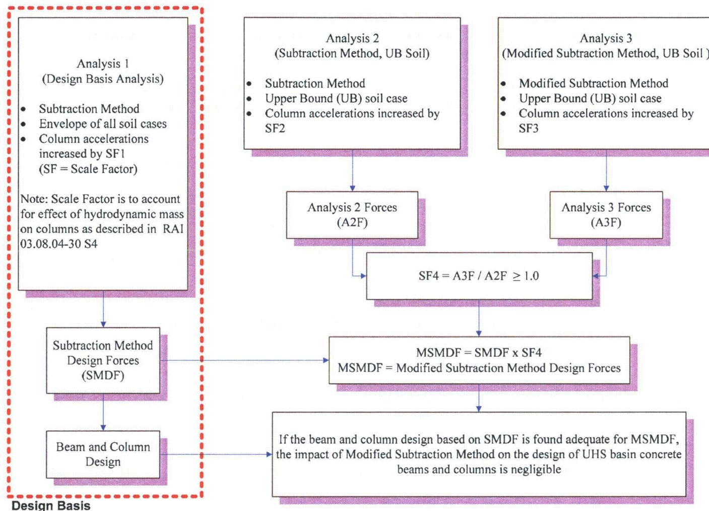
**Figure 03.07.01-29 S1.78: Procedure for Evaluation of UHS Basin Concrete Beams and Columns for Impact of Modified Subtraction Method for Full and Empty Basin Cases**
