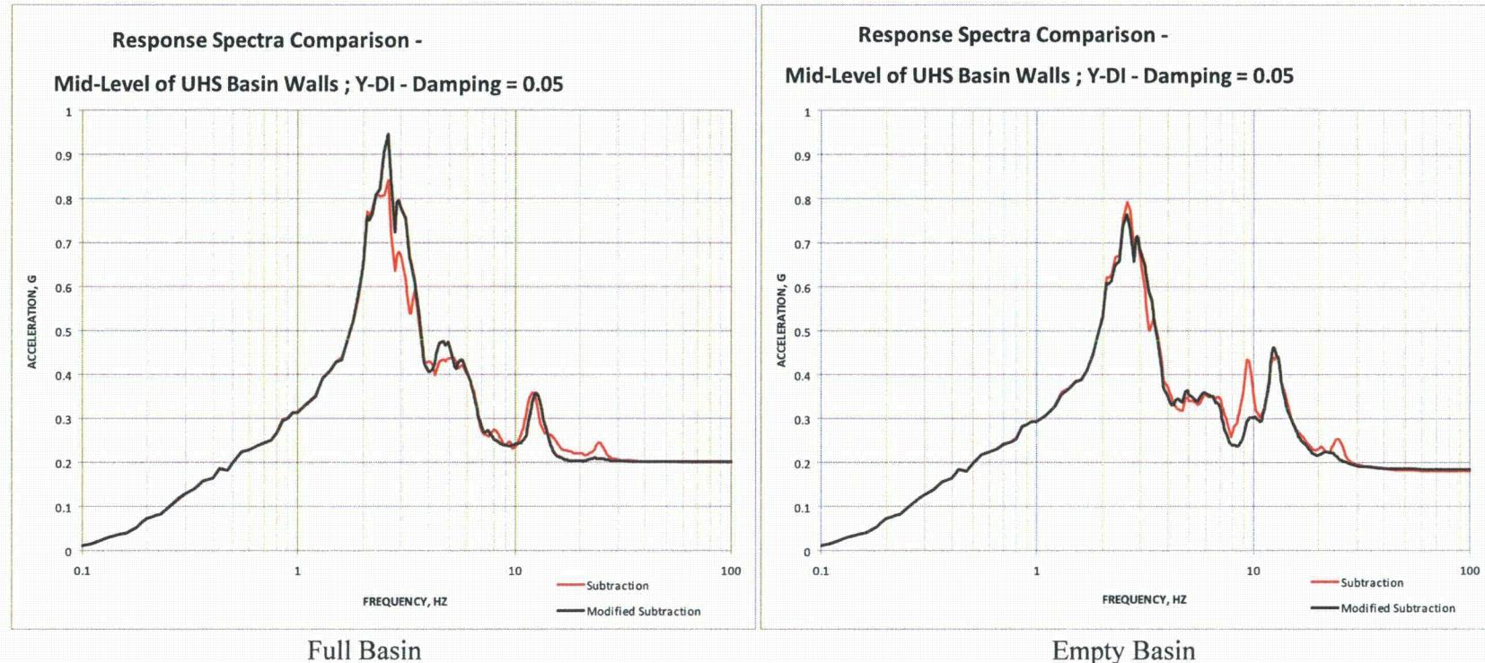
Figure 03.07.01-29 S1.62: Mid-Level of UHS Basin Walls (Group 6) - Y-Direction
