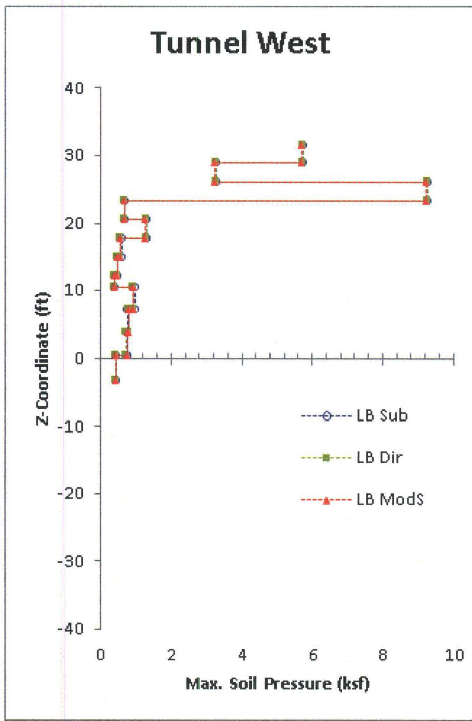
Figure 03.07.01-29 S1.90: Maximum Absolute Soil Pressure (Subtraction vs. Direct vs. Modified Subtraction), RSW Tunnel West Wall, Lower Bound In-Situ
