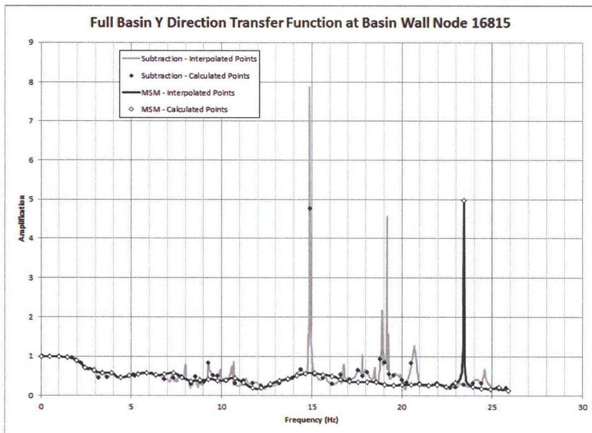
**Figure 03.07.01-29 S1.32: Y Direction Transfer Function, Basin Wall Node 16815
