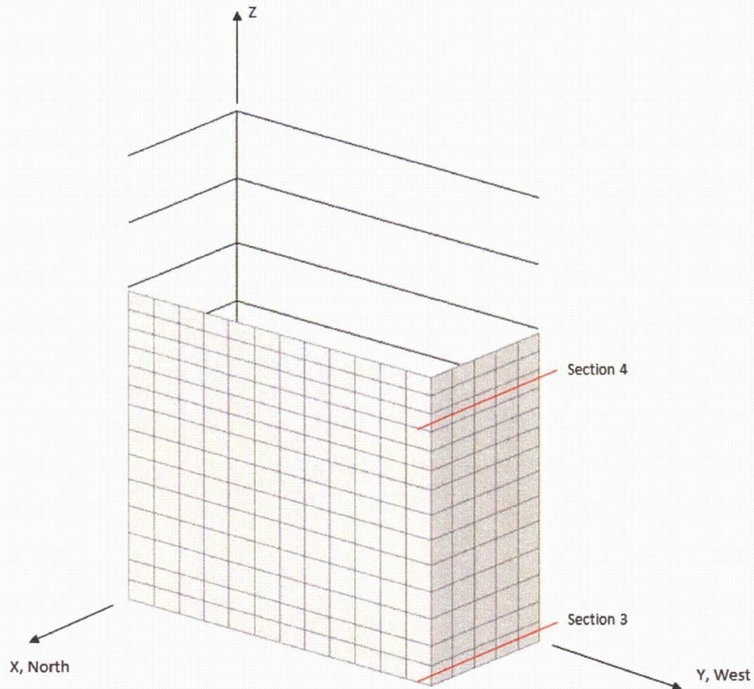
**Figure 03.07.01-29 S1.3: Control Building Section Force Calculation Location**
