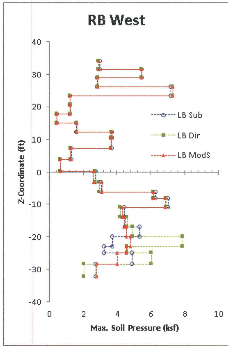
Figure 03.07.01-29 S1.88: Maximum Absolute Soil Pressure (Subtraction vs. Direct vs. Modified Subtraction), RB West Wall, Lower Bound In-Situ
