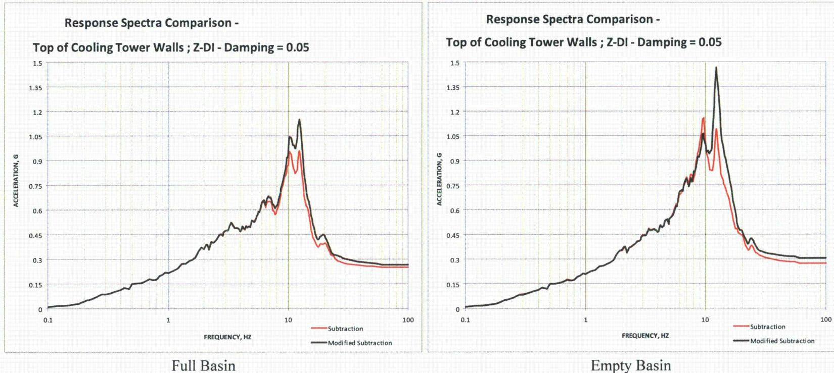
Figure 03.07.01-29 S1.75: Top of Cooling Tower Walls (Group 10) - Z-Direction
