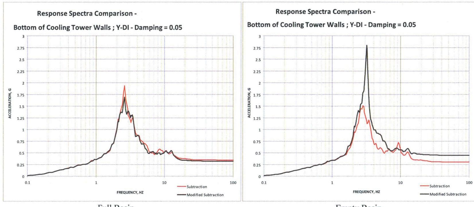
Figure 03.07.01-29 S1.68: Bottom of Cooling Tower Walls (Group 8) - Y-Direction
