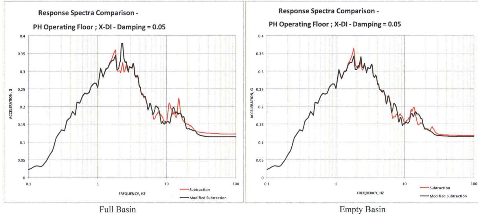
**Figure 03.07.01-29 S1.55: Pump House Operating Floor (Group 4) - X-Direction**
