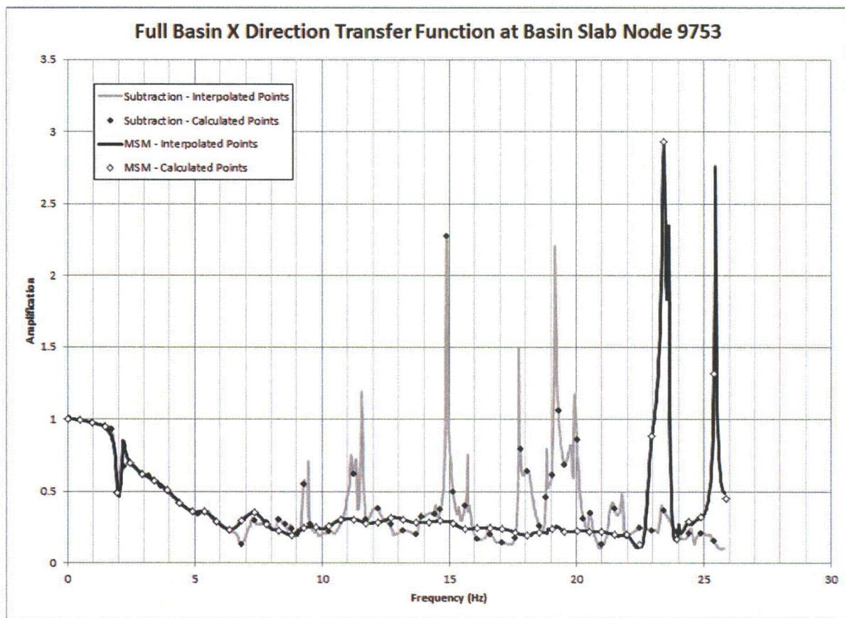
**Figure 03.07.01-29 S1.25: X Direction Transfer Function, Basin Slab Node 9753
