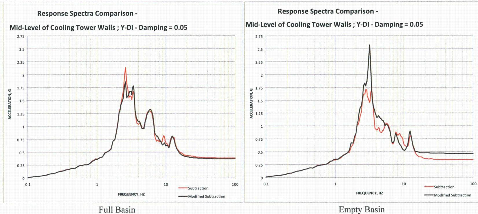
**Figure 03.07.01-29 S1.71: Mid-Level of Cooling Tower Walls (Group 9) - Y-Direction**
