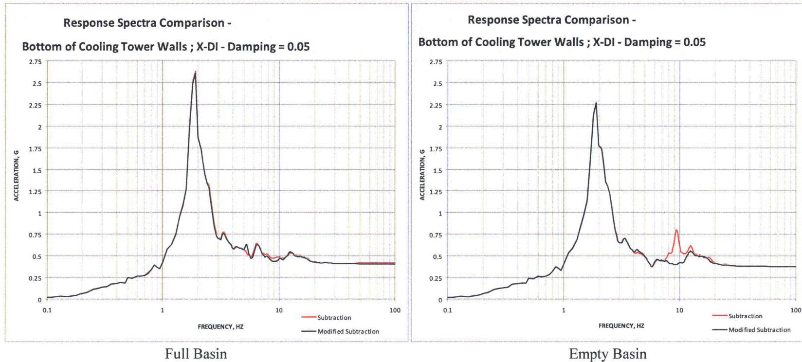
**Figure 03.07.01-29 S1.67: Bottom of Cooling Tower Walls (Group 8) - X-Direction**
