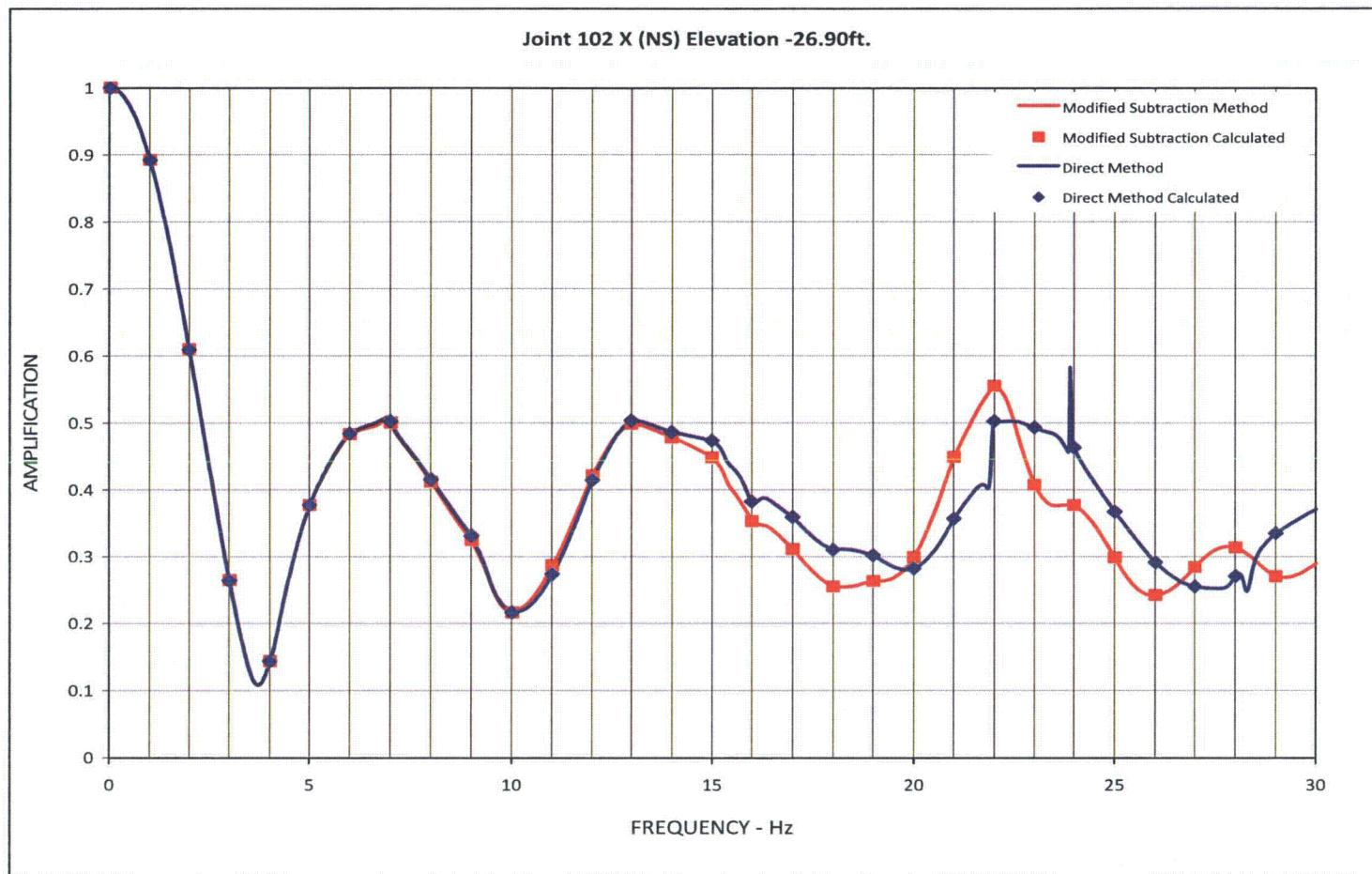
**Figure 03.07.01-29 S1.12: Interpolated and Calculated Transfer Function Comparison
