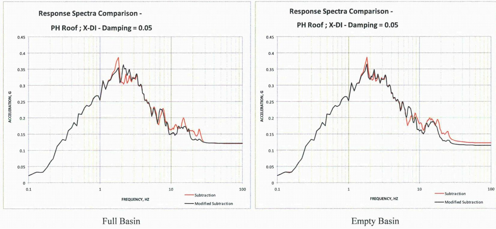
Figure 03.07.01-29 S1.52: Pump House Roof (Group 3) - X-Direction
