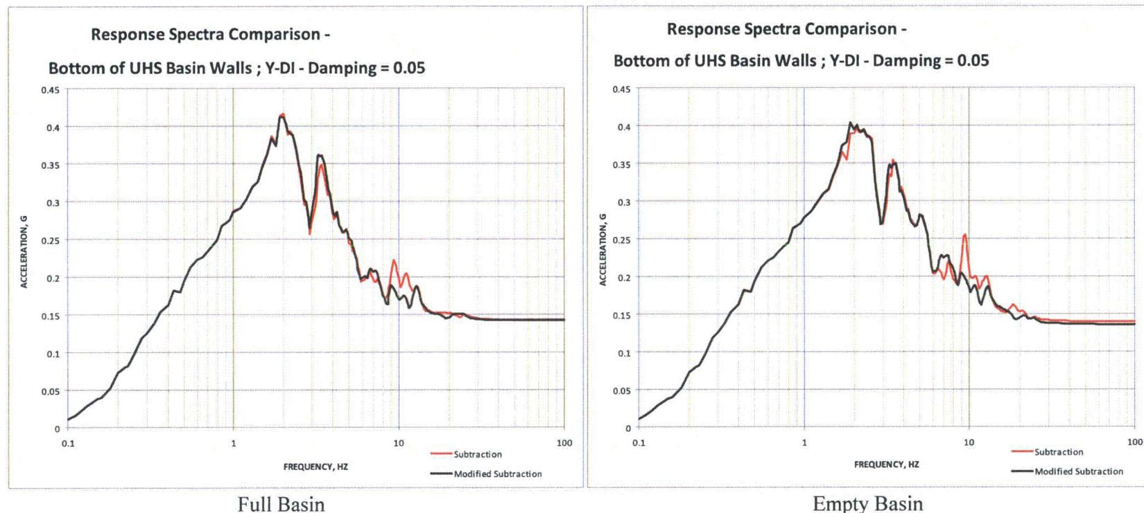
Figure 03.07.01-29 S1.59: Bottom of UHS Basin Walls (Group 5) - Y-Direction
