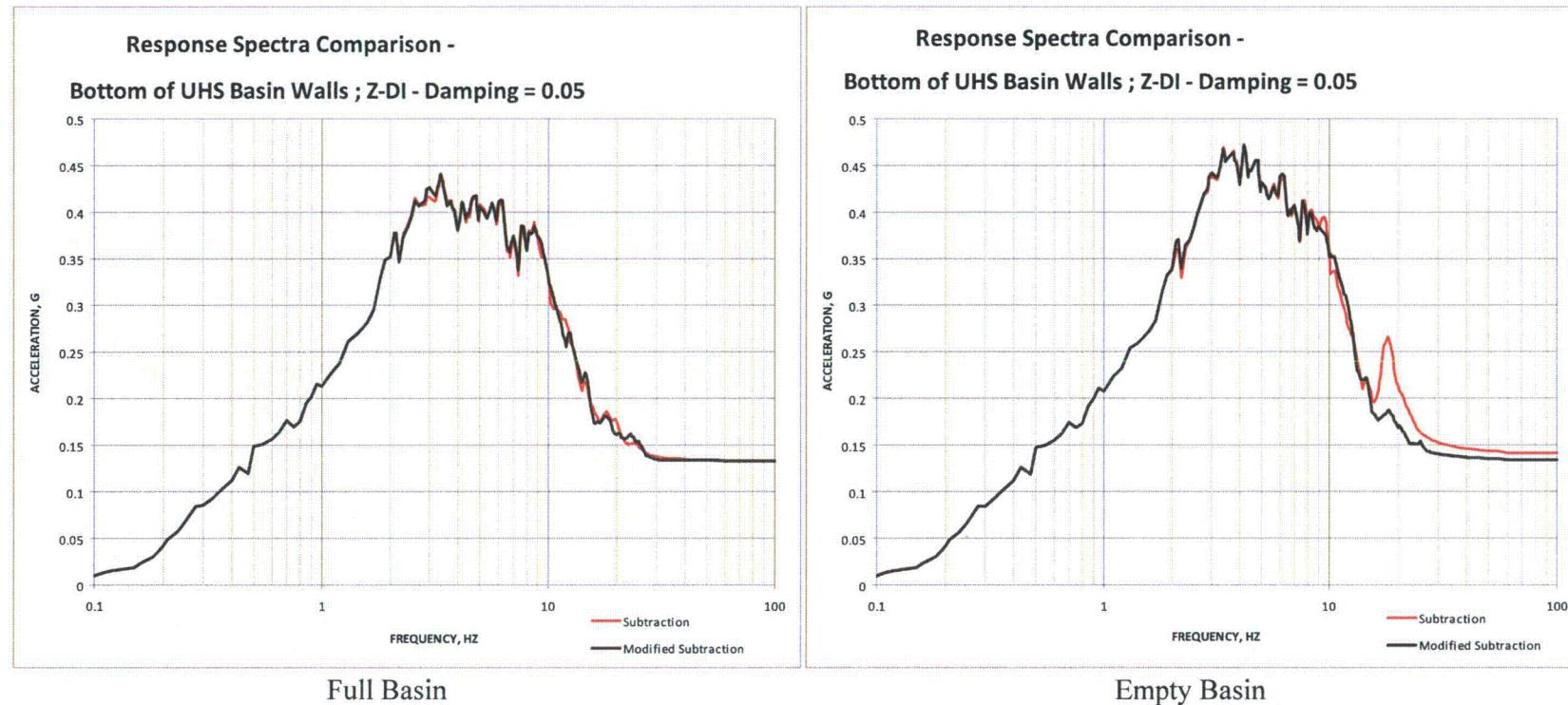
Figure 03.07.01-29 S1.60: Bottom of UHS Basin Walls (Group 5) - Z-Direction
