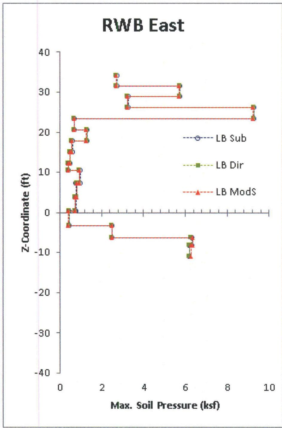
Figure 03.07.01-29 S1.91: Maximum Absolute Soil Pressure (Subtraction vs. Direct vs. Modified Subtraction), RWB East Wall, Lower Bound In-Situ
