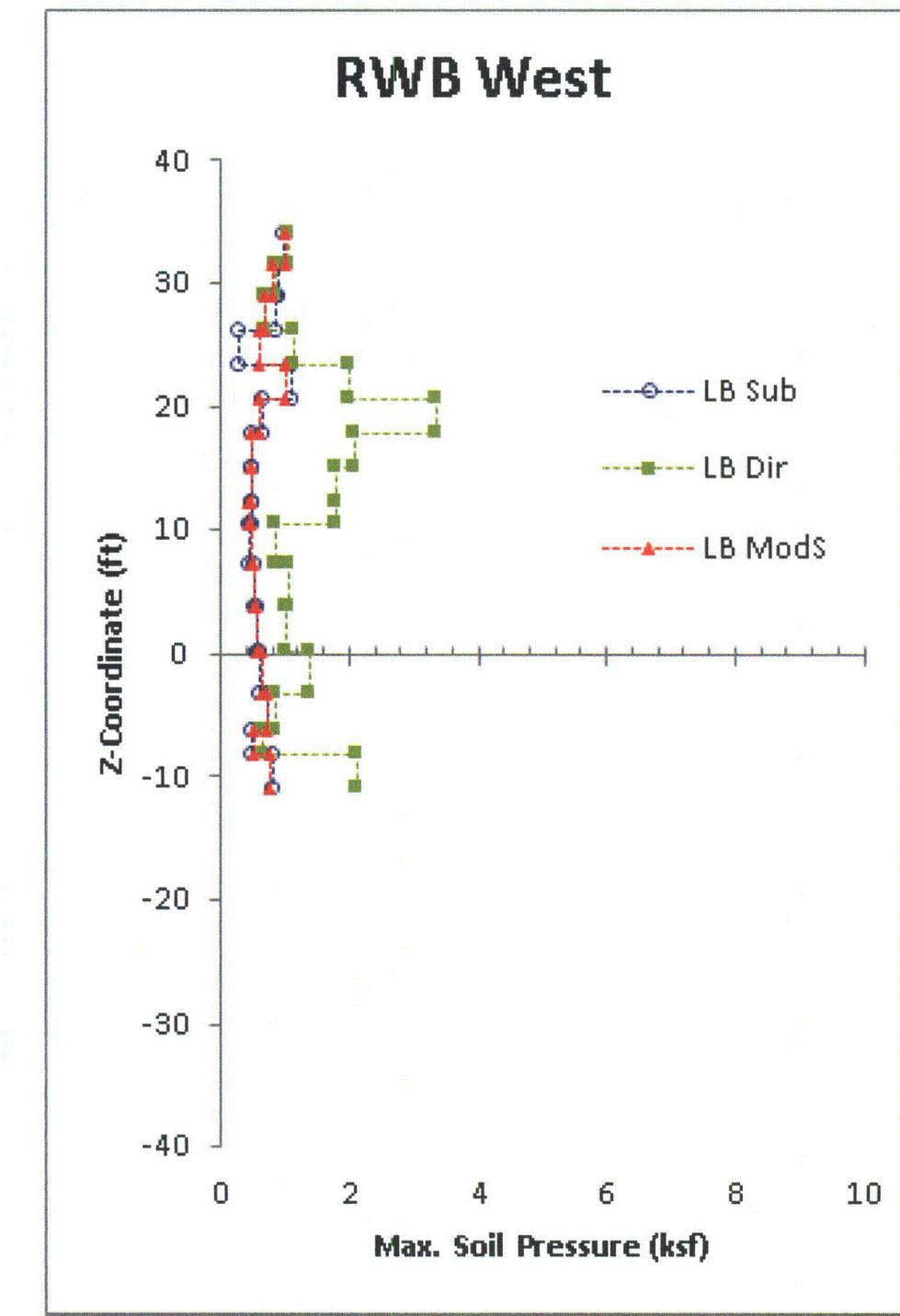
Figure 03.07.01-29 S1.92: Maximum Absolute Soil Pressure (Subtraction vs. Direct vs. Modified Subtraction), RWB West Wall, Lower Bound In-Situ
