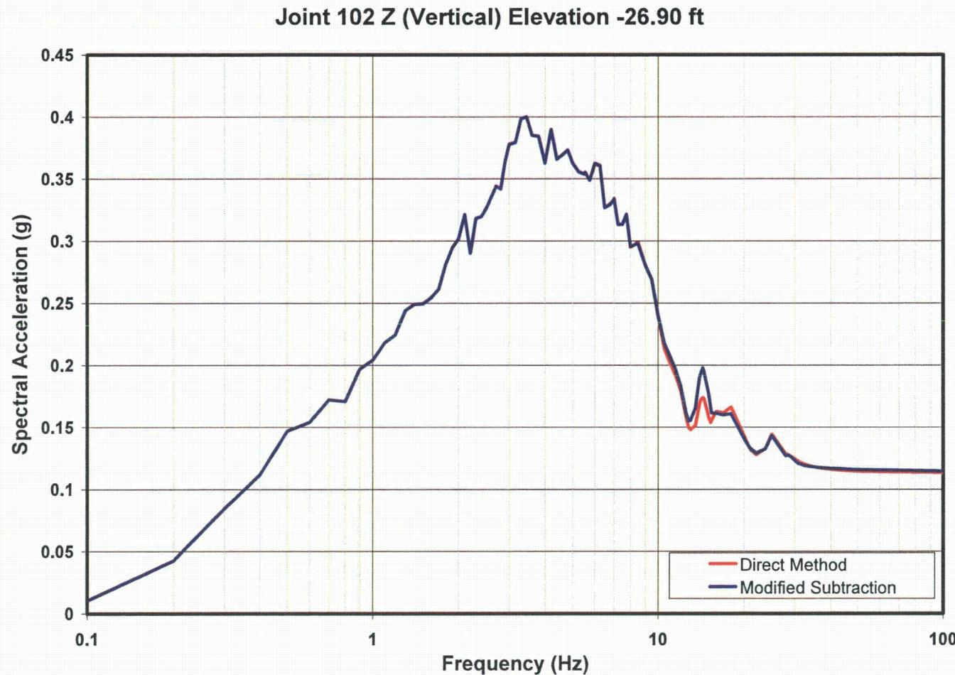
**Figure 03.07.01-29 S1.7: 5% Damped Acceleration Response Spectra Comparison**
