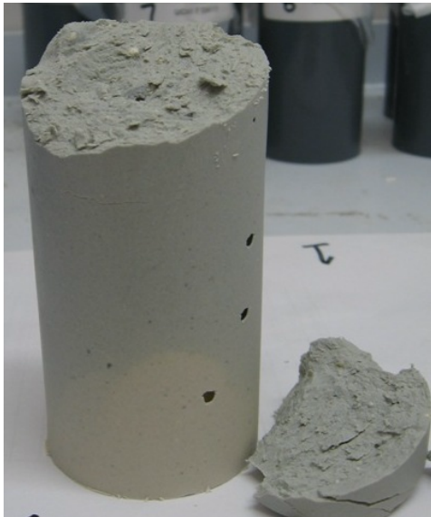
Mix 6. LaFarge MaxCem (70% Joppa Type I/II PC and 30% Slag Cement) – 5%
