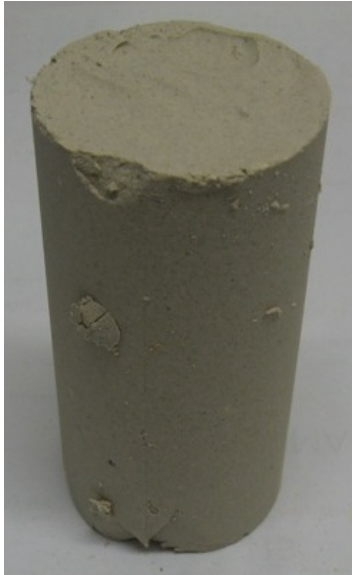
Mix 13. RECON Low Solids Stabilization (LSS) Blend AB: Lime Kiln Dust (LKD), Class C Fly Ash, and Circulating Fluidized Bed (CFB) Fly Ash (25% LKD, 25% CFB, 50% C-ash) – 10%
