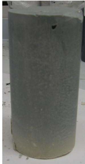
Mix 7. LaFarge MaxCem (70% Joppa Type I/II PC and 30% Slag Cement) – 10%
