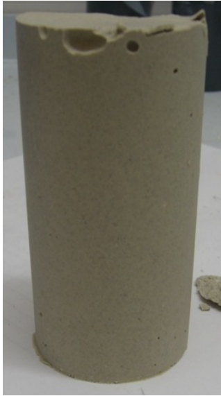
Mix 9. RECON Low Solids Stabilization (LSS) Blend A: Class C Fly Ash and Circulating Fluidized Bed (CFB) Fly Ash (67% C-ash: 33% CFB-ash) – 10%
