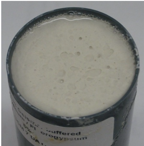
Mix 14. Honeywell Geismar Buffered Crude Gypsum / Fluorogypsum material (CaSO4 Anhydrite) from Hydrofluoric Acid Production – 5%
