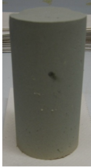
Mix 19. LaFarge MaxCem (70% Joppa Type I/II PC and 30% Slag Cement) – 7.5%
