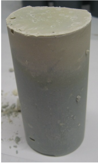
Mix 5. LaFarge NewCem (75%) and LaFarge Type I/II Portland Cement (25%) – 10%
