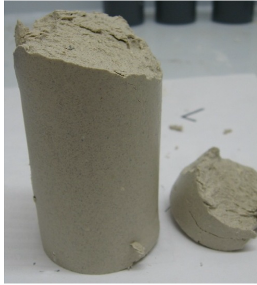
Mix 11. RECON Low Solids Stabilization (LSS) Blend A: Class C Fly Ash and Circulating Fluidized Bed (CFB) Fly Ash (50% C-ash: 50% CFB-ash) – 10%
