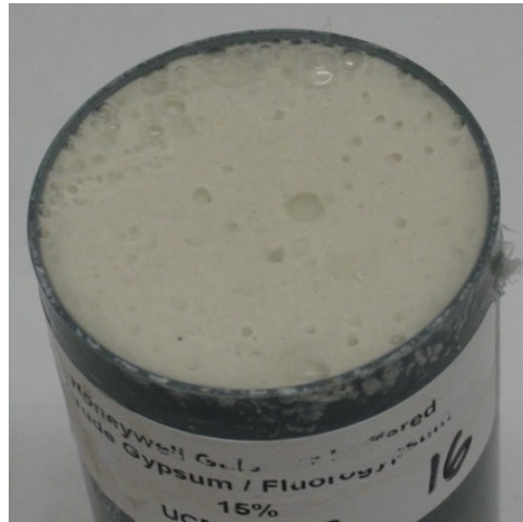
Mix 16. Honeywell Geismar Buffered Crude Gypsum / Fluorogypsum material (CaSO4 Anhydrite), from Hydrofluoric Acid Production – 15%
