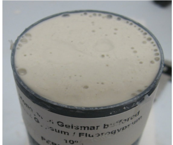
Mix 15. Honeywell Geismar Buffered Crude Gypsum / Fluorogypsum material (CaSO4 Anhydrite), from Hydrofluoric Acid Production – 10%
