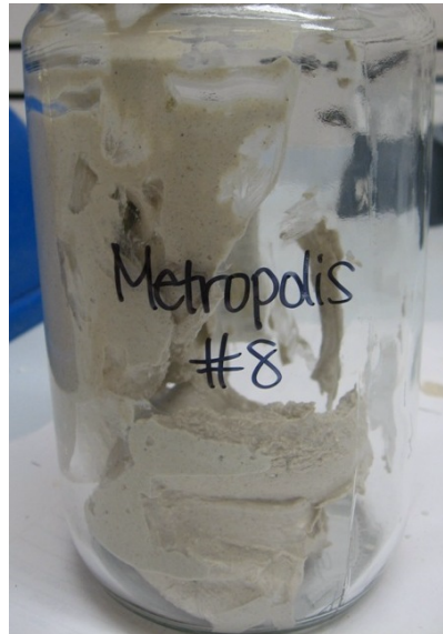
Mix 8. RECON Low Solids Stabilization (LSS) Blend A: Class C Fly Ash and Circulating Fluidized Bed (CFB) Fly Ash (67% C-ash: 33% CFB-ash) – 5%
