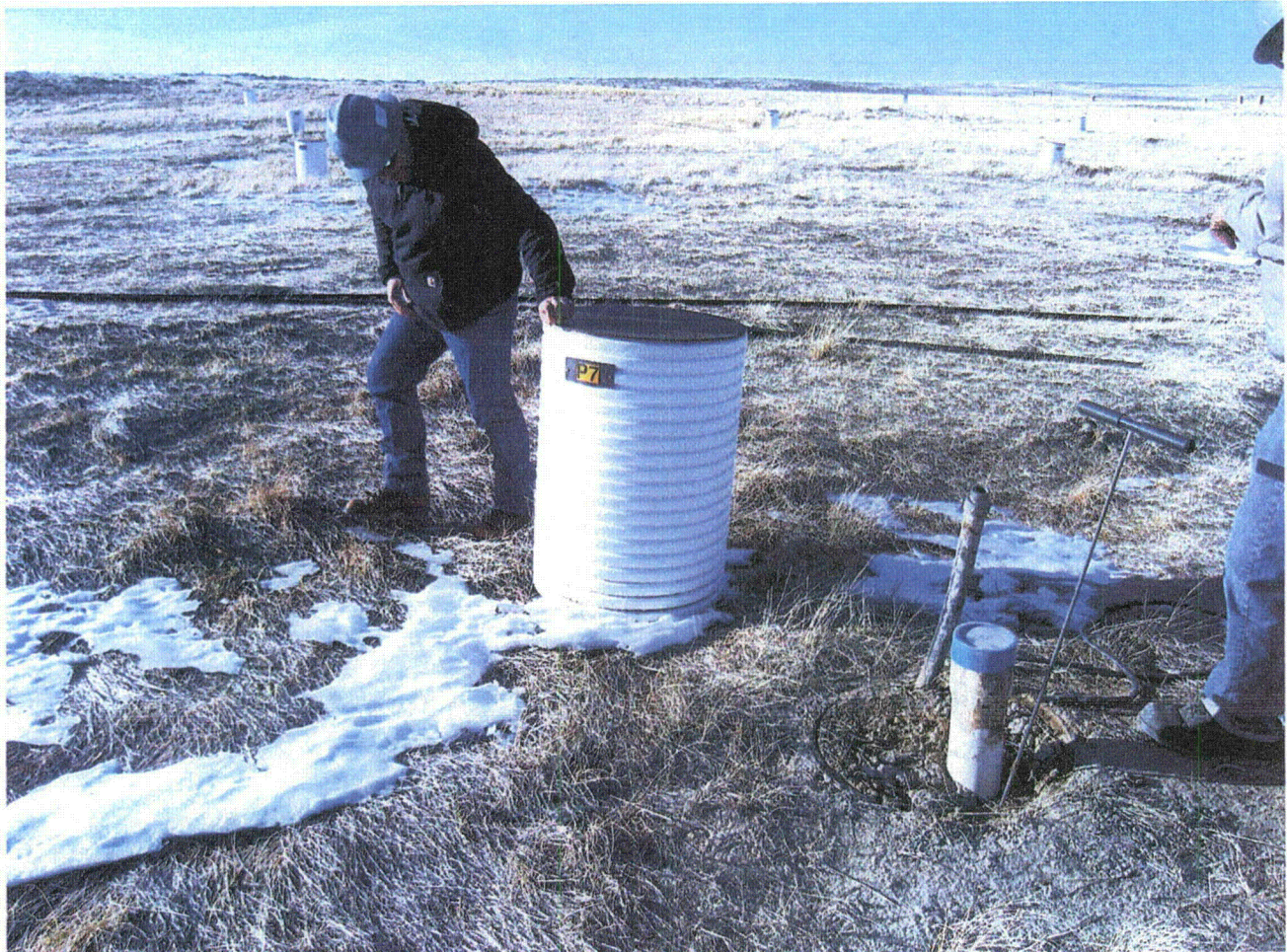
Figure 1 Soil probe inserted and stopped at depth (approximately 3") to concrete seal at repaired well in MU-K
