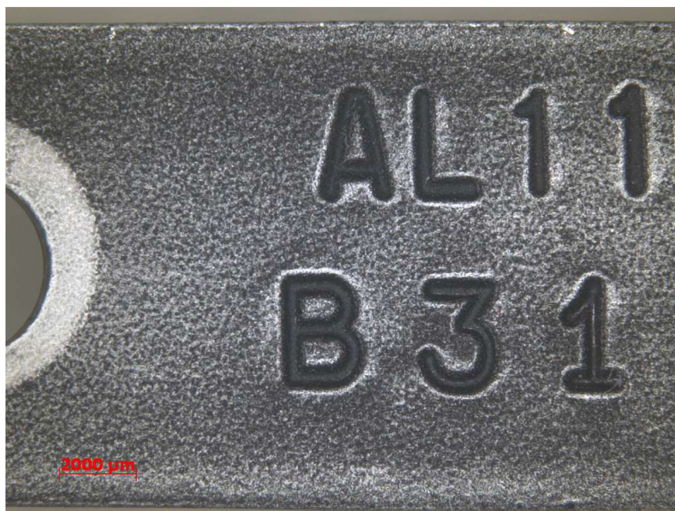
Figure D.2-15 Aluminum Coupon after Cleaning
