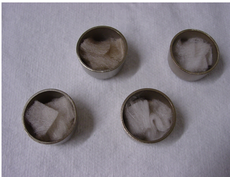
Figure D.2-3 NUKON ® Insulation after Heat at 600°F for 24 Hours
