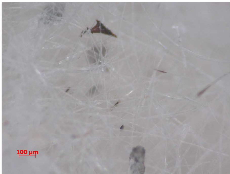
Figure D.2-18 Optical Micrograph of NUKON® Fibers after Test
