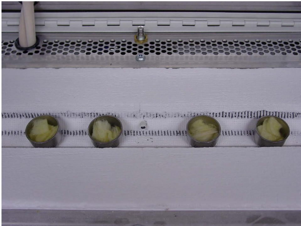
Figure D.2-2 NUKON® Insulation before Heat Treatment
