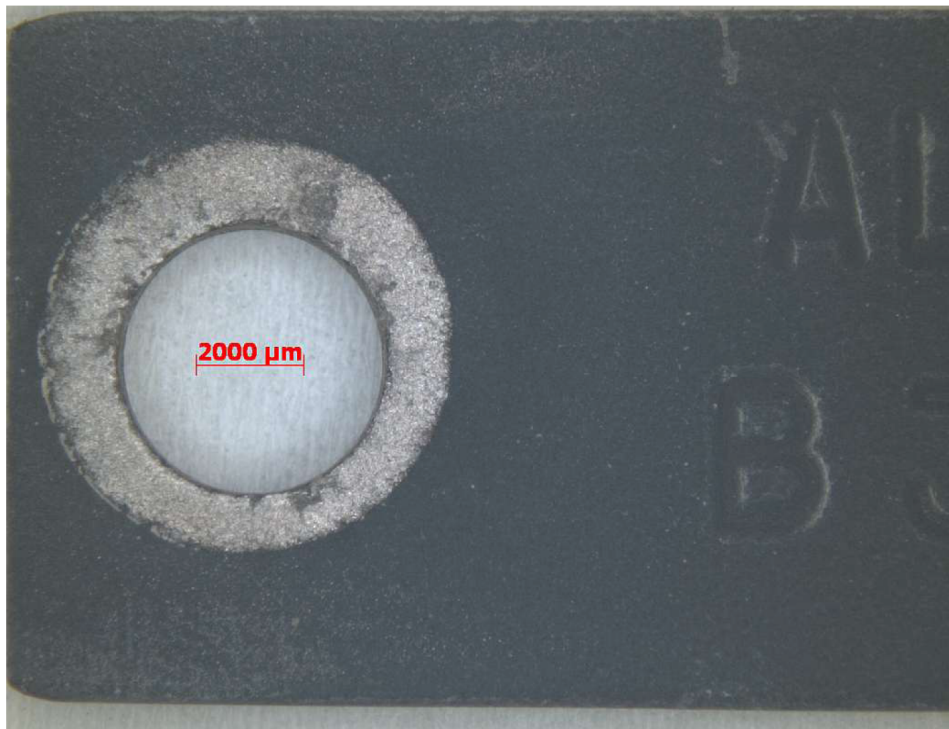
Figure D.2-13 Aluminum Coupon after Removal from Autoclave
