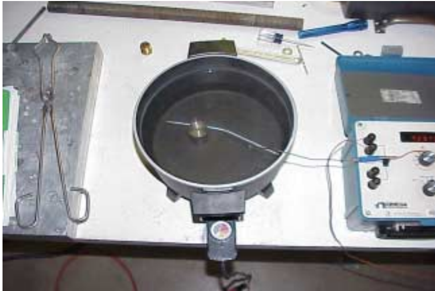
Figure 4-1. Hot liquid bubble test.
