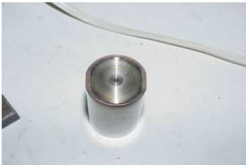
Figure 1-5. Condition of the 3-inch Teletherapy Capsule following the impact test.
