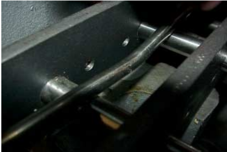
Figure 2-5. Condition of the 8-inch Teletherapy Capsule following the bending (load) test.
