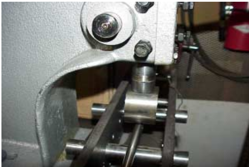
Figure 2-2. Test setup for bending (load).
