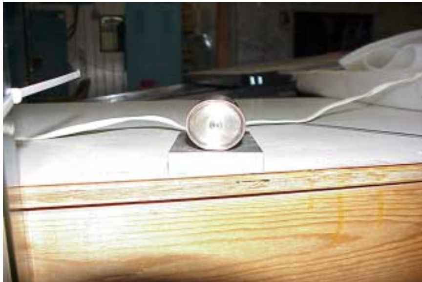
Figure 1-4. Condition of the 3-inch Teletherapy Capsule following the impact test.
