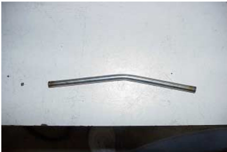
Figure 2-6. Condition of the 8-inch Teletherapy Capsule following the bending (load) test.
