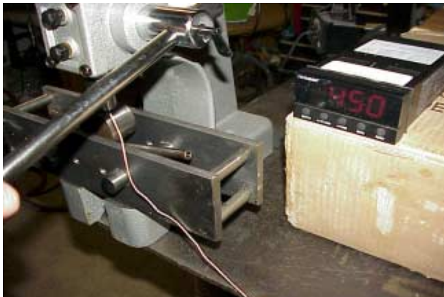
Figure 2-4. Test setup for bending (load).
