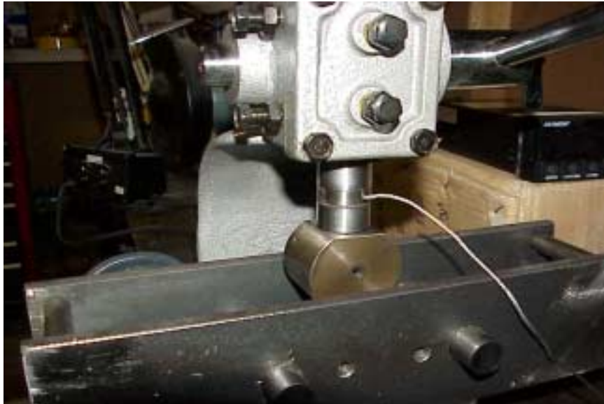
Figure 2-1. Test setup for bending (load).
