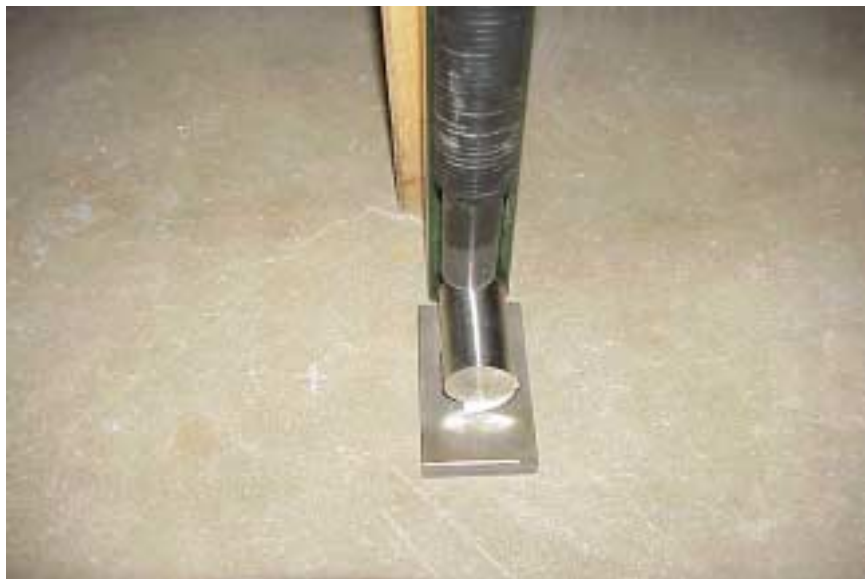
Figure 1-3. Test setup for impact.
