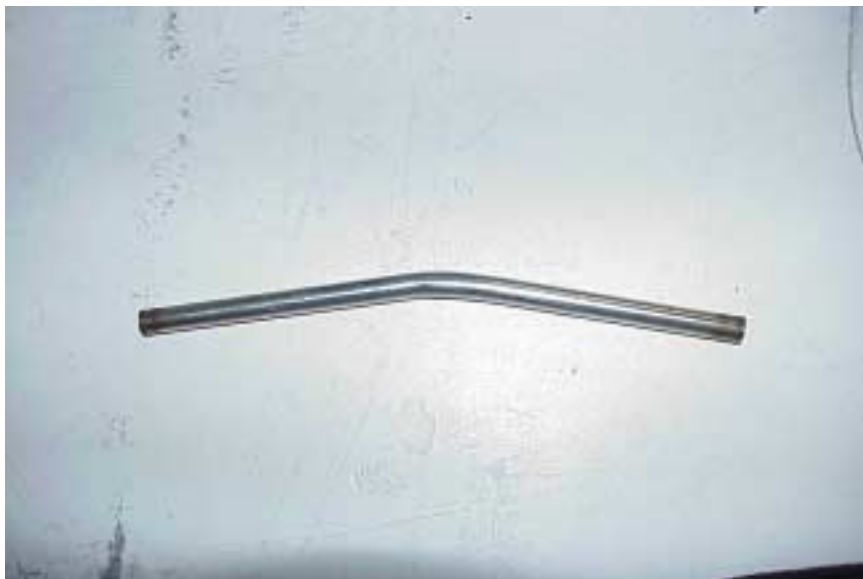
Figure 3-3. Condition of the 8-inch Teletherapy Capsule following the bending (hammer) test.
