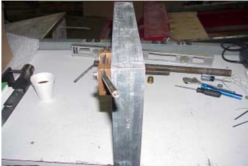
Figure 3-2. Test setup for bending (hammer).
