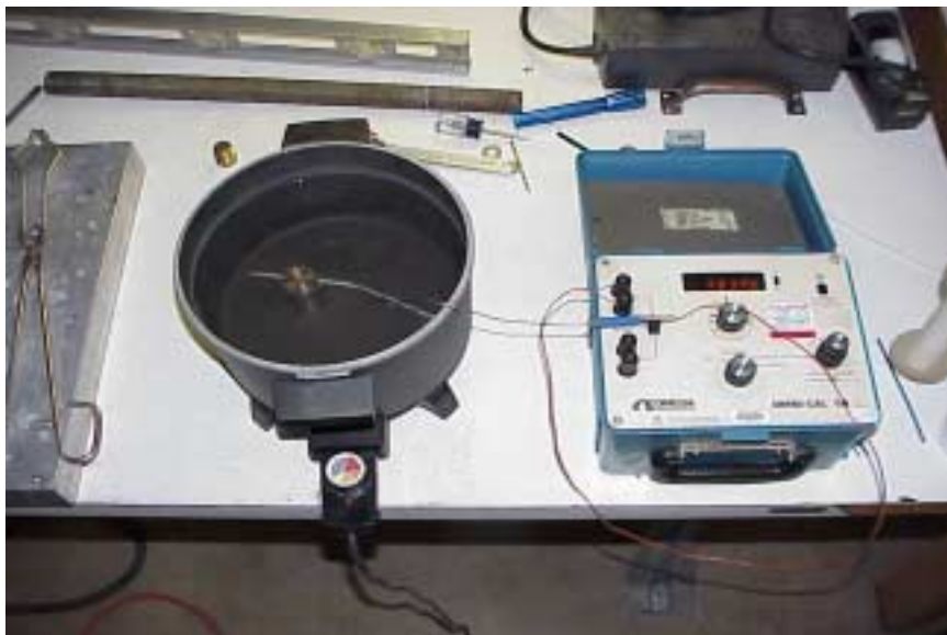
Figure 4-2. Hot liquid bubble test.
