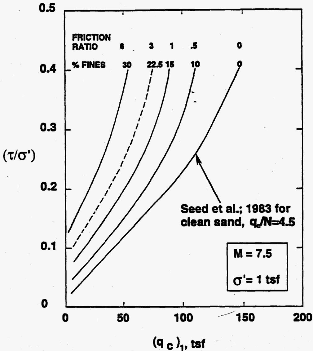
Figure 7-11 Cyclic Stress Ratio versus Cone Penetration Tip Resistance
