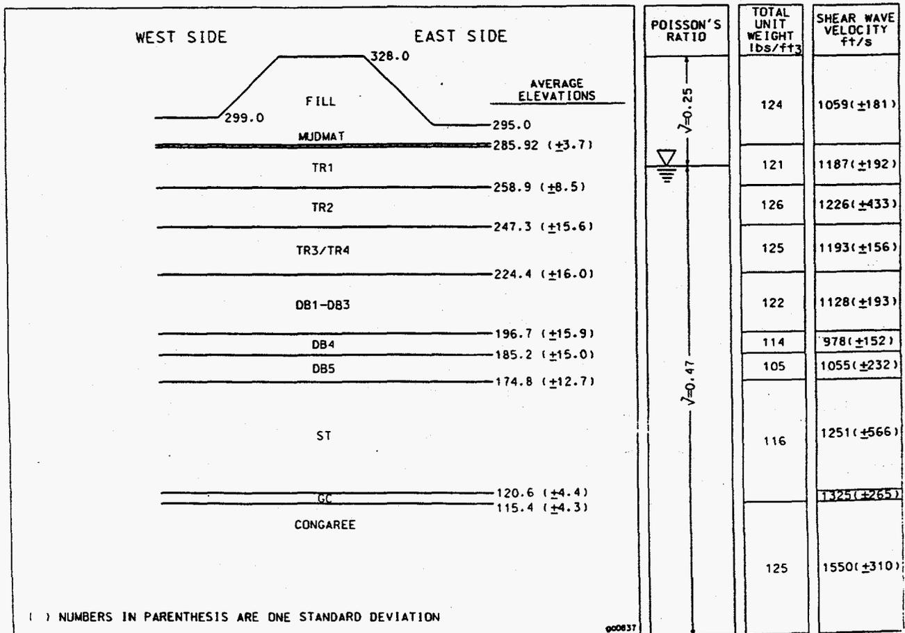
Figure 6-1 Idealized Cross Section Showing Mean Shear Wave Velocities, Poisson's Ratios, and Unit Weights for Each Formation.
