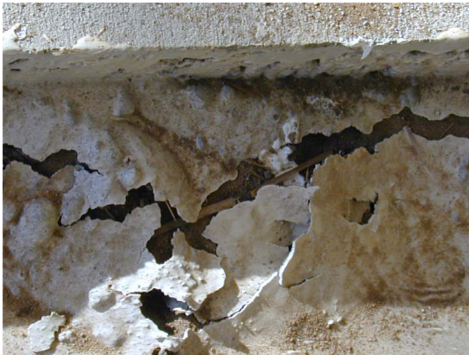
Figure 11. EKOR™ “geopolymer” coating demo at SRS (low tensile strength and self-tearing during curing in absence of applied stress)
