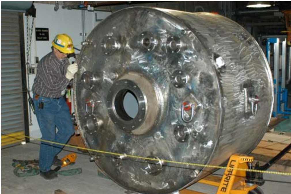
Figure 13. Stainless steel high activity drain (HAD) tank lined with vinyl ester (vinyl ester protects stainless steel from halide attack)
