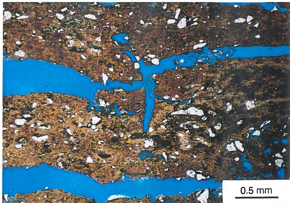
Figure 31. Photomicrograph of Quartz-Rich Terrigenous Mud, Terrigenous Mud Microfacies, Aquifer Unit IIB 1 , General Separations Area, SRS. Well HPC-1, 144 ft. Sample disrupted during thin-section preparation. Plane-polarized light.
