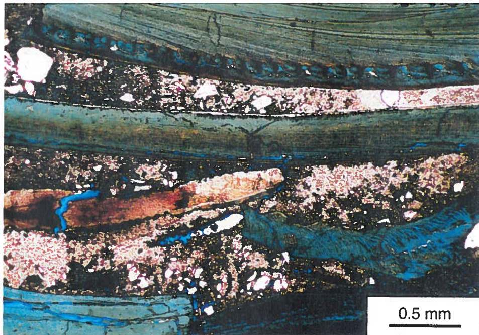
Figure 16. Photomicrograph of Sandy, Skeletal Siliceous Mudstone, Siliceous Mudstone Microfacies, Confining Unit IIA-IIB, General Separations Area, SRS. Opal cement is light brown. Well BGO-9AA, 150 ft. (thin section BGO-9AA-150B). Plane-polarized light.
