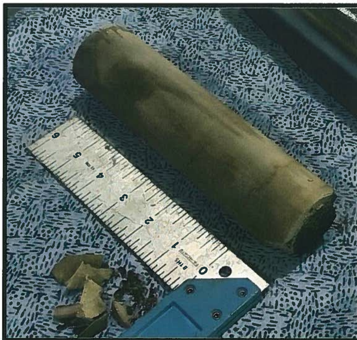
Figure 8, Fast Pour Formed-Core Sample. Note: Arbor Press Used to Remove Core.
