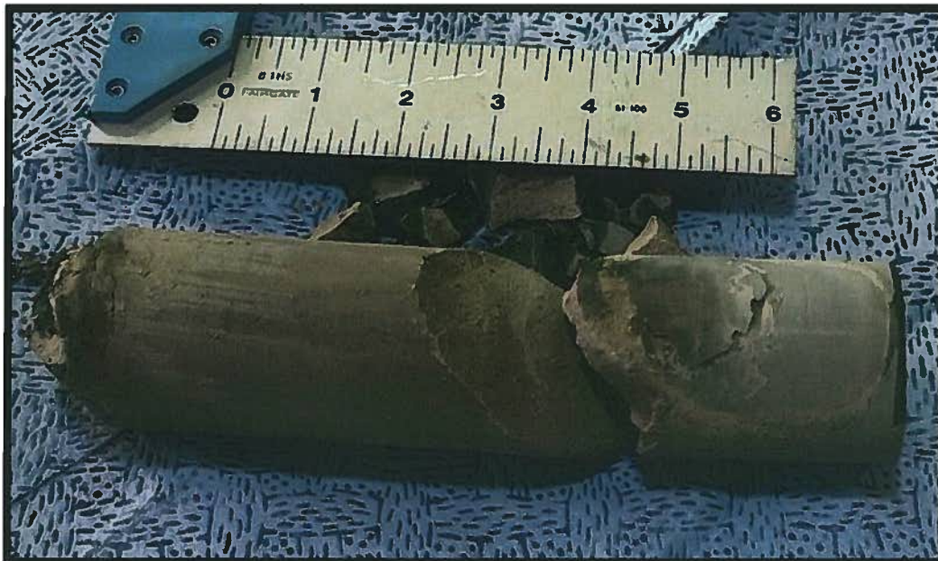
Figure 7, Slow Pour Formed-Core Sample. Note: Core Split Most Likely Due to Failure of Screw Jack Adapter.
