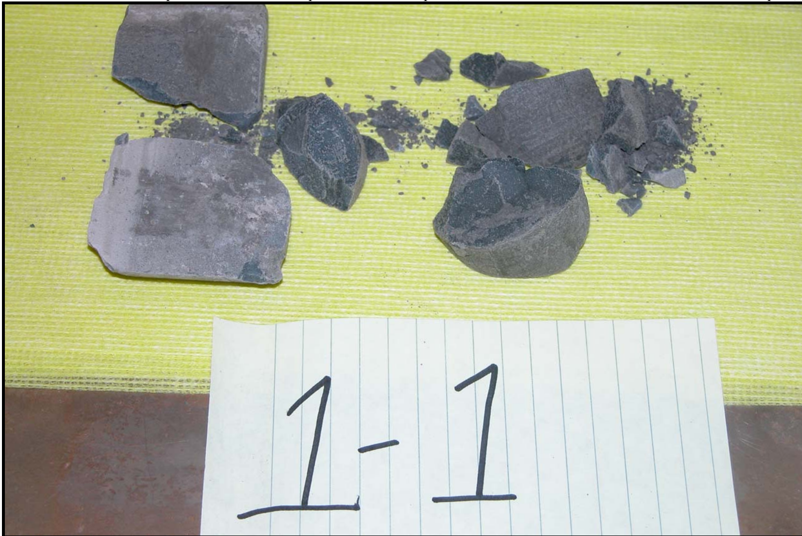
Figure 4 Sample 1-1, No Solid Cylindrical Pieces
