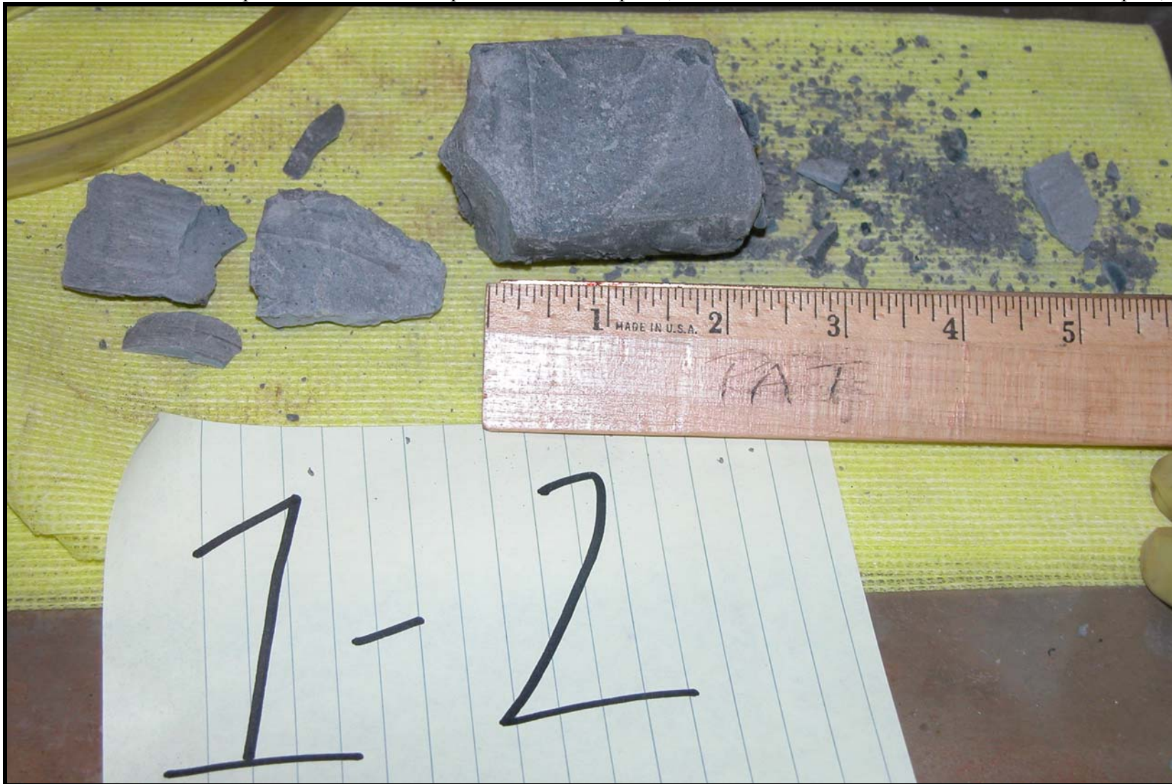
Figure 5 Sample 1-2, No Solid Cylindrical Pieces
