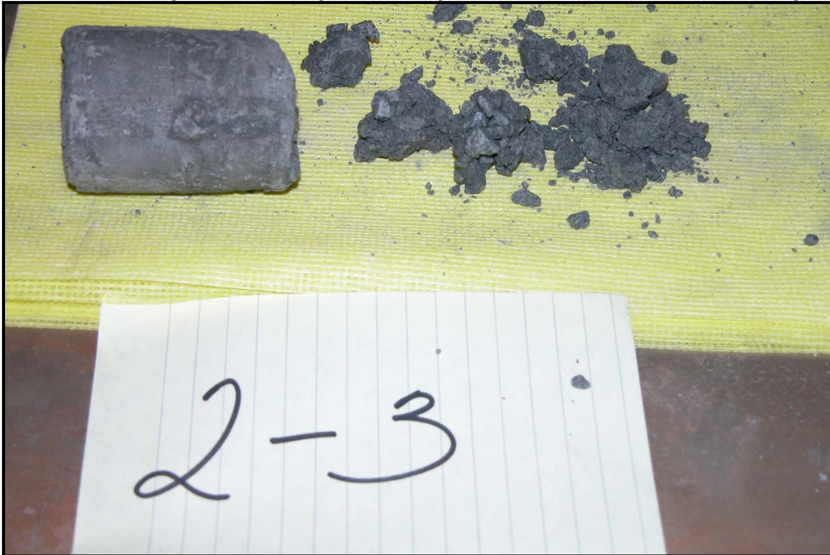
Figure 9 Sample 2-3, 2" Long Solid Cylindrical Piece (Piece on left) and Crumbly Pieces
