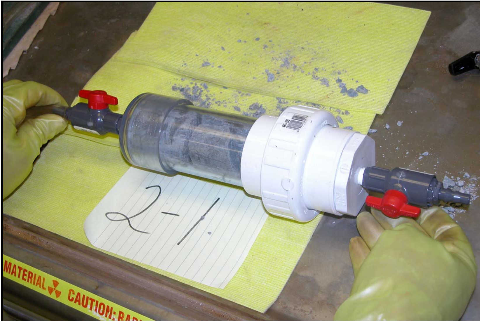
Figure 3 Typical Transparent PVC Holder in the Process of Being Purged with Nitrogen Gas Prior to Isolating the Sample
