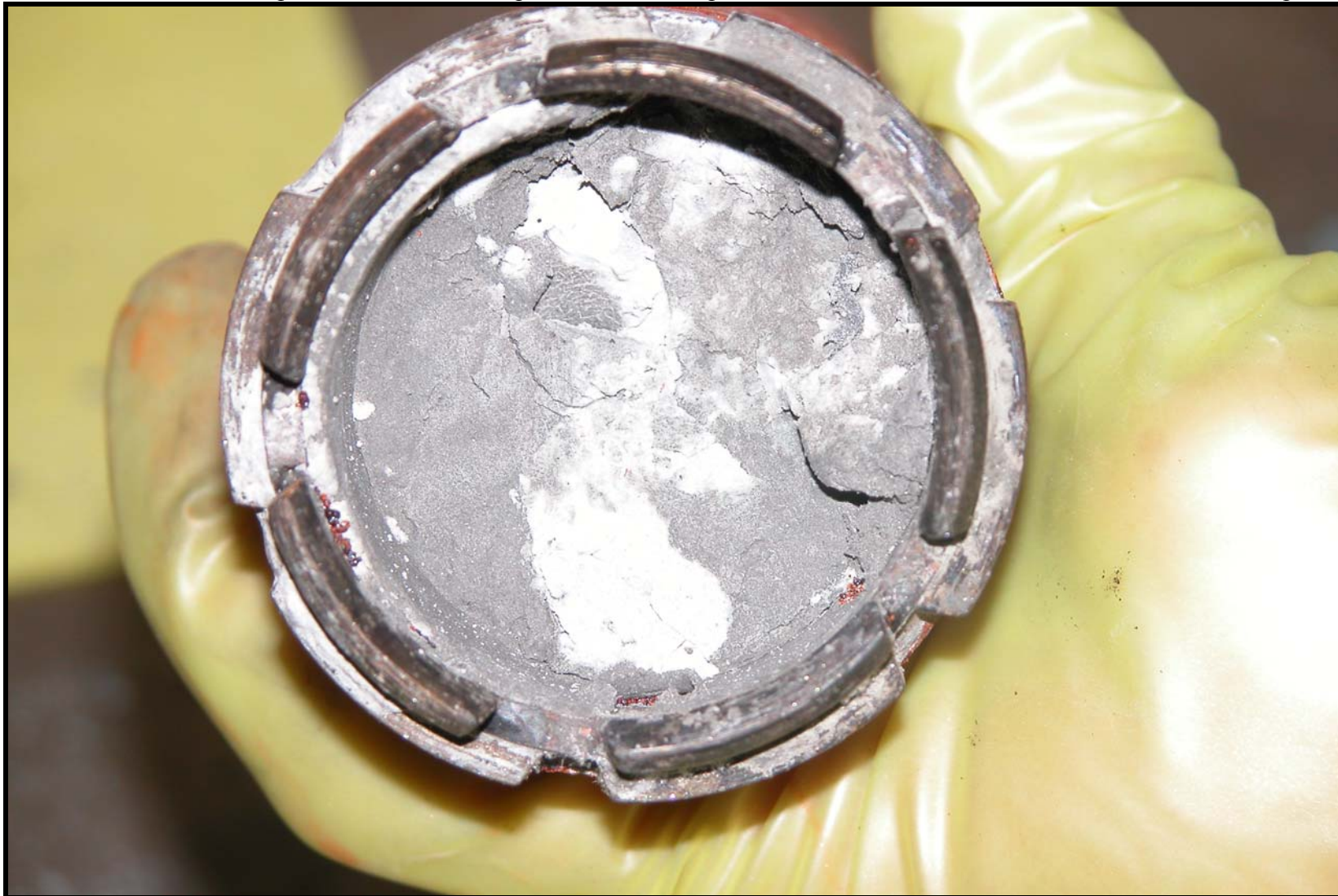
Figure 15 First of the Two Core Bit Samples – Sample Jammed in Bit
