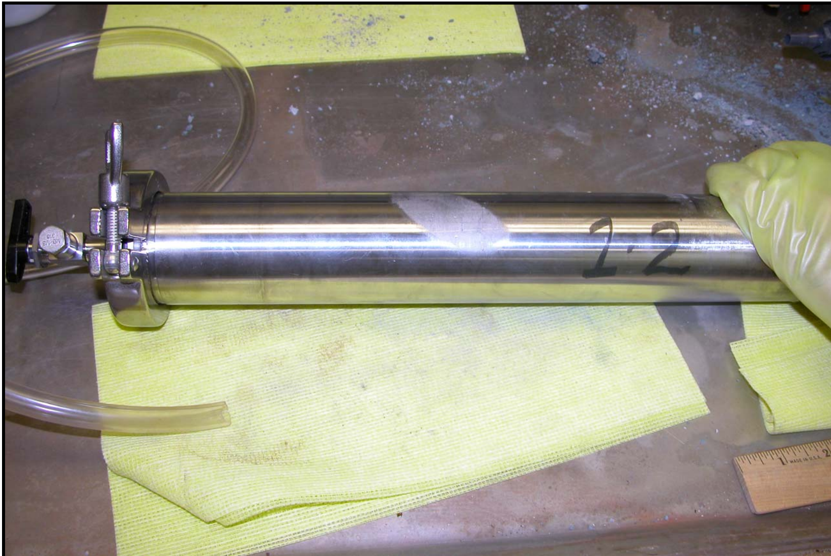
Figure 2 Original Typical Stainless Steel Vault 4 Sample Container – Vent on left side of container
