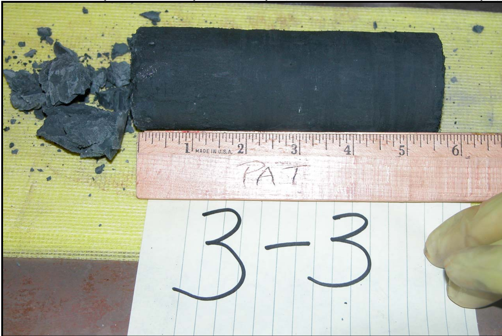
Figure 13 Sample 3-3, 5.5" Long Solid Cylindrical Piece (on Right) and Crumbs
