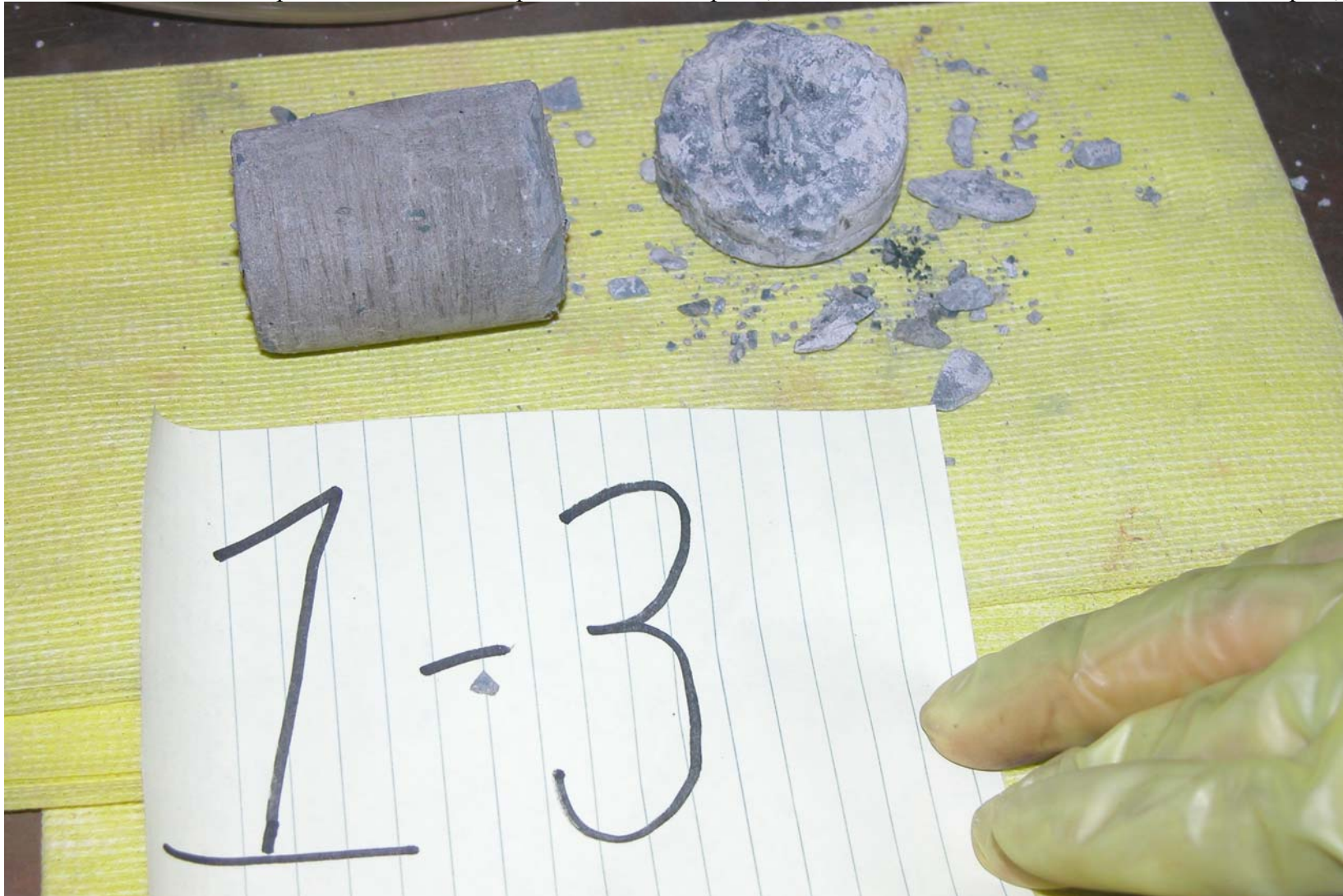
Figure 6 Sample 1-3, No Solid Cylindrical Pieces were Present – Looks Cylindrical, but is not
