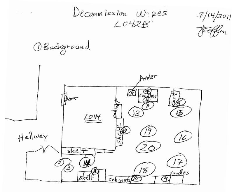
Meter Readings Ludlan 3, Sen#142357 Cal: 10/12/10 Probe: 44-9, PR145855 Background: 20-70 CPMS Readings: Background
