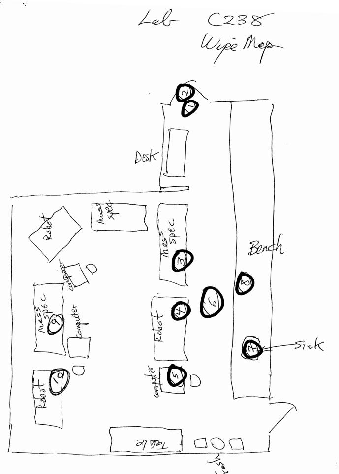
7/13/05 Decommission C238 Hallway Tim Coffin Lab 1350 The Sealed Hoor Monitoring udlymdel 2221 Set 206842 Bench Monitoring Ludlum 3, 99436 Probe 44-3 Background: 400-600 counts Ludlum 3, 211698, Probe 44-9 Background: 0.03 ont reading : 1386 Readings : 0.03 D cleaned to: 863
