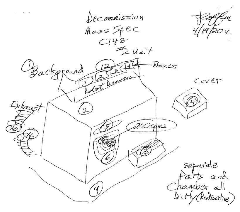
Meter Ludlum 3 == 242761 Cel ; 4/12/11 Probe: 44-9, 1R 257040 Background: 40-80 cpms Readings: Beckground (Except Beckof Chamber 9 Parts
