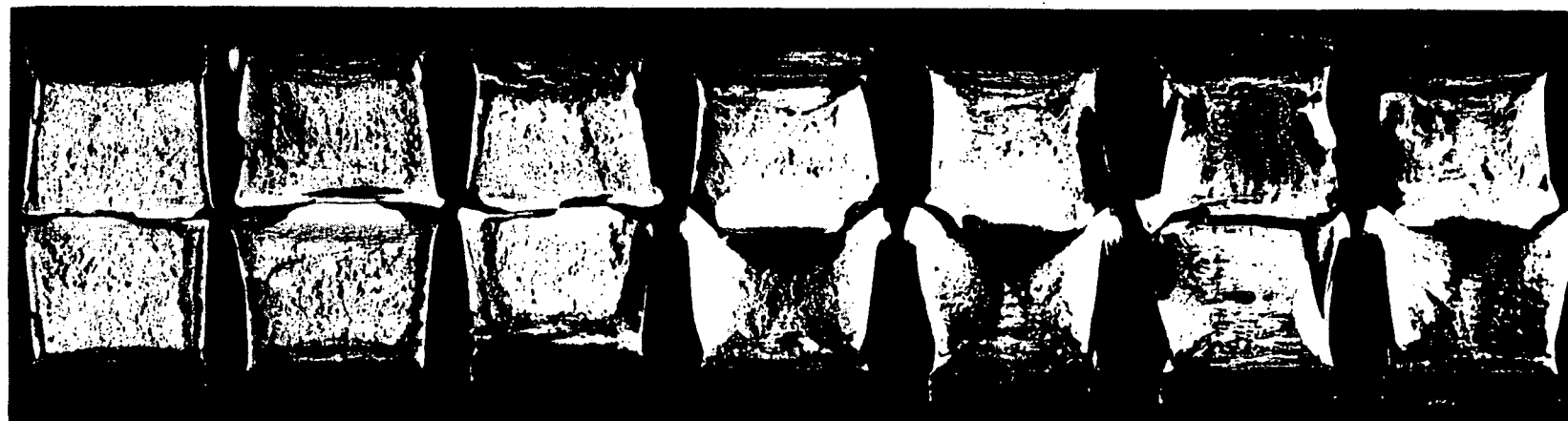
FIGURE 22. CHARPY IMPACT SPECIMEN FRACTURE SURFACES FOR THE IRRADIATED WELD METAL SPECIMENS FROM THE MONTICELLO 30 DEGREE SURVEILLANCE CAPSULE
