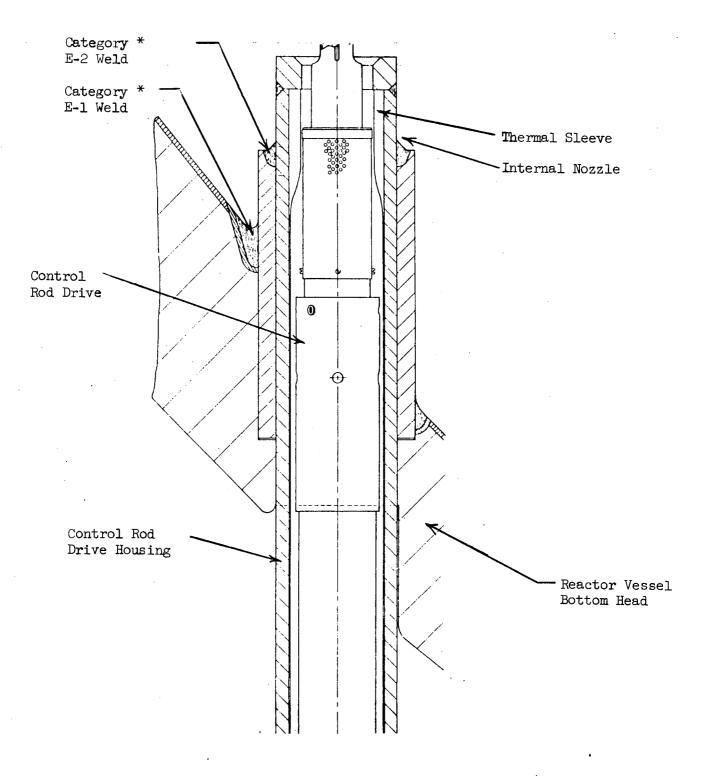
Figure 1 CRD Housing Welds
