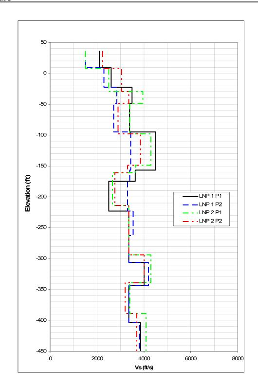
Note: Profiles LNP 1 P1 and LNP 2 P1 are based on suspension logging data Profiles LNP 1 P2 and LNP 2 P2 are based on downhole data Progress Energy Florida
