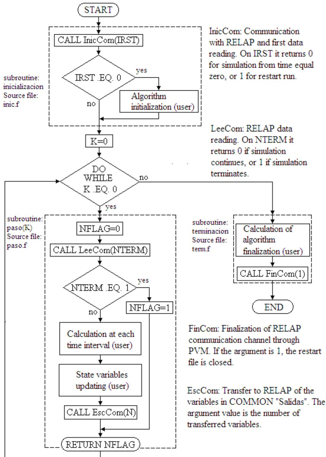
**Fig. 1 -.** Flow chart of the external control program.
