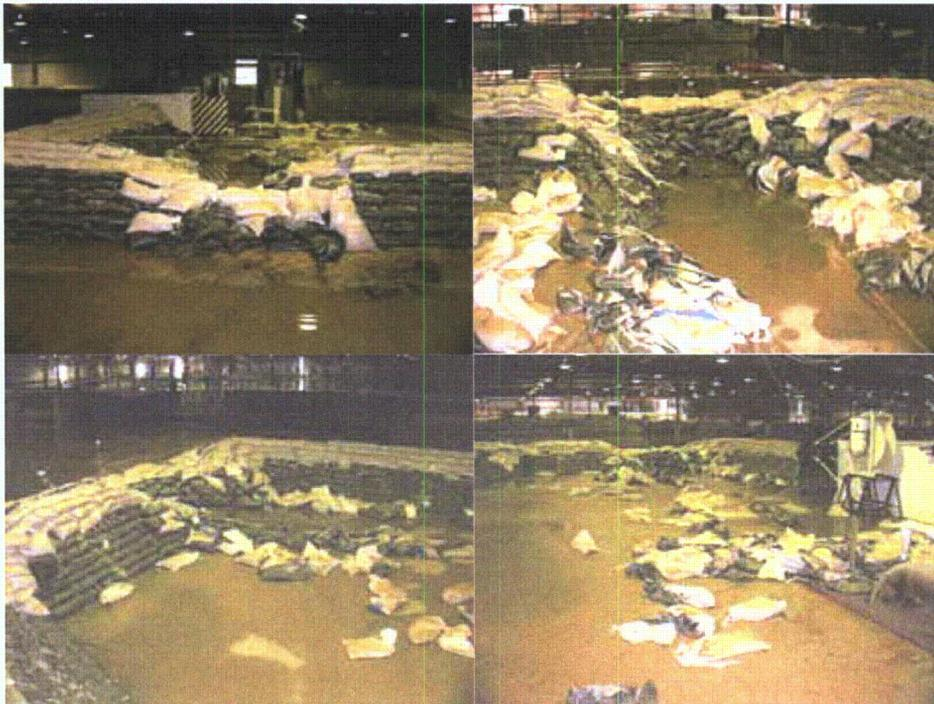
Figure 2-39. Sandbag levee after failure
