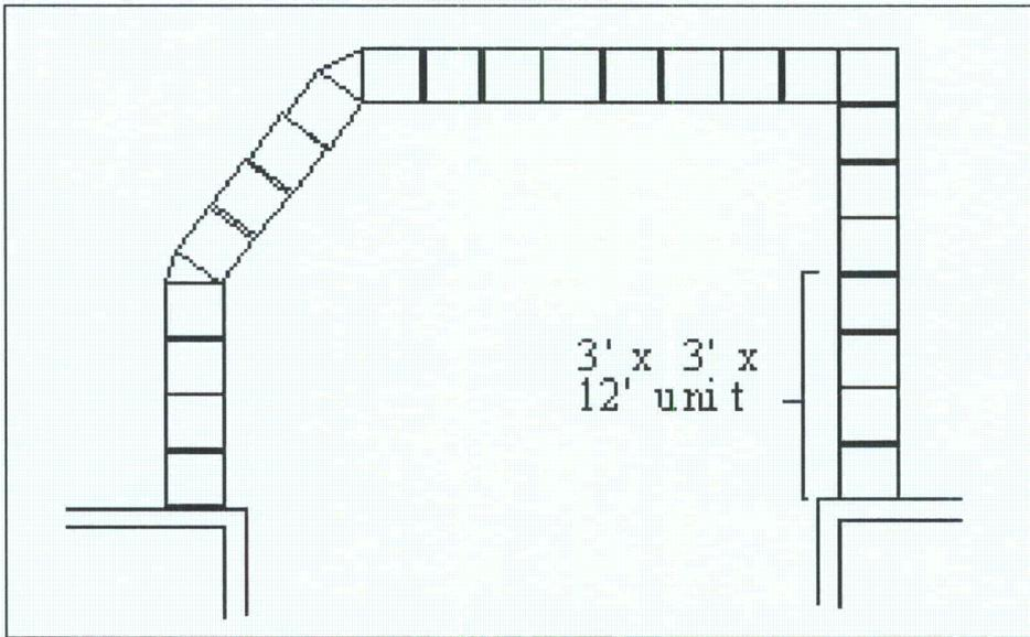
Figure 2-45. Hesco® levee layout
