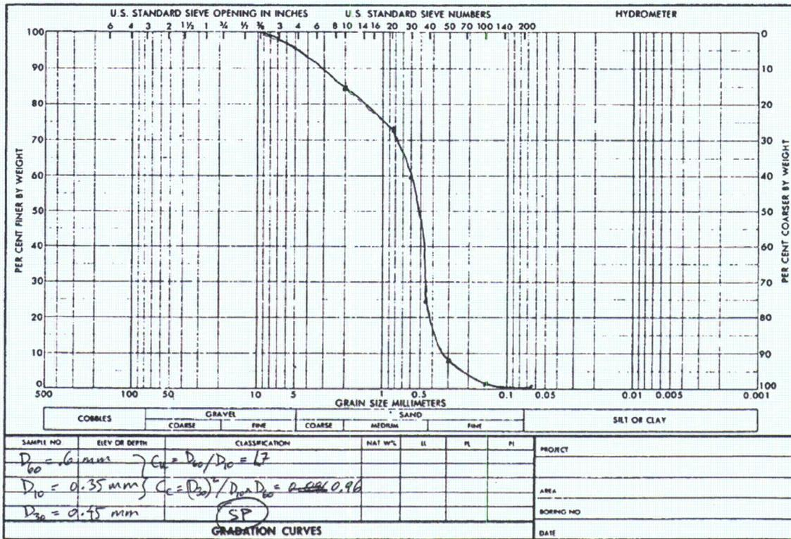
Figure 2-20. Gradation of sand used for filling sandbags
