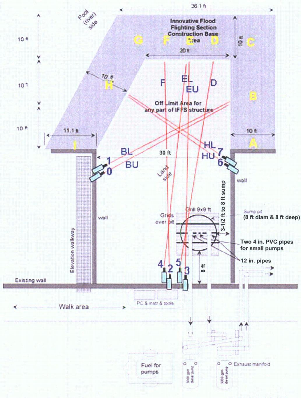
Figure 2-7a. Lasers and their targets on levee
