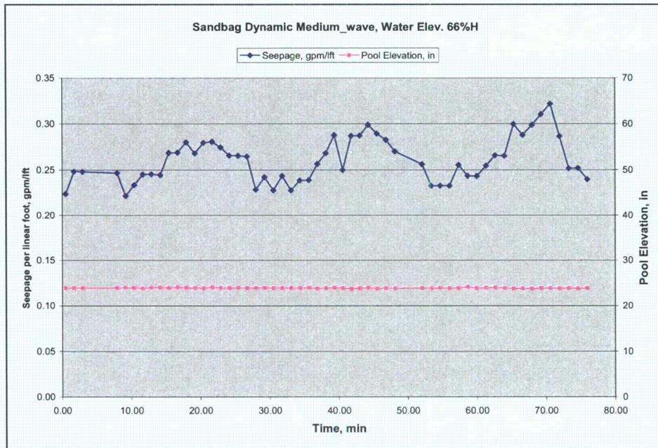
Figure 2-30. Seepage with dynamic testing at 66 percent levee height and 7- to 9-in. waves
