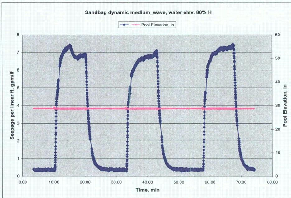
Figure 2-33. Seepage with dynamic testing at 80 percent levee height and 7- to 9-in. waves
