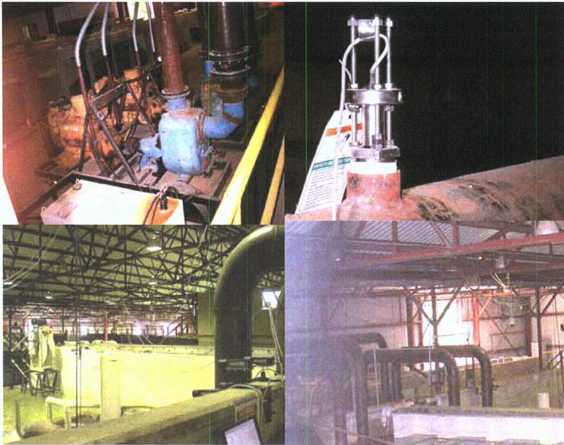
Figure 2-3. Pumping system used for overtopping, 12 in. diam. Top left: diesel pumps. Top right: flow meter. Bottom left: pipes leaving basin to pumps. Bottom right: pipes from basin to pumps and back to basin
