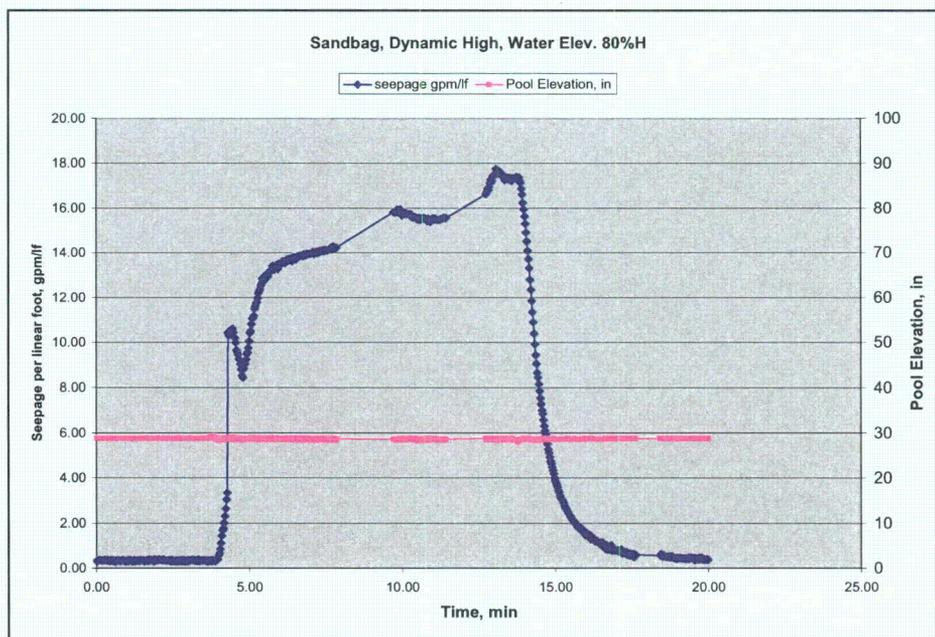
Figure 2-34. Seepage with dynamic testing at 80 percent levee height and 10- to 13-in. waves
