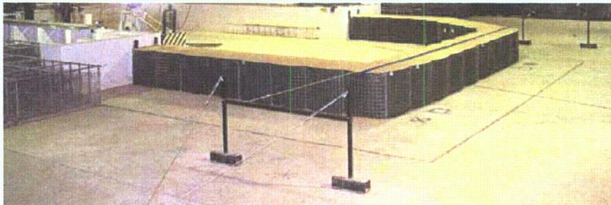
Figure 2-61. Center wall displacement monitoring system
