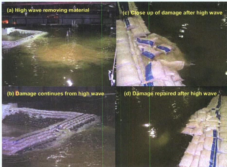
Figure 2-41. Sandbag levee damage and levee after field repair 1
