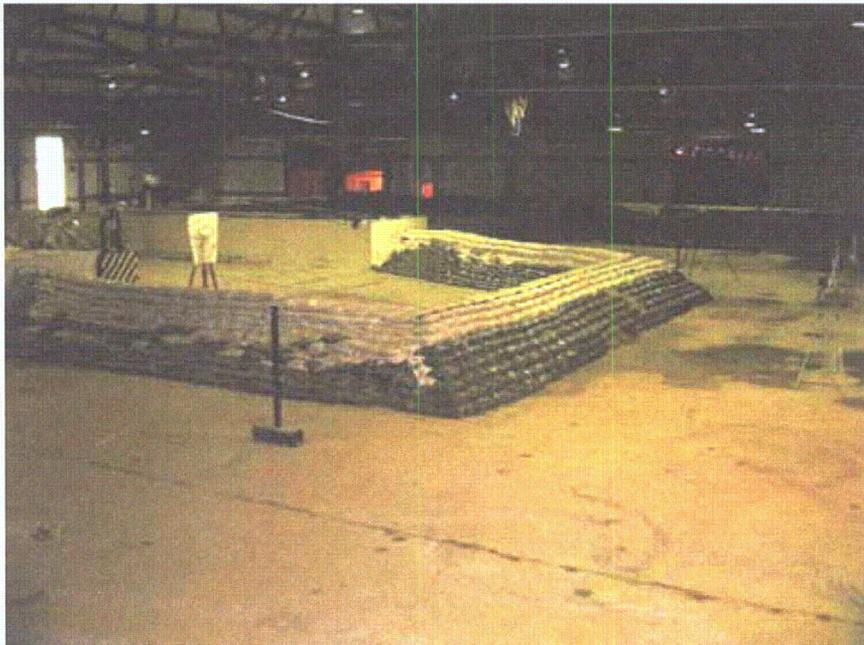
Figure 2-28. Sandbag levee after repair
