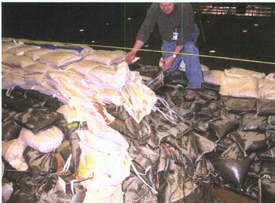
Figure 2-40. Sandbag levee autopsy after overtopping
