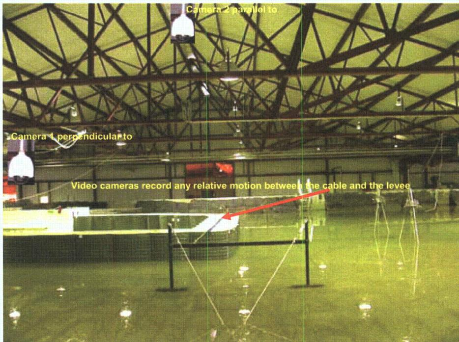
Figure 2-8. Relative movement and video monitoring system
