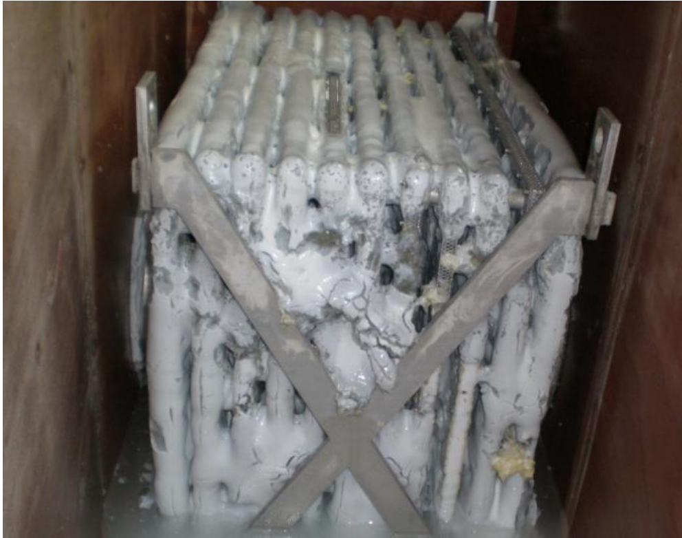
Figure 2: Photograph showing WCAP-16530-NP chemical surrogate following a head-loss test for STP
