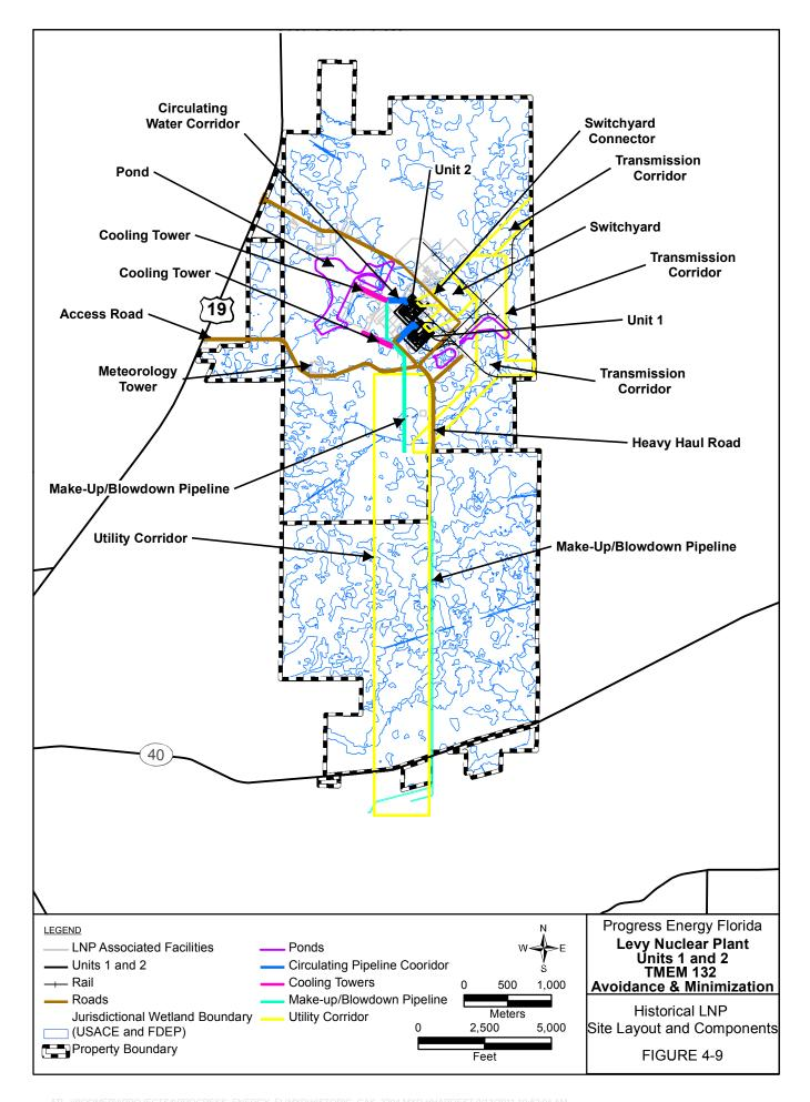
Four stormwater ponds (A, B, C, and D) were originally proposed to manage stormwater drainage, and to maintain or exceed historic floodplain storage on the LNP site. The ponds were designed based on the SWFWMD *Basis of Review, Part B*. Two of the ponds were combined and reconfigured to avoid wetlands. Pond D was reduced in size to avoid wetlands. The stormwater ponds are elevated and shallow, which reduces the potential for groundwater drawdown in adjacent wetlands.
