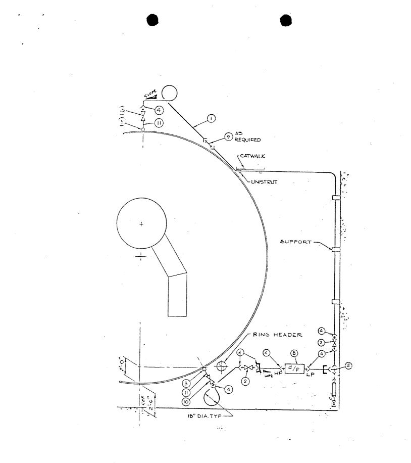
Figure 2 Containment Water Level Monitors
