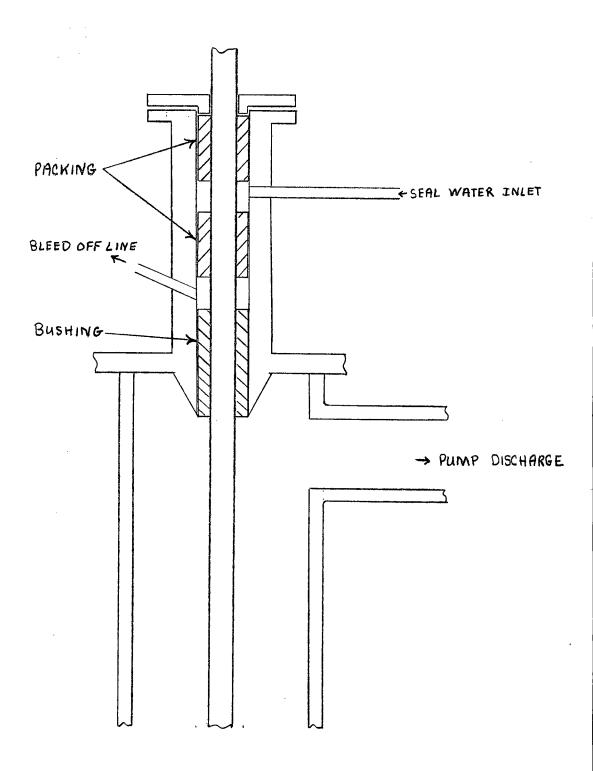
RHR SERVICE WATER PUMP SEAL WATER ARRANGEMENT
