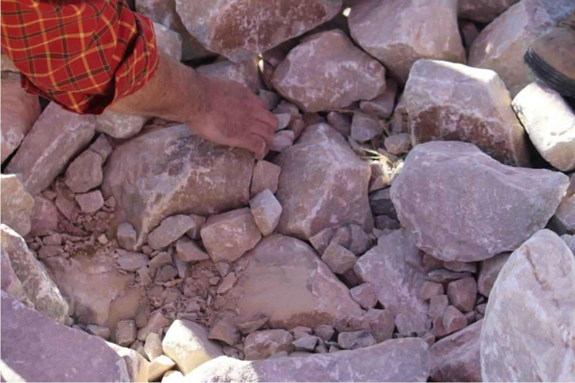
Visual inspection of bedding layer material under Type C rock
