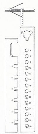
FIG. 4 Calibration Bars for Caliper Probes (3)
