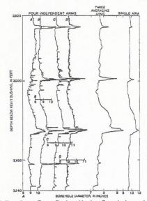
FIG. 3 Caliper Logs From Probes Having Four Independent Arms, Three Averaging Arms, and a Single Arm, Madison Limestone Test Well 1, Wyoming (2)
