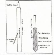
FIG. 1 Probe for Making Side-Collimated Gamma-Gamma Logs with Single-Arm Caliper (2)
