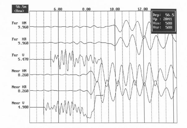
Figure 2. Sample suspension method waveform data showing horizontal normal and reversed (HR and HN), and vertical (V) waveforms received at the near (bottom 3 channels) and far (top 3 channels) geophones. The arrivals in milliseconds for each pick are shown on the left. The box in the upper right corner shows the depth in the borehole and the velocities calculated based on the picks.
