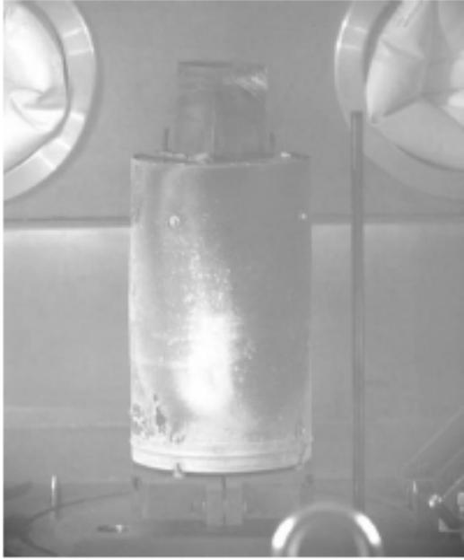
**Figure 14: Corrosion on the heating element**
