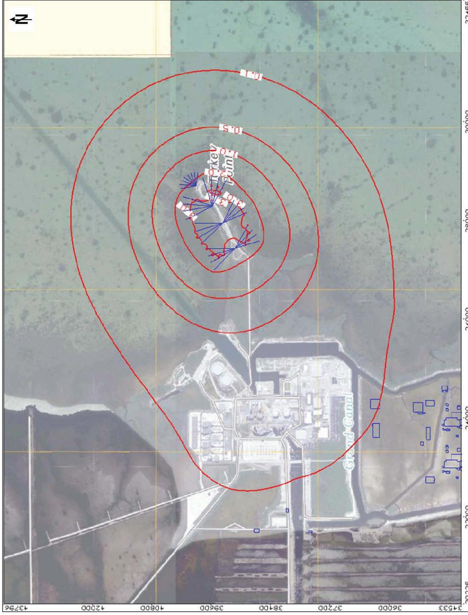
Note: Thin red line = 0.1, 0.5, 1.0, 2.0, and 3.0 foot drawdown contours. Light yellow portion in top right is where aerial imagery is not available. Approximate elevation of Upper Higher Flow Zone underneath Turkey Point Peninsula is -22 ft NAVD 88.
