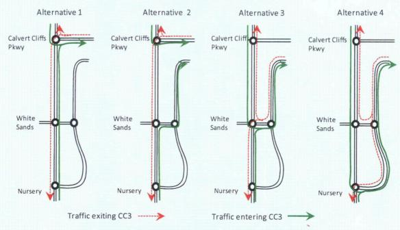
Figure 5 – Illustration of CC3 Access Alternatives
