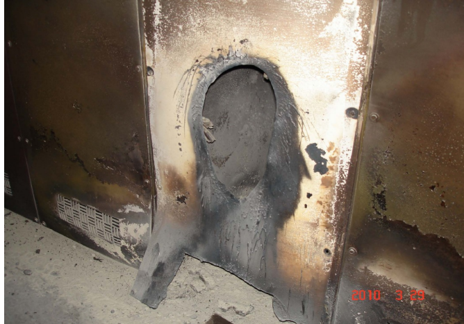
Figure 8: Impact of HEAF event on the switchgear cabinet
