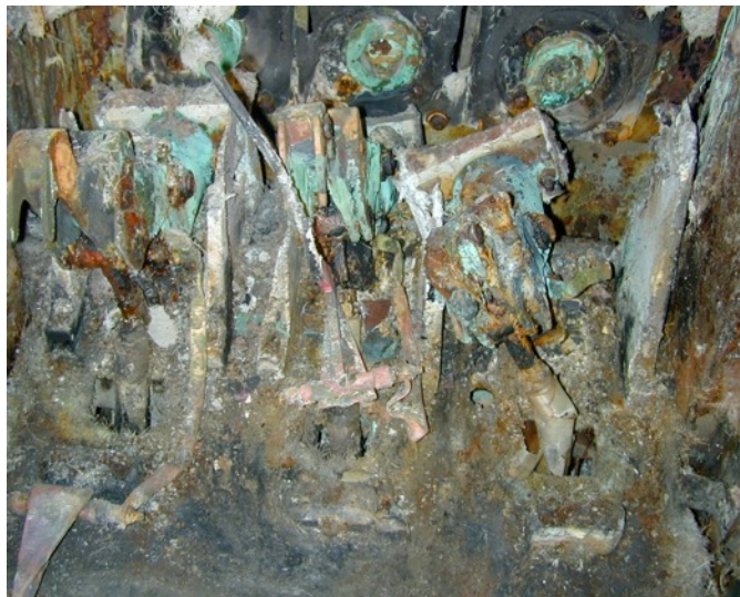
Figure 9: Internal view of a HEAF incident along the posts
