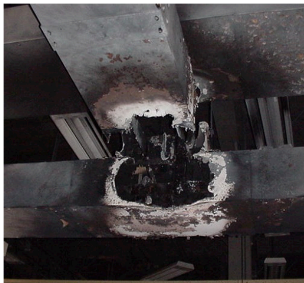
Figure 3: HEAF inside cable duct
