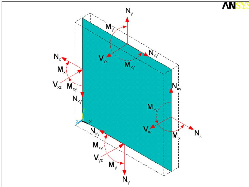
Figure 8.1-1 Force and Moment Demands for Design of SC Walls
