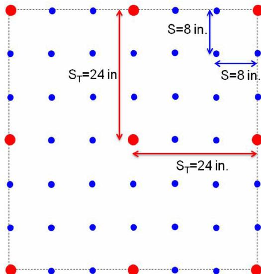
**Figure 2.1-1 Stud and Tie Bar Grid Pattern on Steel Faceplates**
