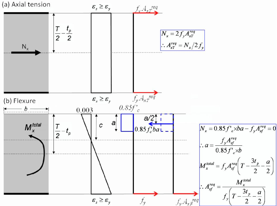
Figure 8.2-1 Section Equilibrium Used to Compute Steel Areas when  $N_x$ ,  $N_y$  in Tension
