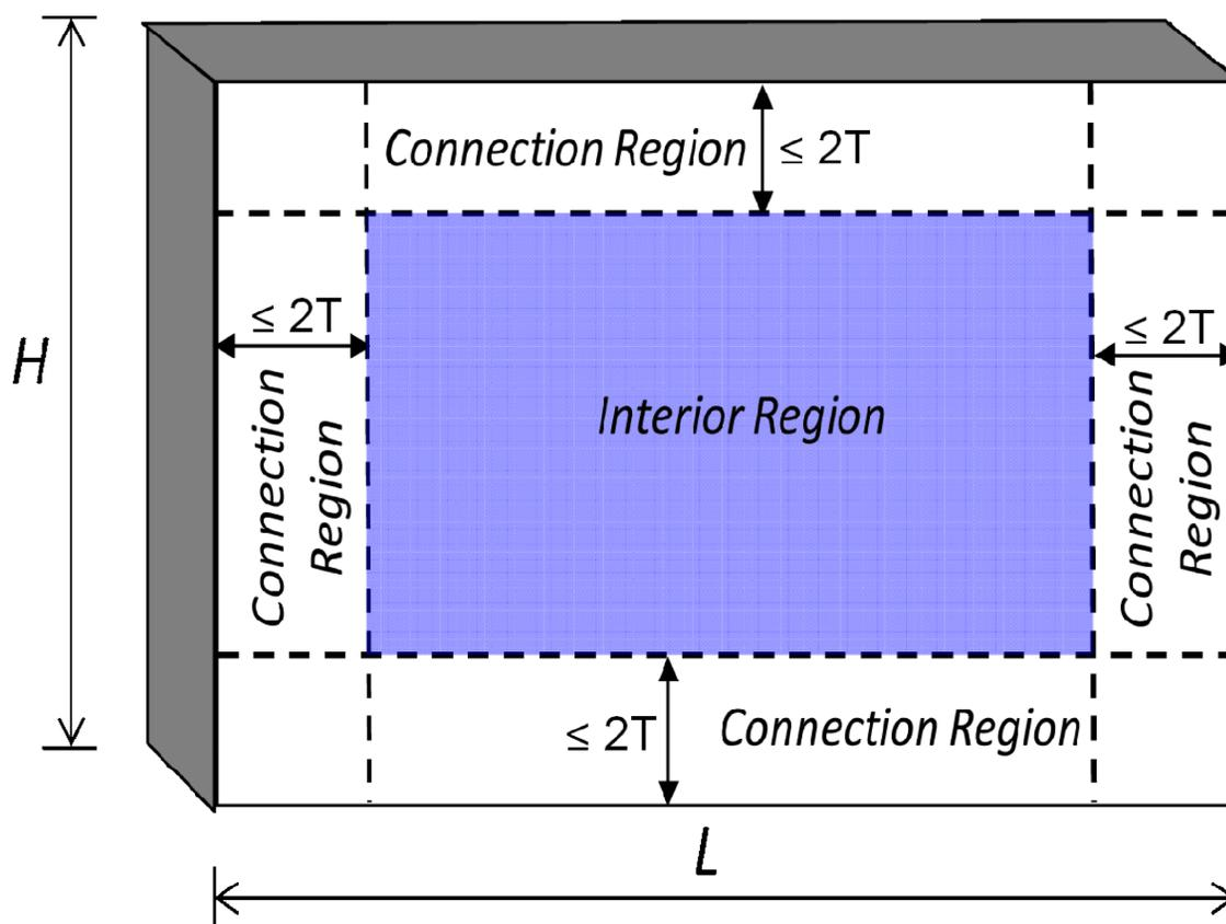
Figure 1.2-1 Interior and Connection Regions for SC Walls
