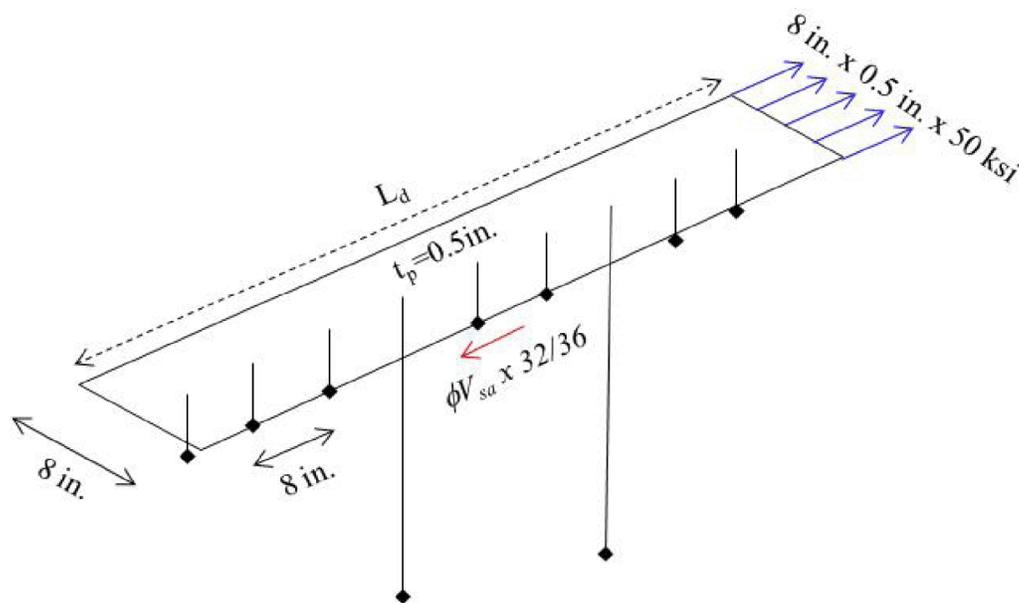
**Figure 2.4-1 Free Body Diagram for Calculating Development Length**
