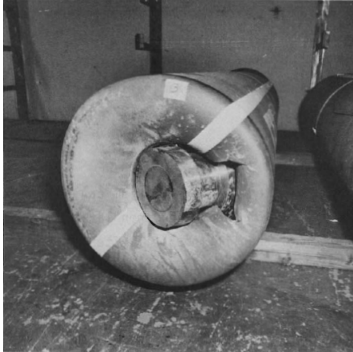
Figure 7-4. Asymmetric Deformation of Titanium Canister Showing Rupture at the Nozzle. Top Drop Event From a Height of 9 m [30 ft] (Peterson, et al., 1985)
