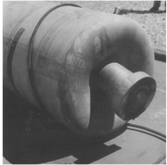
Figure 7-8. End Deformation of Stainless Steel Test Canister Subjected to a Top Drop With Center of Gravity in Line With Canister Shoulder (Olson and Alzheimer, 1989)
