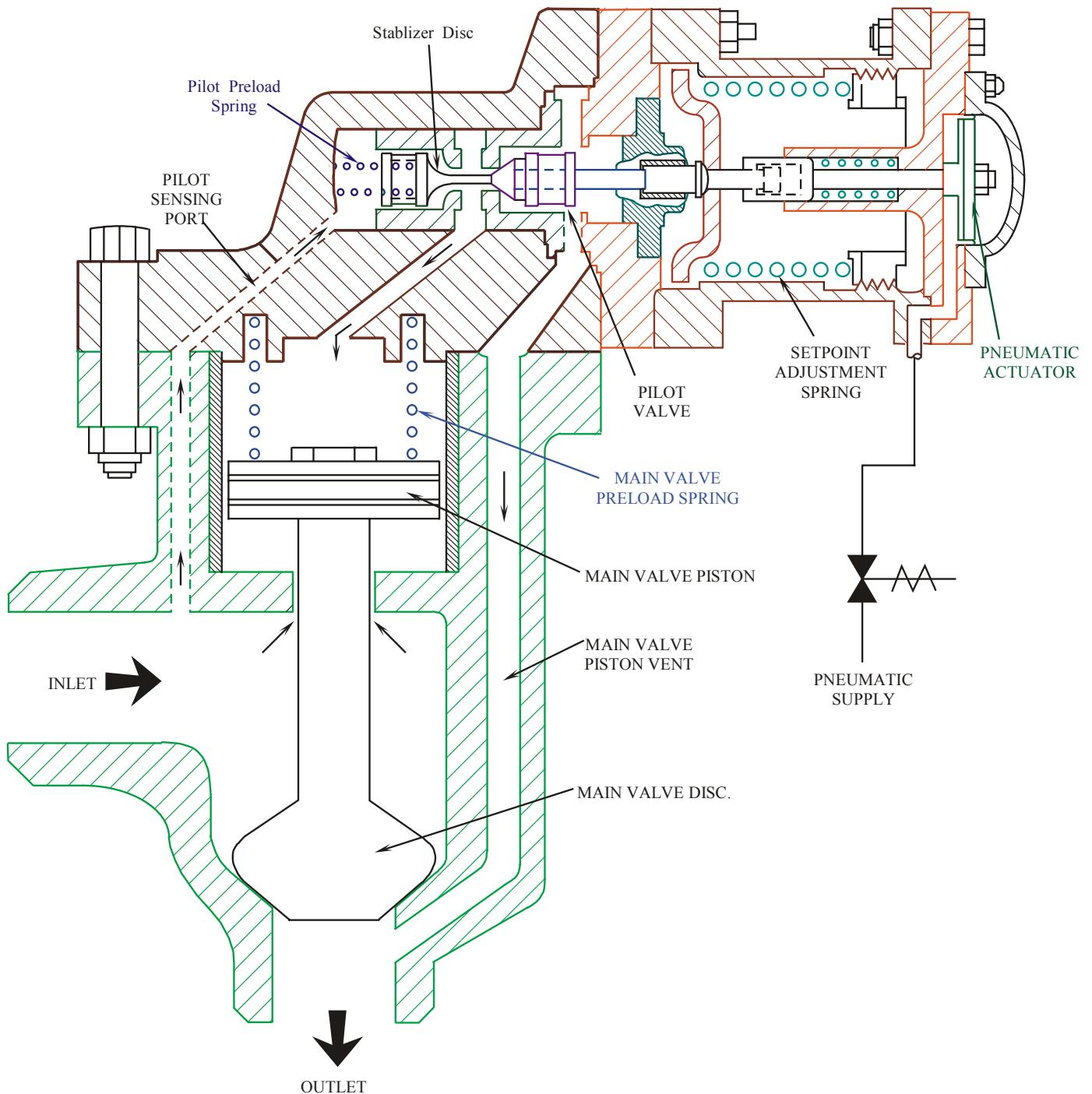
Figure 6.8-1 Two Stage Target Rock SRV (Closed)
