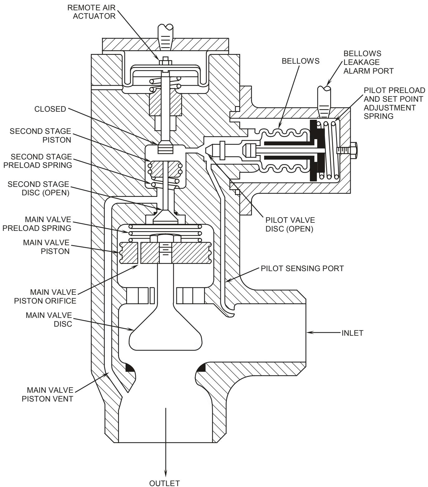
Figure 6.8-4 Three Stage Target Rock SRV (Safety Actuated)
