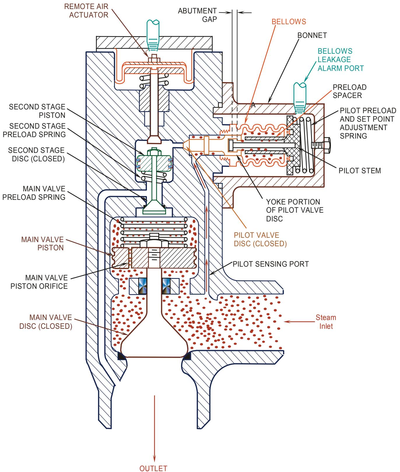
Figure 6.8-3 Three Stage Target Rock SRV (Closed)
