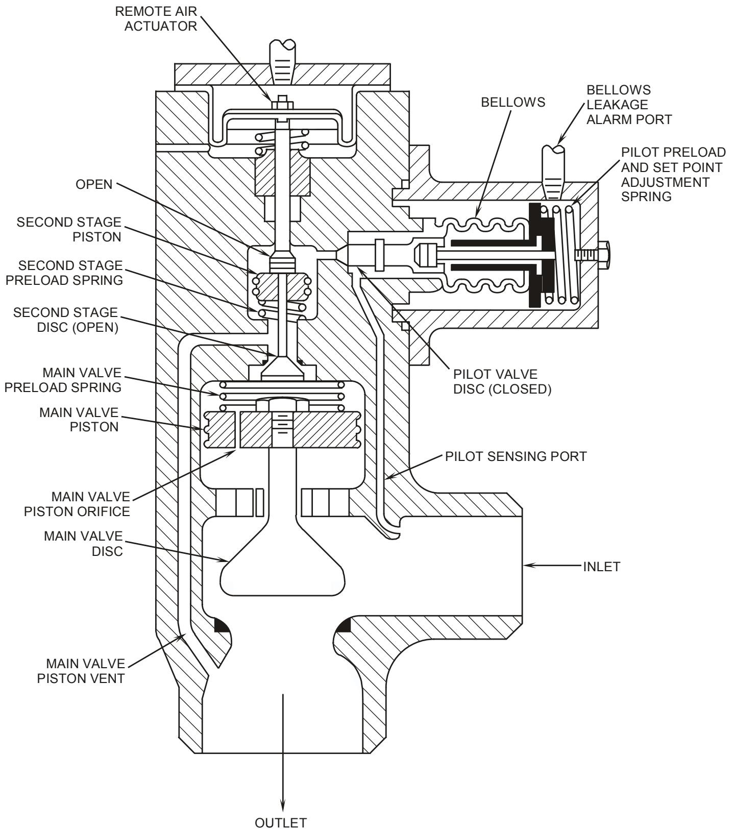
Figure 6.8-5 Three Stage Target Rock SRV (External Actuation)
