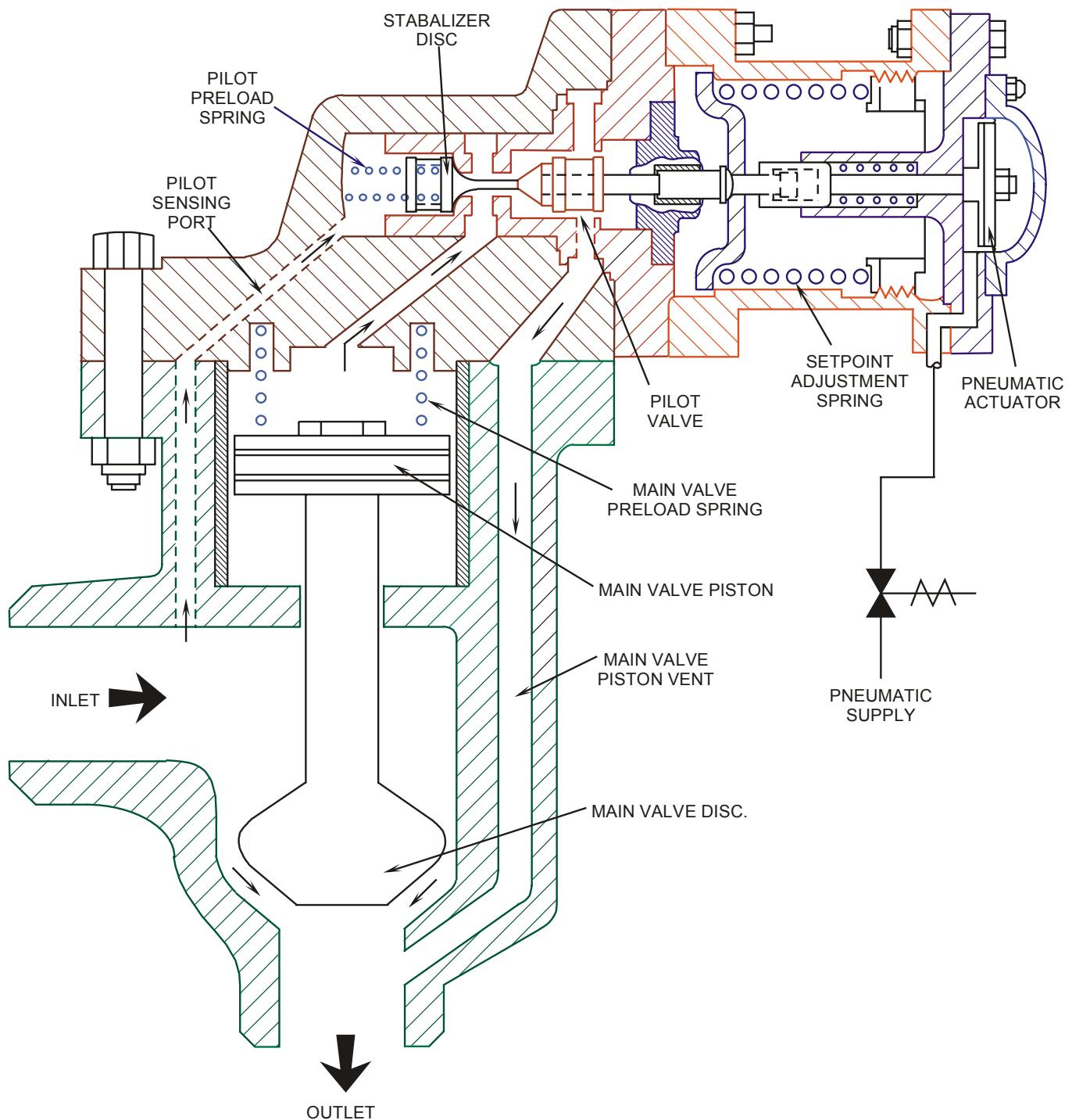
Figure 6.8-2 Two Stage Target Rock SRV (Open)
