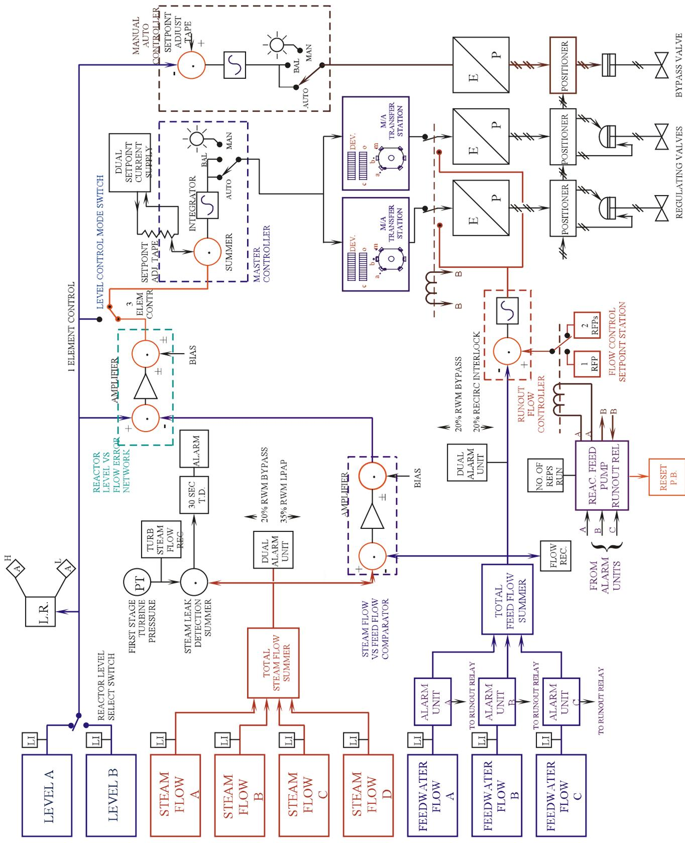
Figure 6.7-3 Feedwater Control System for Motor Driven Feed Pumps
