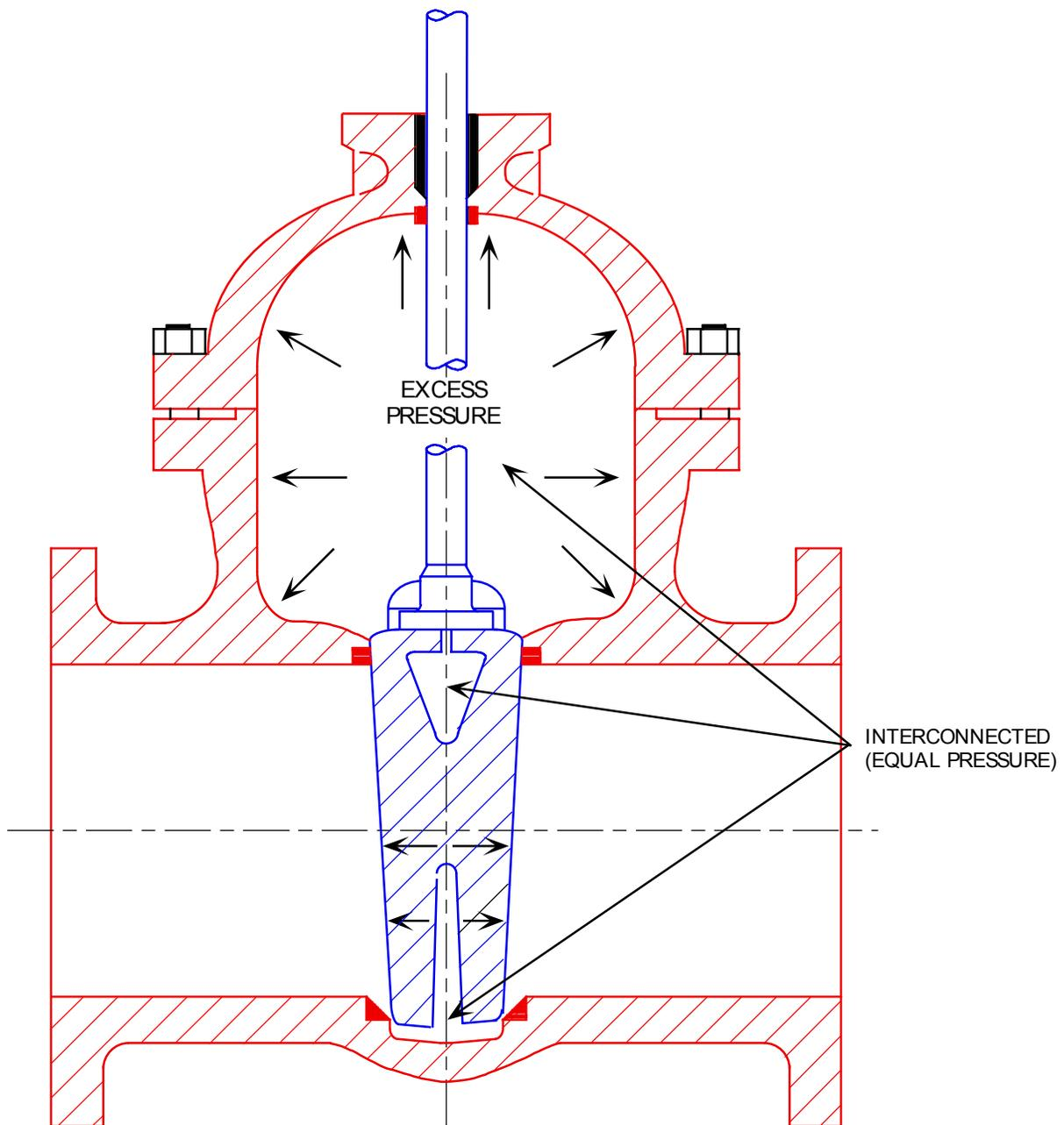
Figure 4.10-2 Pressure Locking Flexible-Wedge Gate Valve
